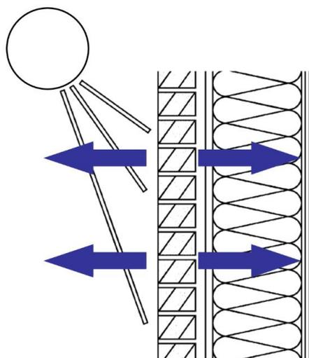
Figure 5. Solar vapor drive and interstitial condensation.
