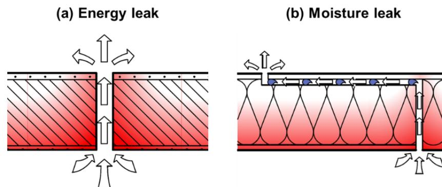
**Figure 3.** Types of indoor air leaks through joints or connections.
