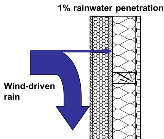
Figure 4. EIFS showing the deposit location of rainwater penetration through leaks.
