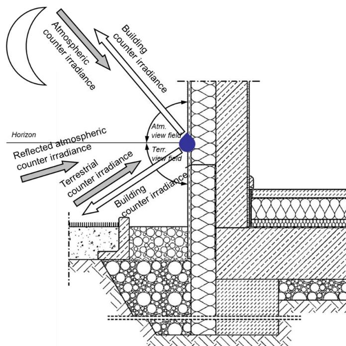
**Figure 6.** Long-wave radiation conditions on a vertical exterior surface.
