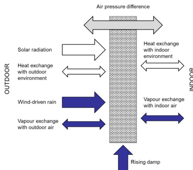
Figure 2. Hygrothermal loads and interchanging periodical directions on building envelope.
