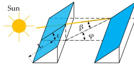
**Figure 2.** Schematic diagram of PV modules installed on a flat roof.
