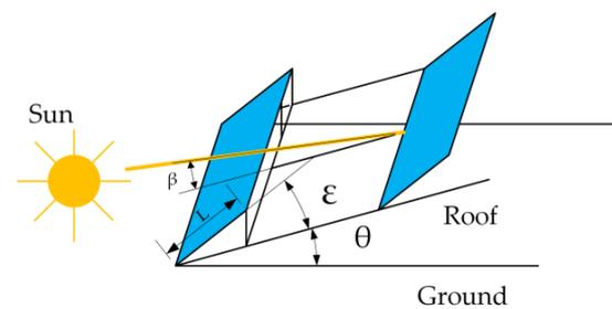
**Figure 3.** Schematic diagram of PV modules installed on a pitched roof.
