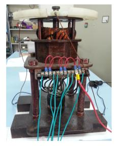
Figure 12. Split-winding bearing machine prototype.
