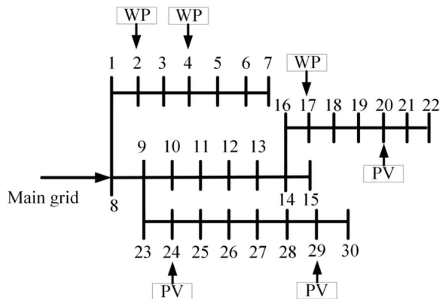
**Figure 1.** Improved IEEE 30 node distribution network system structure diagram.
