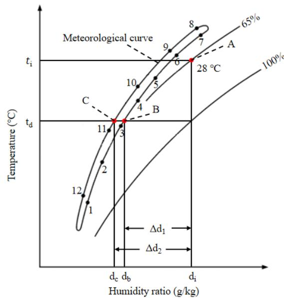
Figure 2. Principle diagram of ventilation-curve method.
