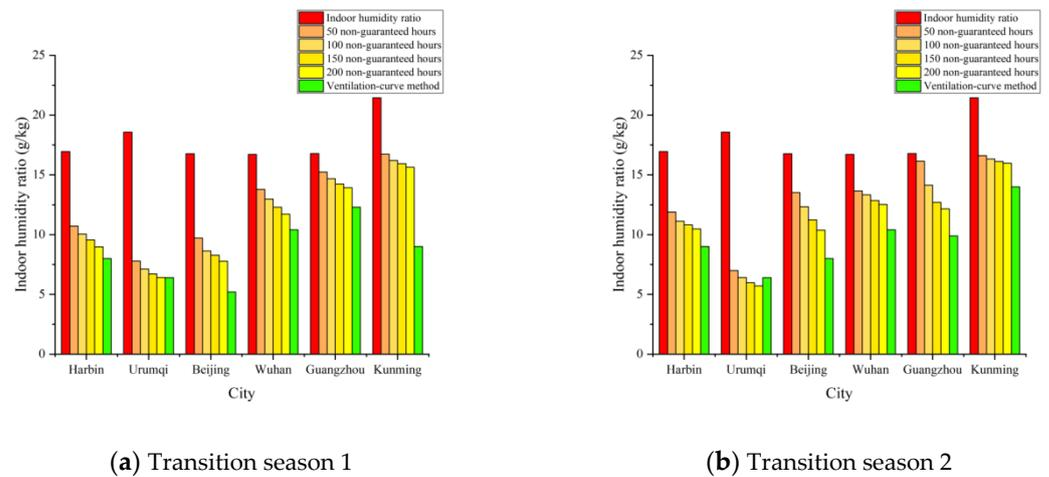
**Figure 6.** Calculation of indoor and outdoor humidity ratios.
