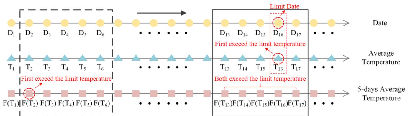
**Figure 4.** Principle diagram of 5-day moving average method.
