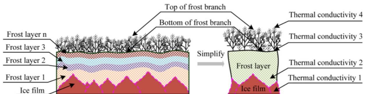
Figure 12. Morphology of frost formation on not properly clean heat exchanger surface [47].
