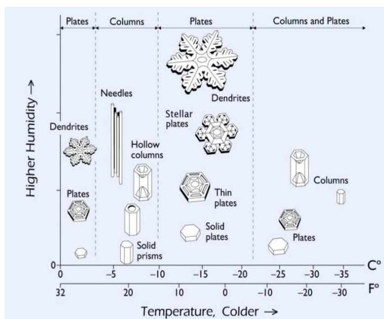
**Figure 10.** Frost flakes pattern depending on different temperature and humidity ranges. Reproduced with permission from [42], Elsevier, 2022.
