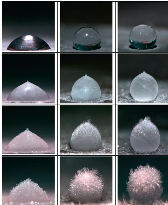
**Figure 13.** Water droplet freezing with farther crystal growth. Reproduced with permission from [43], Elsevier, 2022.
