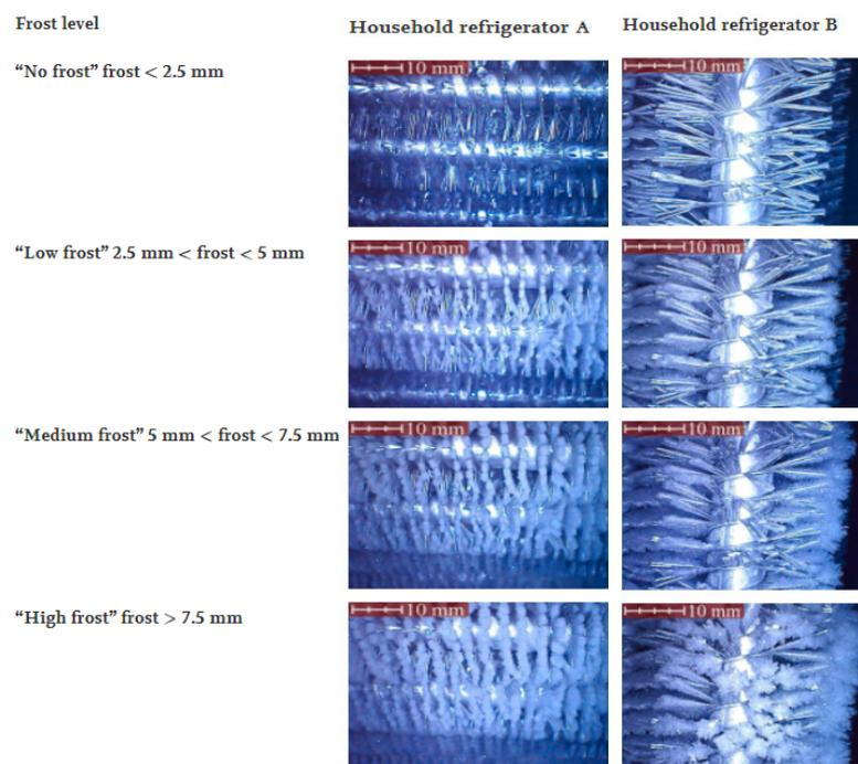
**Figure 15.** Frost layer growth on the evaporator of the domestic refrigerator. Visualization and thickness measurements. Reproduced with permission from [48], Elsevier, 2022.
