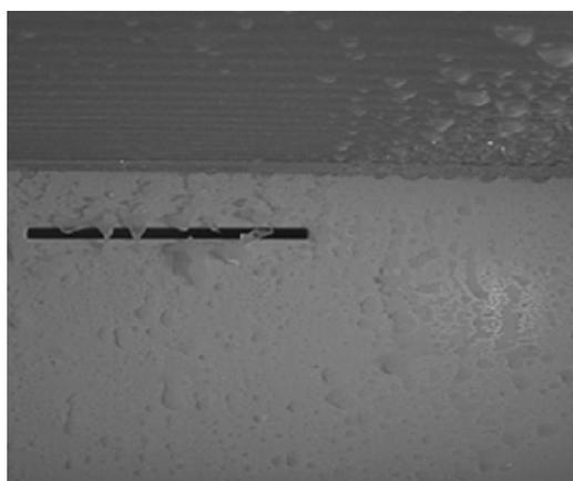
**Figure 9.** Frost formation on the surface of liner. Reproduced with permission from [37], Elsevier, 2011.
