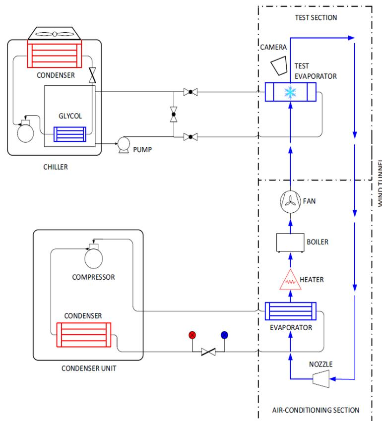
Figure 16. Schematic of the test setup. Where the blue color represents refrigerant (glycol) cycle and red—the air. Reproduced with permission from [64], Elsevier, 2021.
