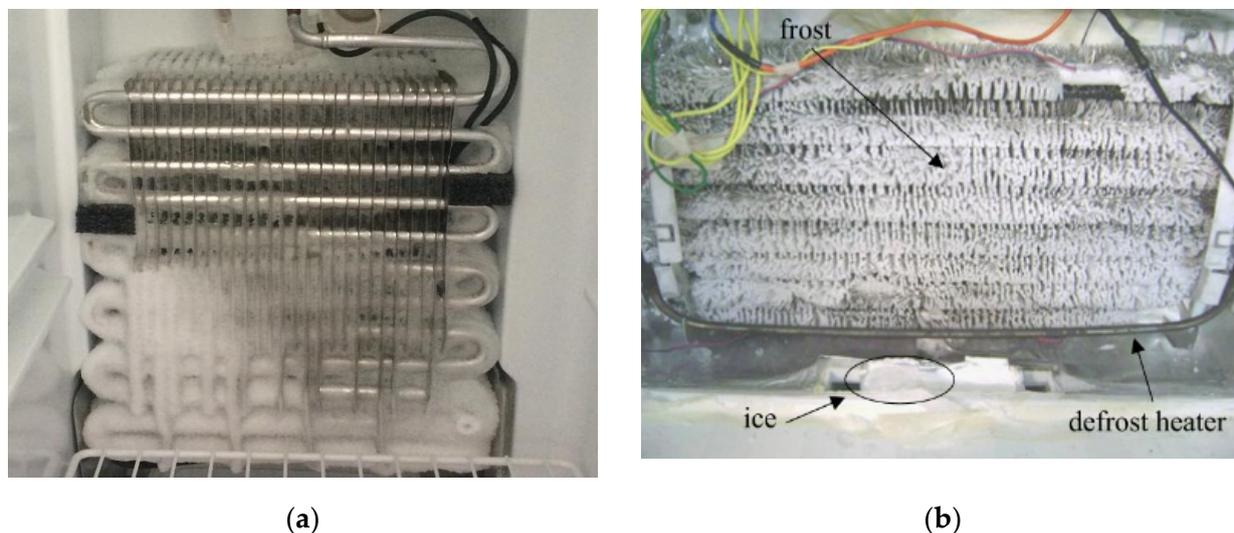
**Figure 8.** Clogged evaporator: (a) Vertical FoT (fin on tube) evaporator [35]; (b) Horizontal FoT evaporator. Reproduced with permission from [36], Elsevier, 2015.
