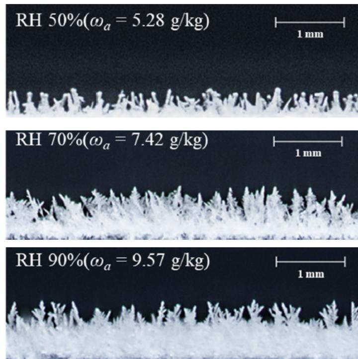
**Figure 11.** Frost pattern for different humidity ranges. Reproduced with permission from [42], Elsevier, 2022 [42].
