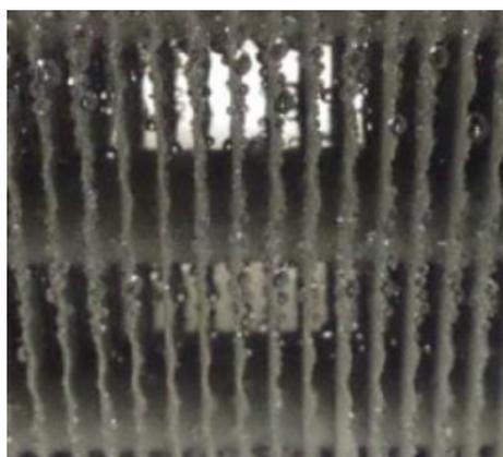
**Figure 7.** Frost formation on the ACM machine. Reproduced with permission from [16], Elsevier, 2022.
