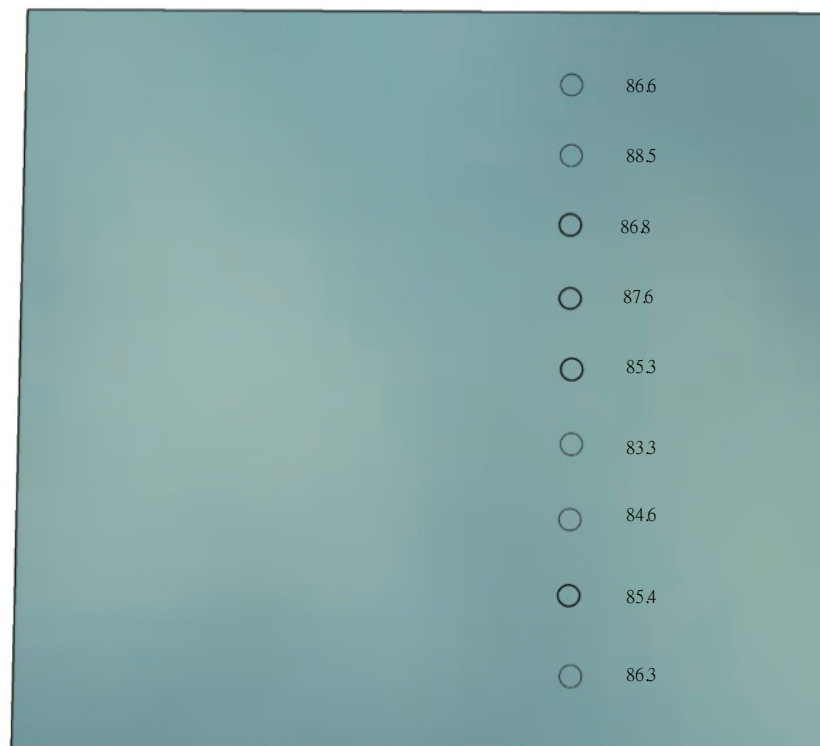
Figure 12. Automated measurement result of light transmittance after 3.5 days of dust deposition.
