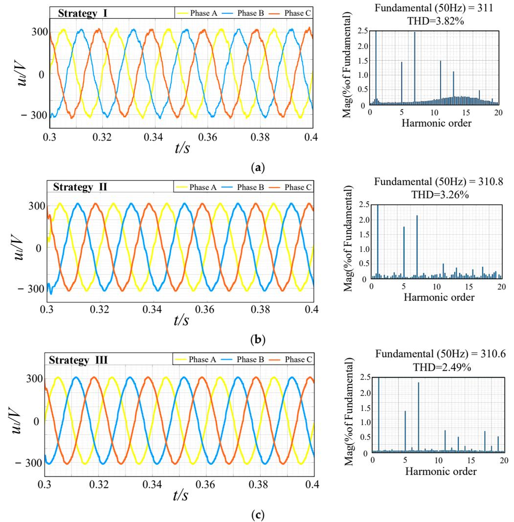
**Figure 12.** Load voltage after compensation under harmonic conditions. (a) Load voltage under Strategy I; (b) load voltage under Strategy II; (c) load voltage under Strategy III.
