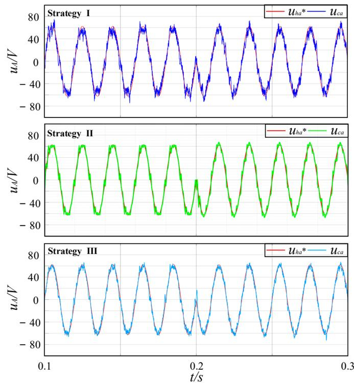
Figure 9. Comparison of A-phase output voltage tracking effect.
