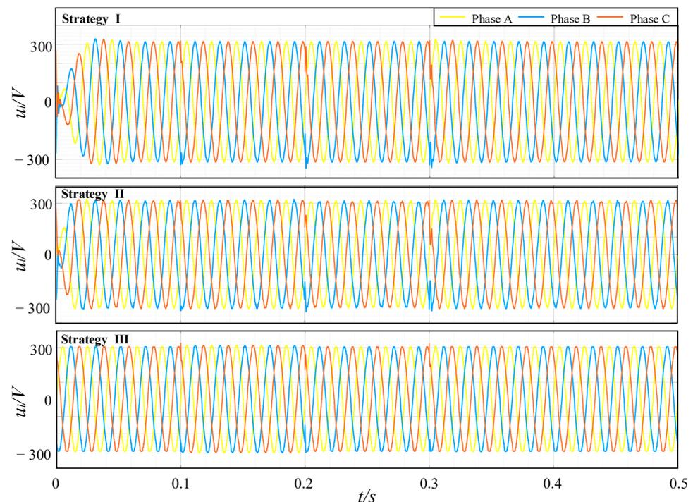
**Figure 7.** Load voltage under temporary swell, sag, and sudden load change conditions.
