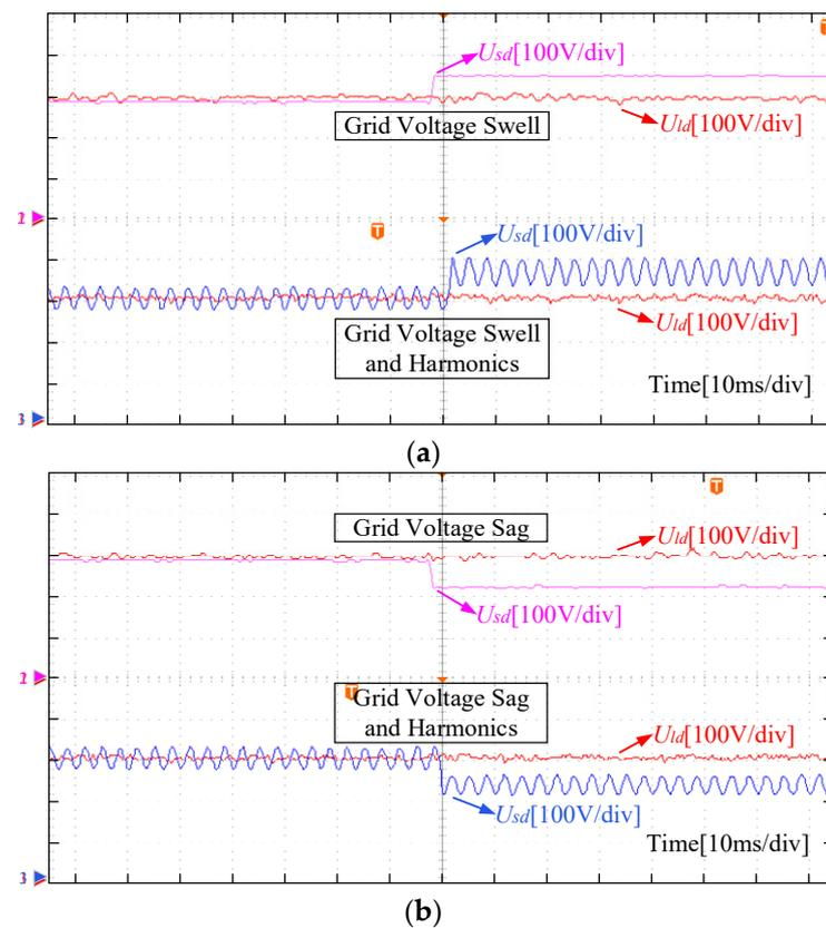
**Figure 18.** d-axis voltage at change in working conditions. (a) Grid voltage swell and harmonics. (b) Grid voltage sag and harmonics.
