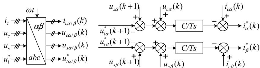
Figure 3. Reference current generation mechanism based on DBDC.
