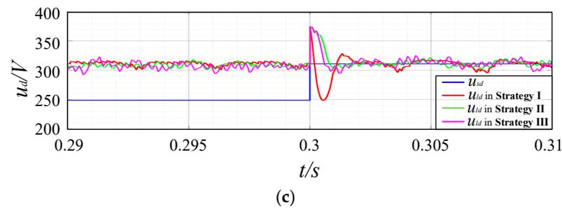
**Figure 11.** Voltage details at change in working conditions. (a) Instantaneous grid voltage swell; (b) instantaneous grid voltage sag; (c) instantaneous sudden changes in load.
