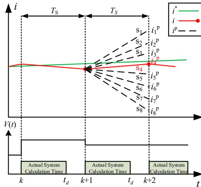
Figure 4. Predictive current control diagram after delay compensation.
