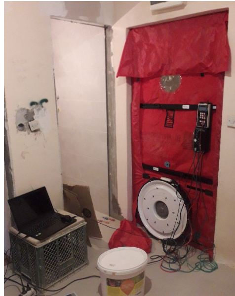
Figure 2. Airtightness measurement using blower door fan.
