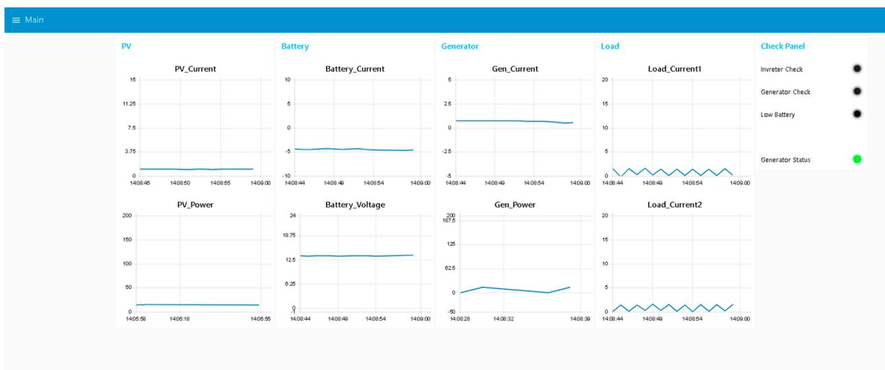
Figure 13. Node-Red dashboard for visualization.
