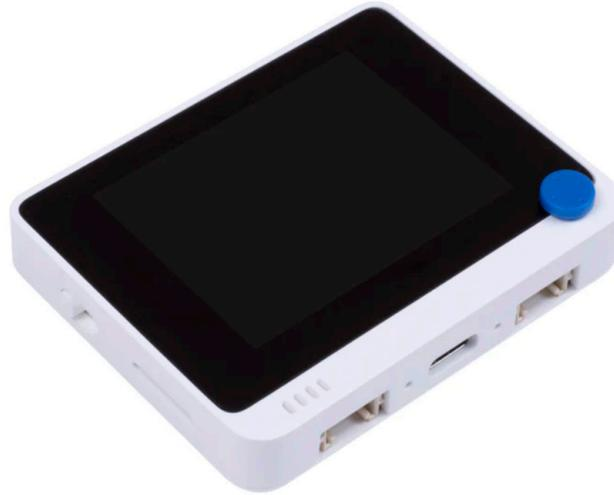
Figure 5. Wio terminal as the second RTU.
