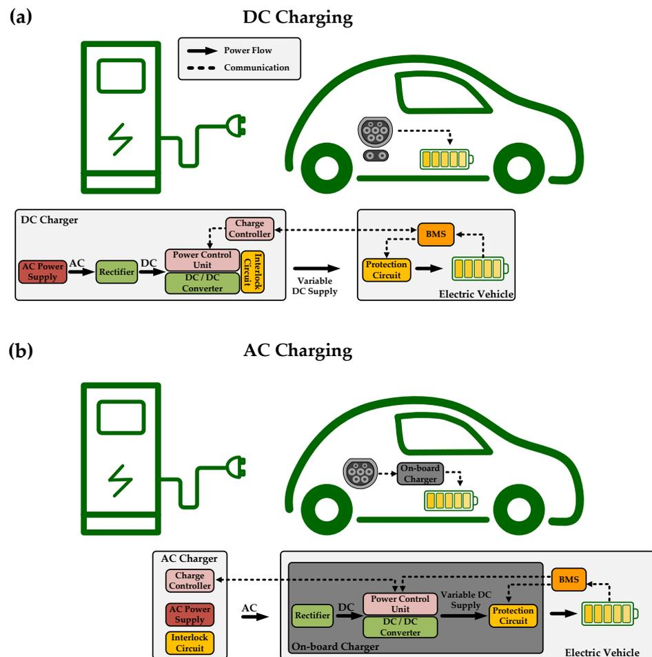
Figure 1. General schemes for (a) DC charging and (b) AC charging [25–27].
