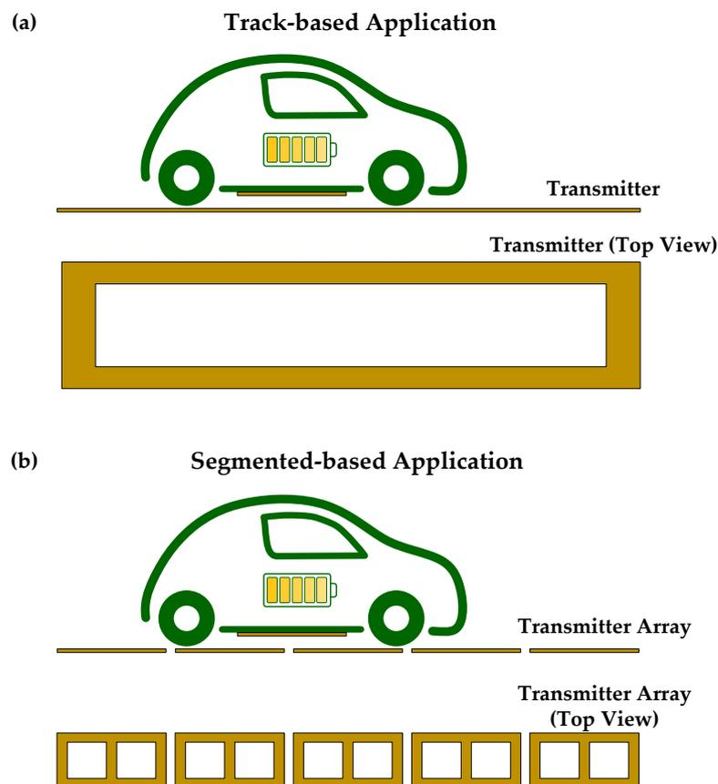
**Figure 7.** Transmitter coil configuration: (a) track-based; (b) segmented-based.
