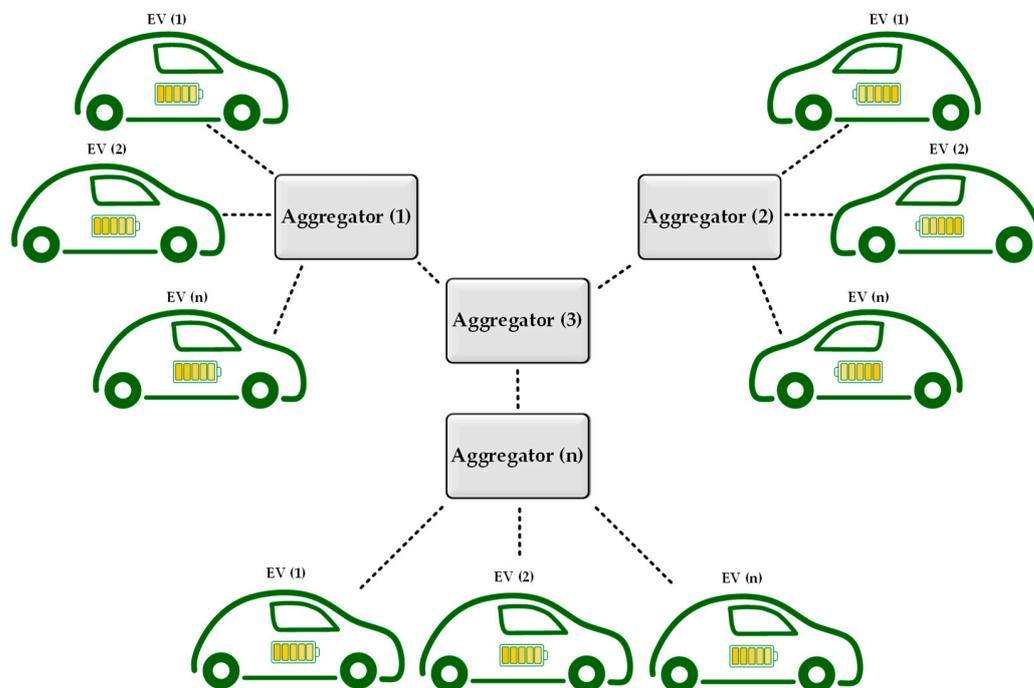
Figure 10. Hierarchical control architecture of EV charging [13,69].
