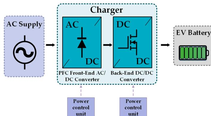
**Figure 2.** Block diagram of a conductive unidirectional EV charging system.
