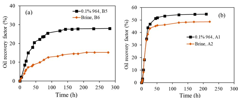
**Figure 7.** Oil recovery of Middle Bakken and Berea core samples with different pore sizes. (a) B5, B6 from well #1. (b) A1 and A2.
