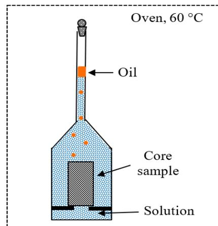
**Figure 3.** Image of spontaneous imbibition experiments setup. Experiments were conducted in an oven at 60 °C.
