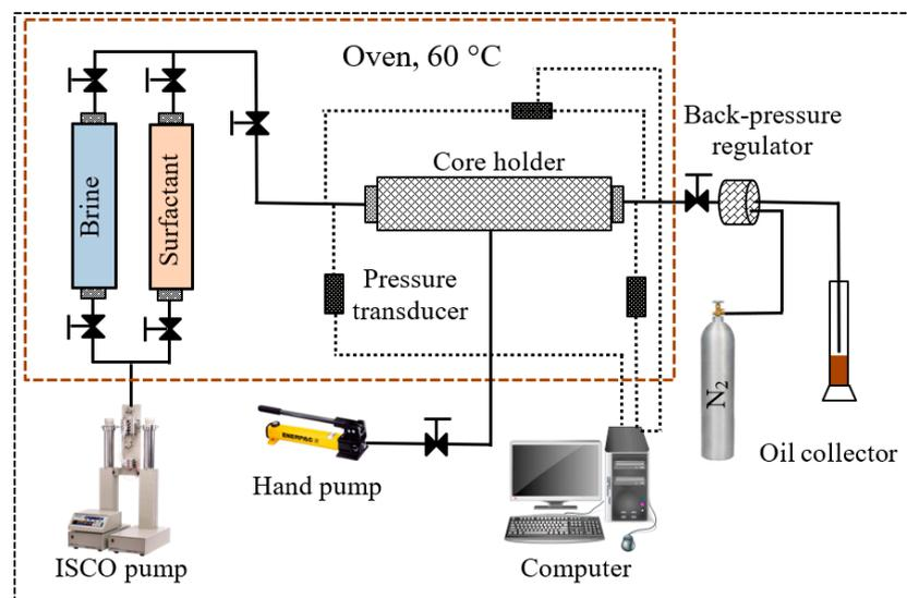
**Figure 4.** Schematic of core-flooding setup.
