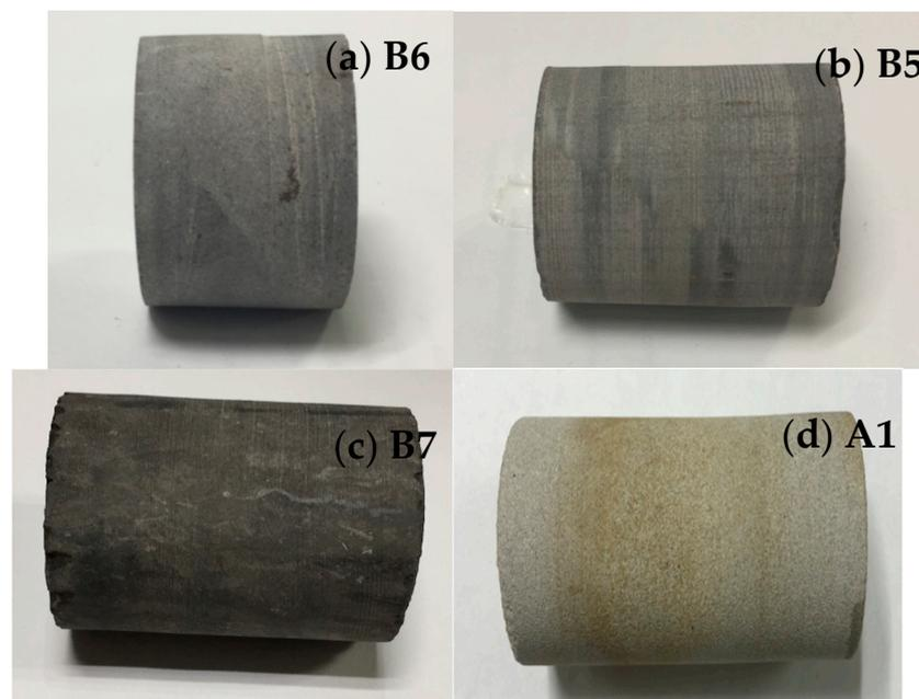
**Figure 1.** Pictures of studied Bakken and Berea core samples.
