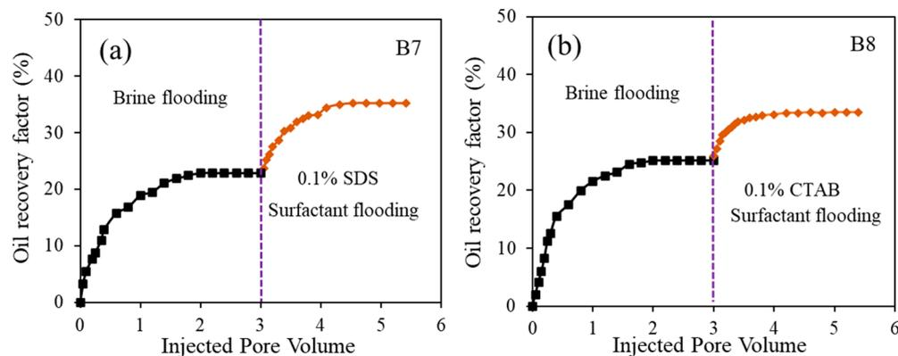
**Figure 8.** Enhanced oil recovery in two Bakken tight rocks samples by brine and surfactant flooding. (a) Flooding with 0.1% SDS. (b) Flooding with 0.1% CTAB.
