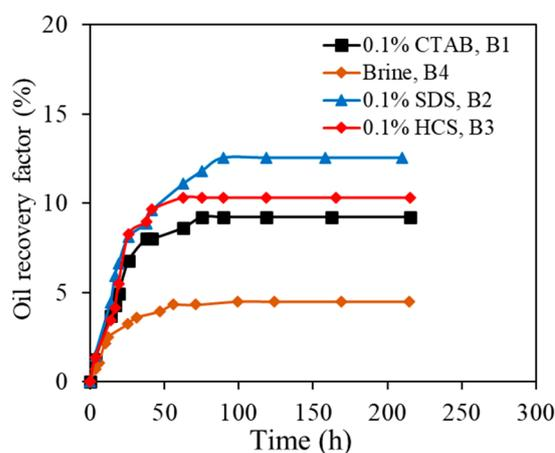
**Figure 6.** Oil recoveries of B1–B4 (well #1) through spontaneous imbibition experiments with and without various surfactants added.
