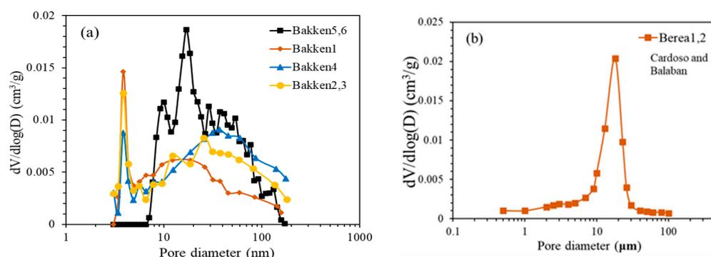
**Figure 5.** Pore size distribution of Bakken and Berea samples. (a) Bakken samples. (b) Berea samples from mercury intrusion by Cardoso and Balaban [36].
