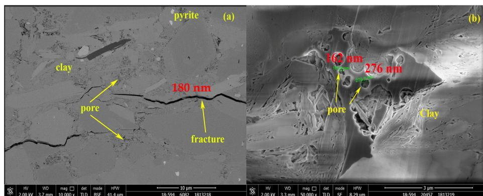
**Figure 2.** SEM images of the Middle Bakken samples. (a) B5 and B6. (b) B7 and B8.
