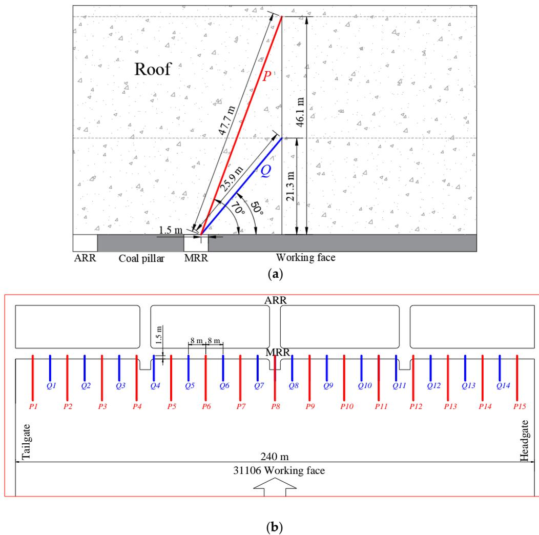
**Figure 16.** Roof fracturing scheme of retracement roadway: (a) fracturing borehole profile inside the main retracement roadway; (b) borehole layout.
