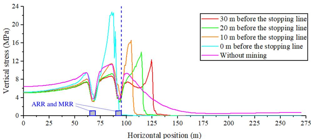
**Figure 9.** Distribution of immediate roof stress during the final mining period of working face 31,106.
