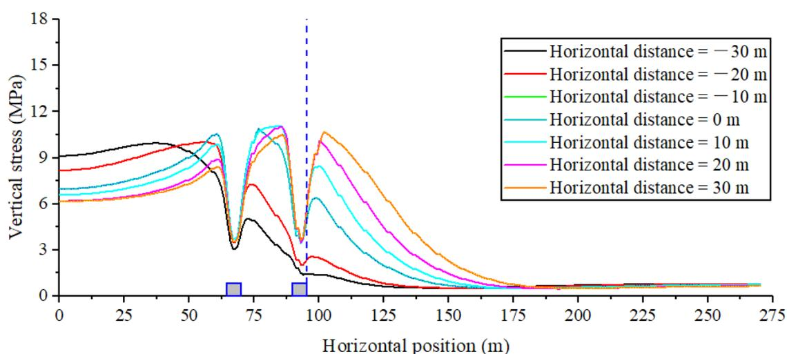
**Figure 6.** Distribution of immediate roof stress at different horizontal distances.
