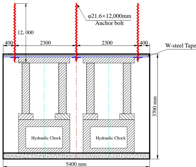
**Figure 14.** Schematic diagram of roof reinforcement and support of main retracement roadway.
