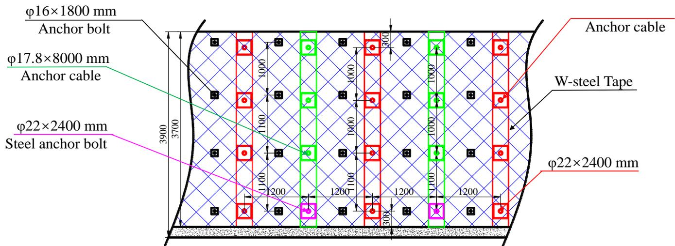
**Figure 15.** Secondary reinforcement and support of auxiliary wall of main retracement roadway.
