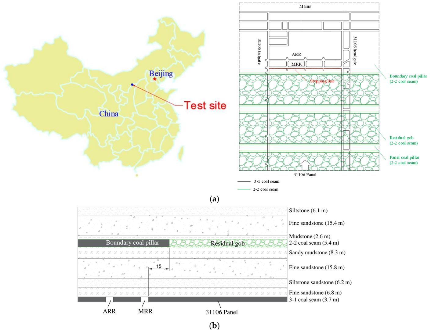
**Figure 1.** Overview of working face 31,106: (a) The layout of the 31,106 panel and 2–2 residual coal seam; (b) section of the relative position of the retracement roadway and the residual pillar of working face 31,106.
