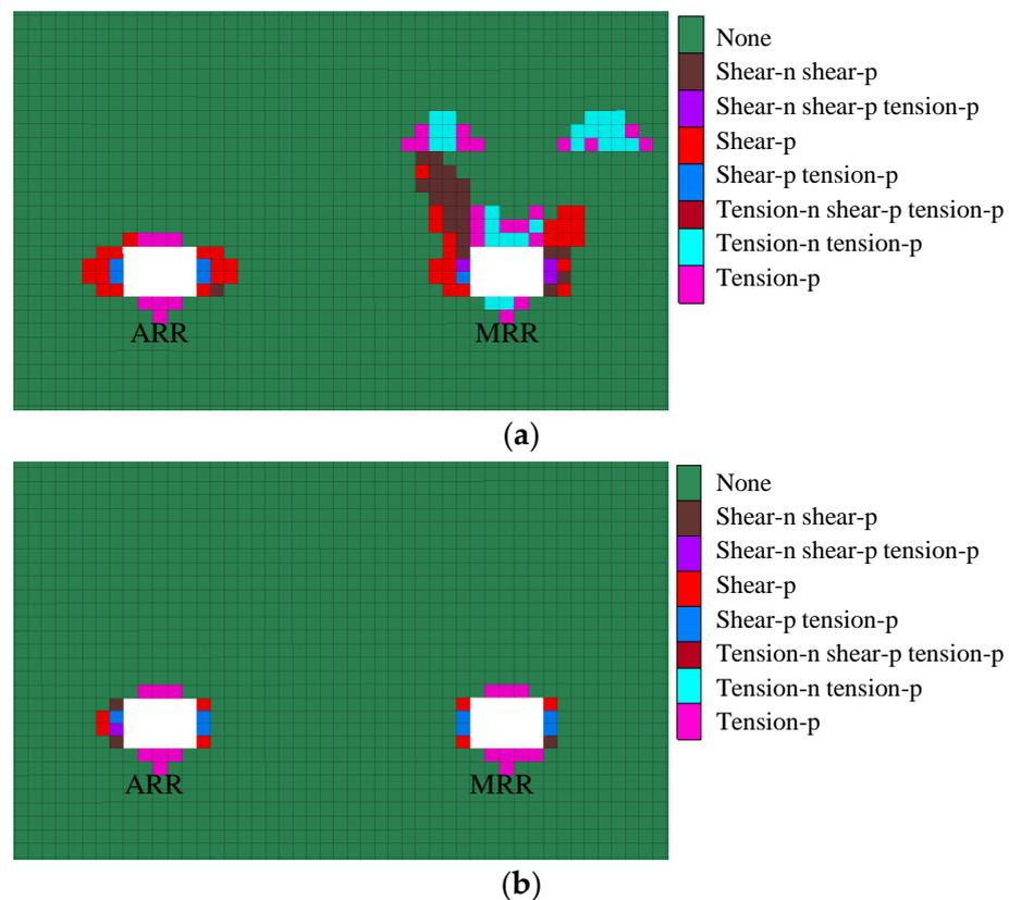
**Figure 8.** Distribution of plastic zone of surrounding rock of retracement roadway: (a) horizontal distance = 15 m; (b) horizontal distance = −30 m.
