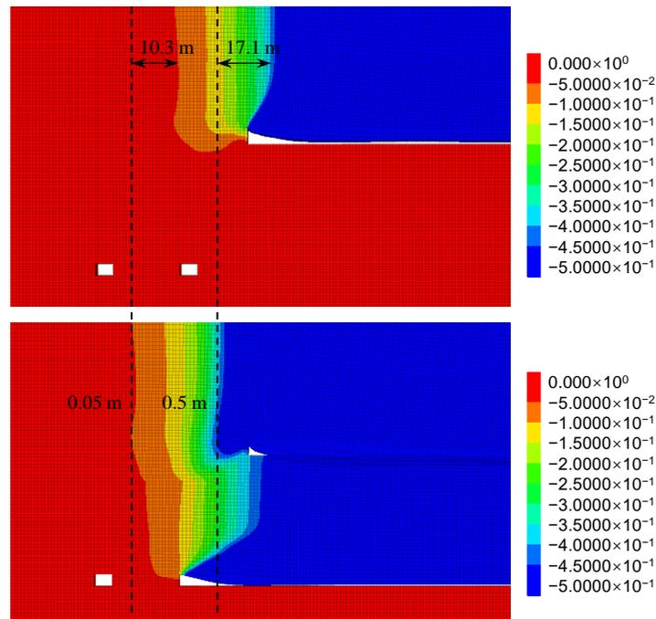
Figure 11. Distribution of roof displacement in different mining stages.
