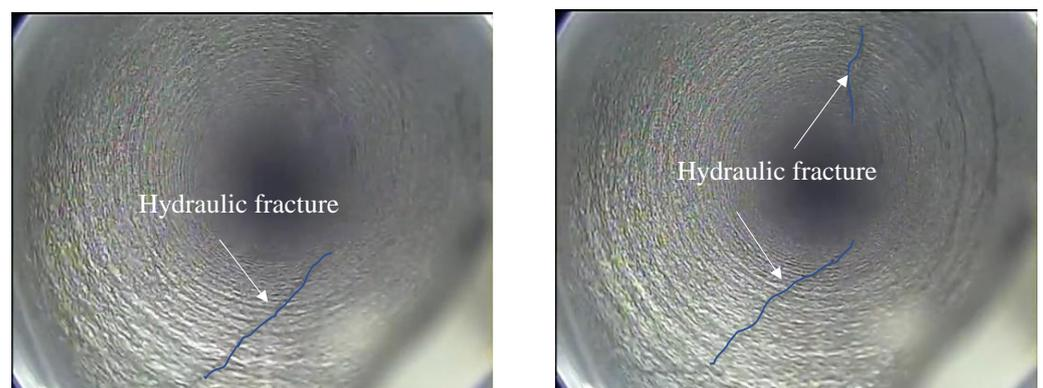
**Figure 17.** Fracture distribution characteristics of hydraulic fracturing boreholes.
