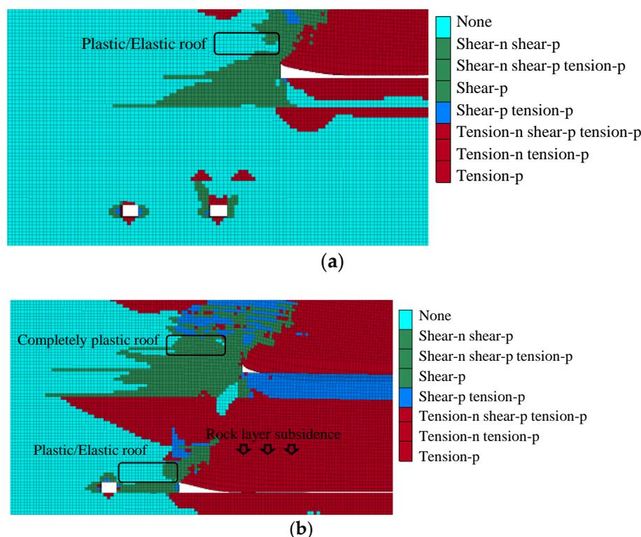
**Figure 10.** Distribution of plastic zones in different mining stages: (a) after mining of the 2–2 coal seam; (b) after the working face 31,106 is connected with the retracement roadway.
