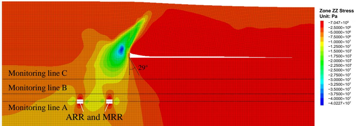
**Figure 4.** Cloud chart of surrounding rock stress under the action of residual pillar in working face 31,106.
