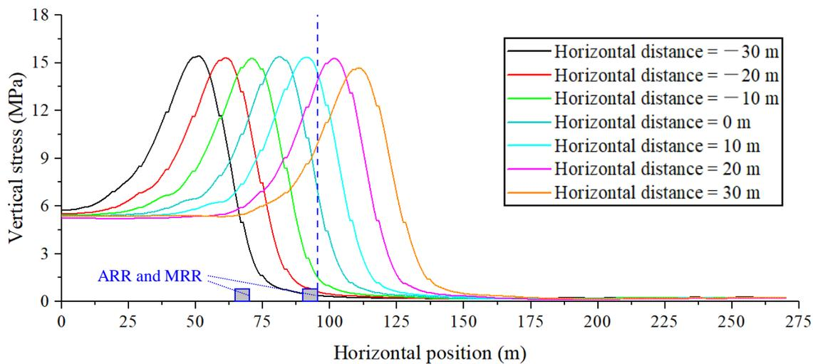
**Figure 7.** Distribution of main roof stress at different horizontal distances.
