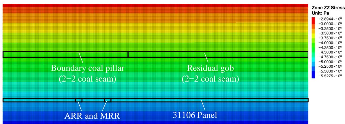
**Figure 3.** Schematic diagram of numerical model for mining under residual pillar (vertical stress cloud chart).
