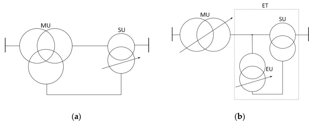
**Figure 5.** Examples of schematic diagrams of a regulating transformer: (a) power supply of the series transformer from the third winding of the main unit; (b) powering the series transformer from the exciting transformer.
