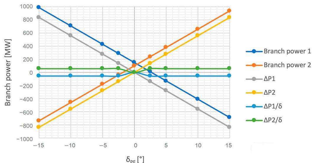
Figure 14. Graph of the dependence of the branch power as a function of the phase shifter adjustment angle.
