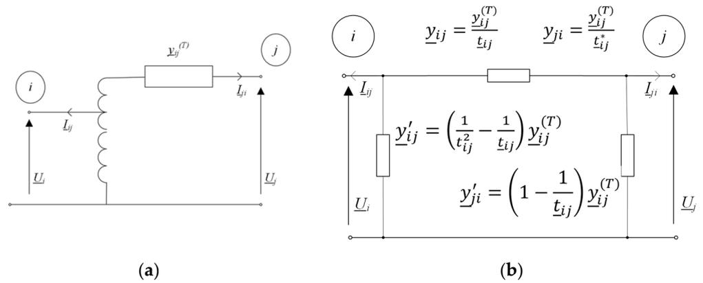
**Figure 12.** Replacement scheme: (a) with an autotransformer, (b) II-type four-pole equivalent.
