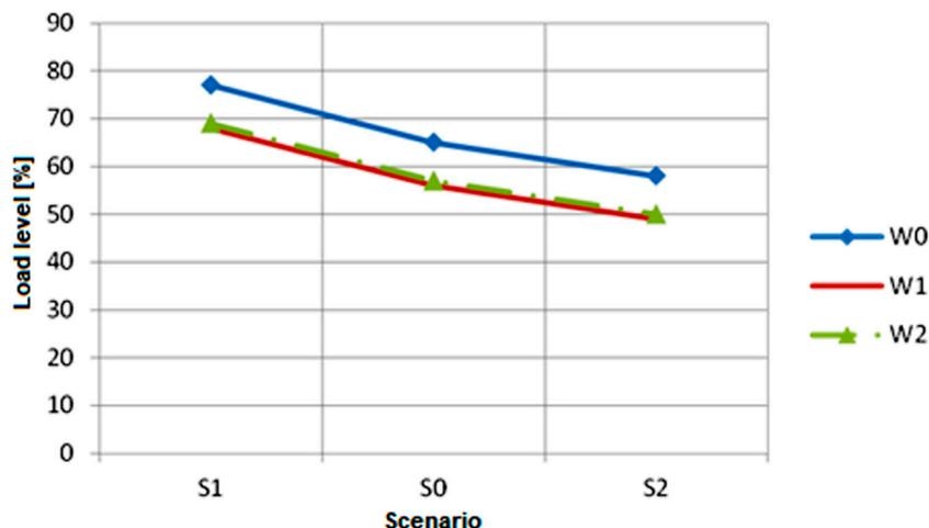
**Figure 11.** Changes in the load level on the 220 kV line on the Joachimów–Rogowiec relation for various variants of the PPS operation and scenarios for the transformer control settings.
