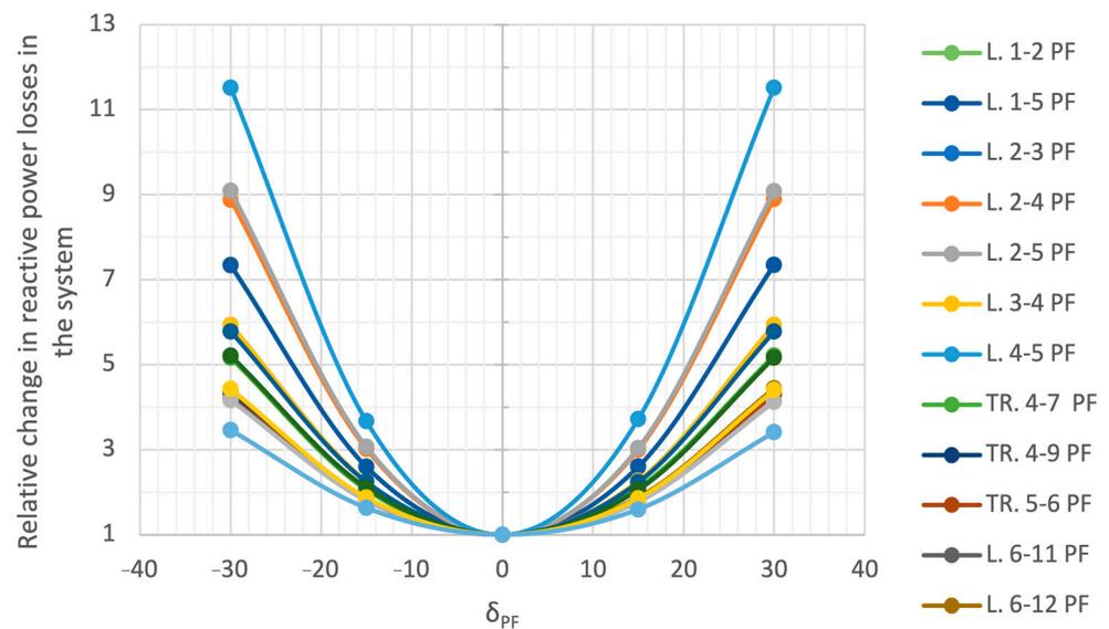
**Figure 20.** Relative changes in the reactive power of the 14 W system as a function of the regulation angle PF.
