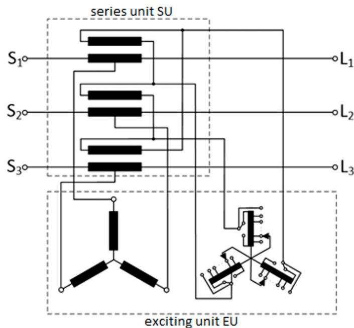
**Figure 6.** Schematic diagram of a regulating transformer exciting unit, where S1–S3 means three-phase source terminals and L1–L3 respectively means load terminals.
