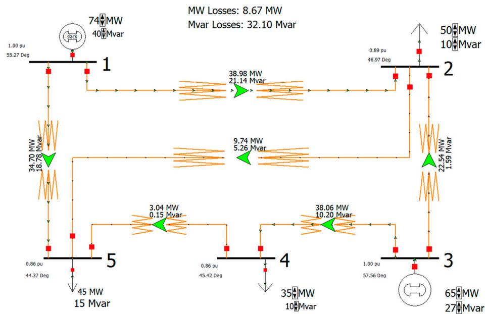
Figure 15. IEEE 5-node test system.
