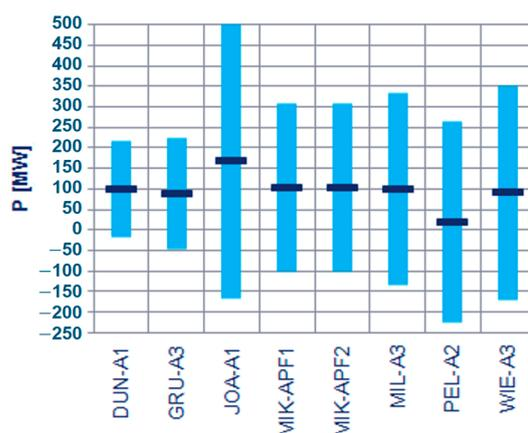
**Figure 2.** Maximum changes in the power flow of regulating transformers in the Polish NPS.
