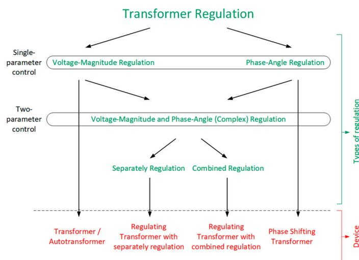
**Figure 4.** Types of regulation and transformer devices implementing them [48].
