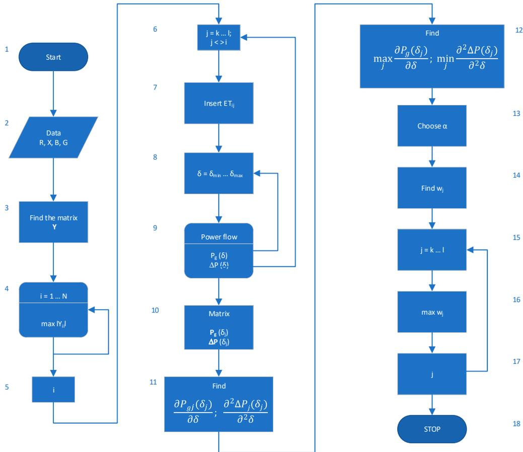
Figure 21. Algorithm for determining the optimal location of the regulating transformer.
