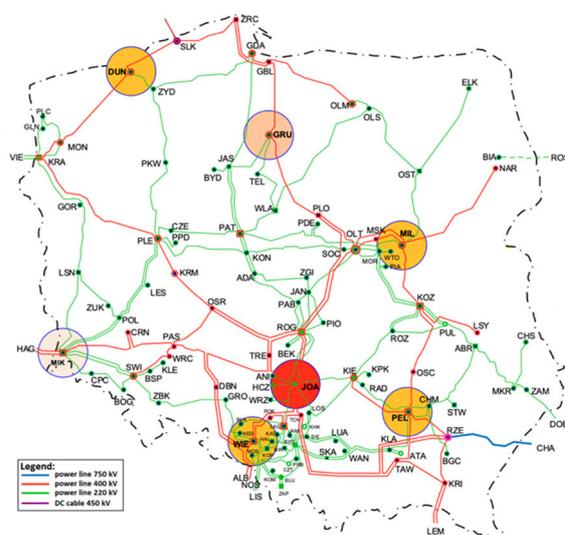
**Figure 1.** Locations of control transformers in the Polish power system.
