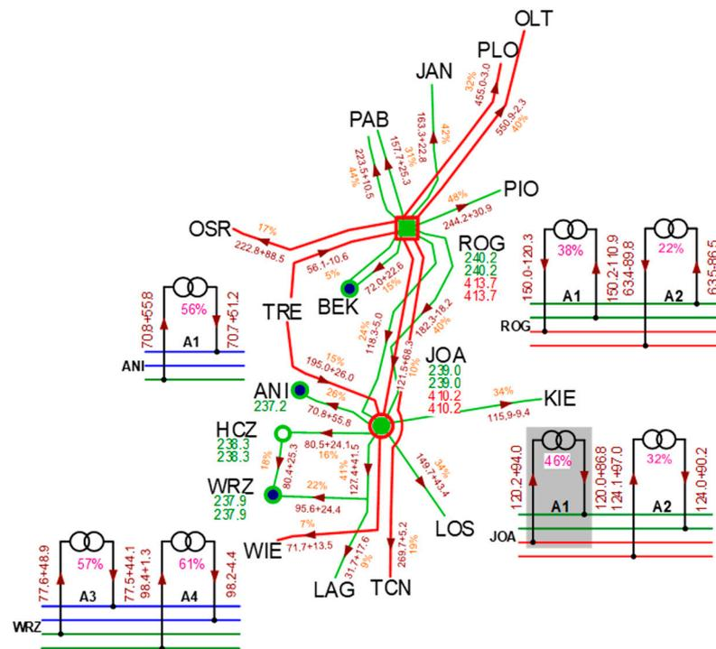
Figure 8. Power flows in the substation with the JOA-A1 transformer and in its network vicinity.
