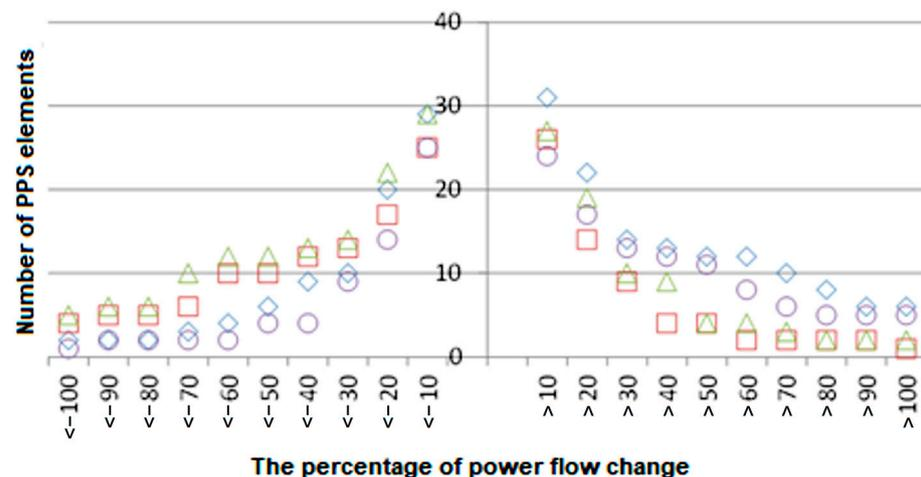
**Figure 10.** Dependence of the number of PPS elements on the direction and range of power flow change for various control scenarios of the JOA-A1 transformer.
