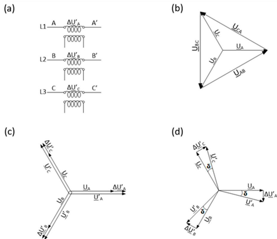
**Figure 7.** The idea of regulating transformer regulation: (a) series transformer winding; (b) phase voltages and phase-to-phase voltages supplying the series unit; (c,d) phase voltages at the output of the series unit (Figure (c)—for voltage-magnitude regulation; Figure (d)—for phase-angle regulation).
