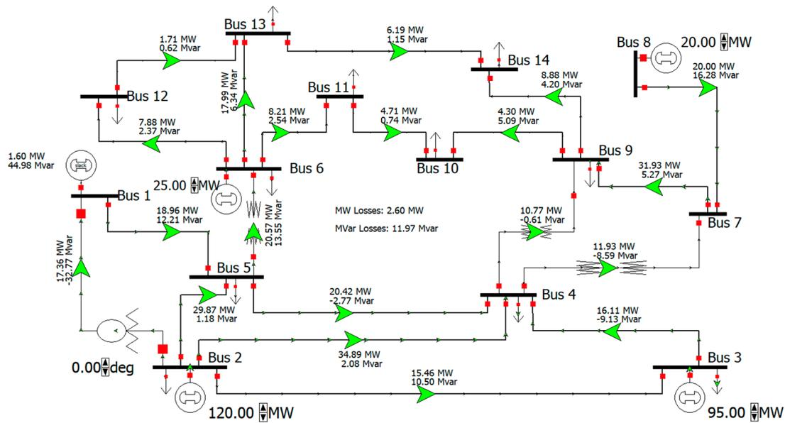
Figure 18. Test 14-node IEEE system.
