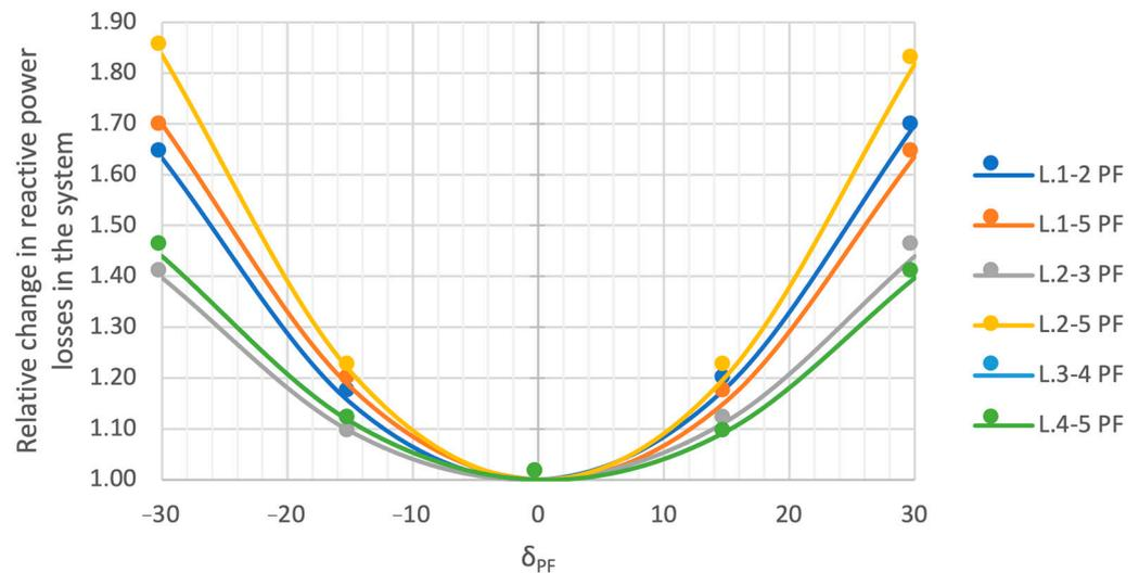
**Figure 17.** Relative reactive power losses as a function of the control angle PF.
