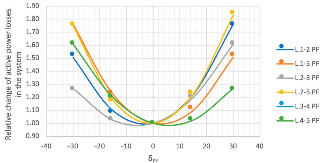
**Figure 16.** Relative active power losses as a function of the control angle PF.
