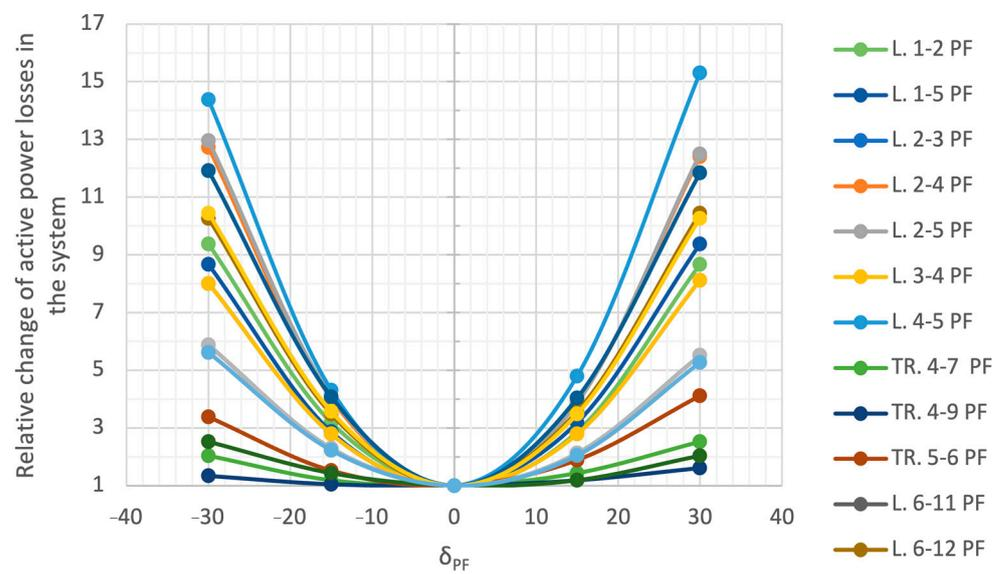
**Figure 19.** Relative changes in the active power of the 14 W system as a function of the regulation angle PF.
