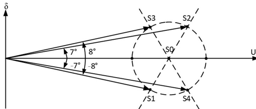
Figure 9. Scenarios for setting the regulation parameters of a regulating transformer.
