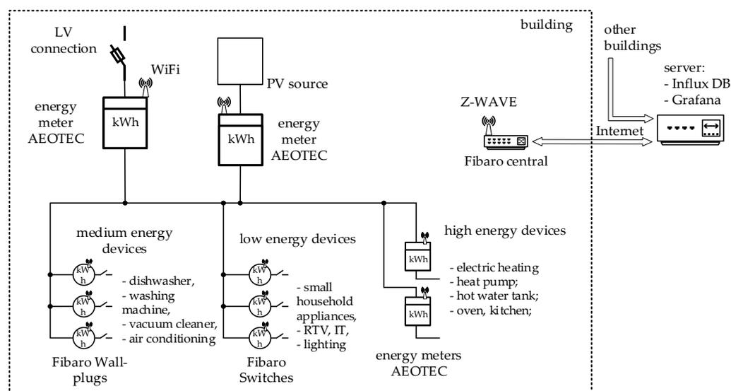
**Figure 3.** Scheme of the Fibaro measurement system in the building. Source: author's development.
