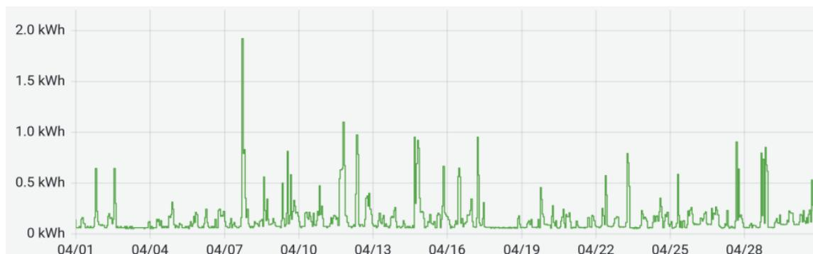
**Figure 5.** An example graph from the Grafana application of 60 min energy from 1–30 April 2022, for a flat used by 2 persons. Source: author’s development.
