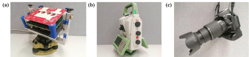
Figure 3. Instruments: (a) MIMO-SAR system, (b) total station, and (c) video camera.
