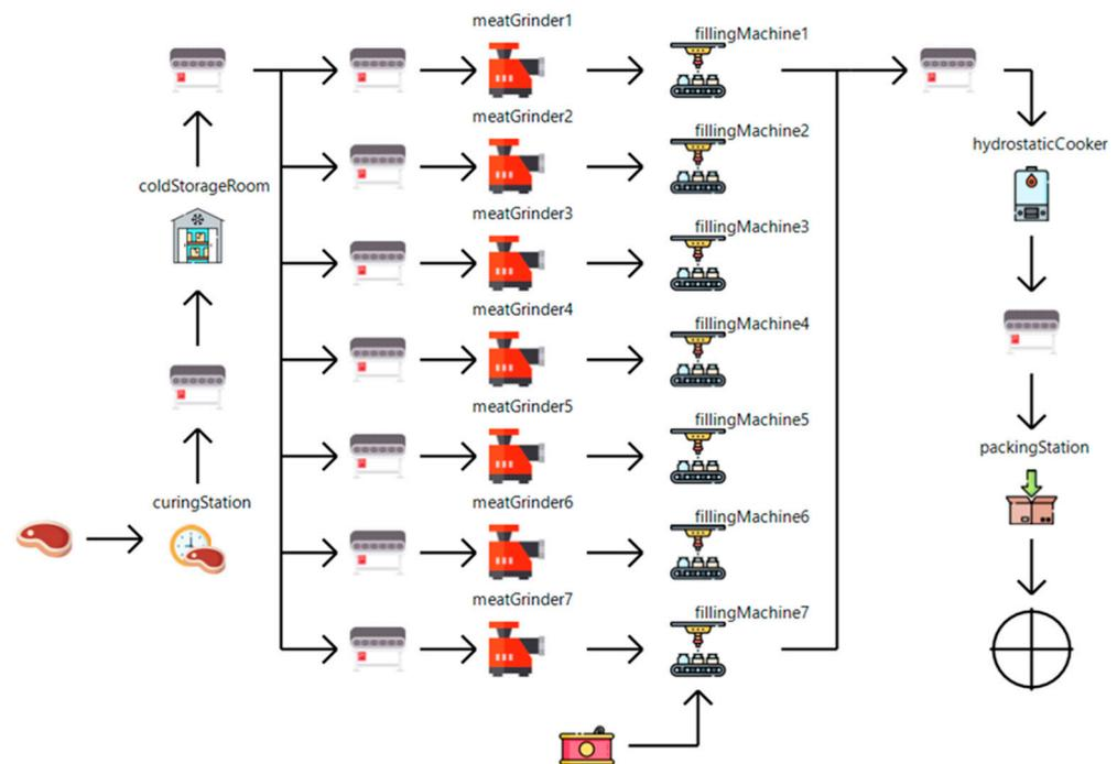
Figure 9. Developed process-flow for the canned-meat production process.
