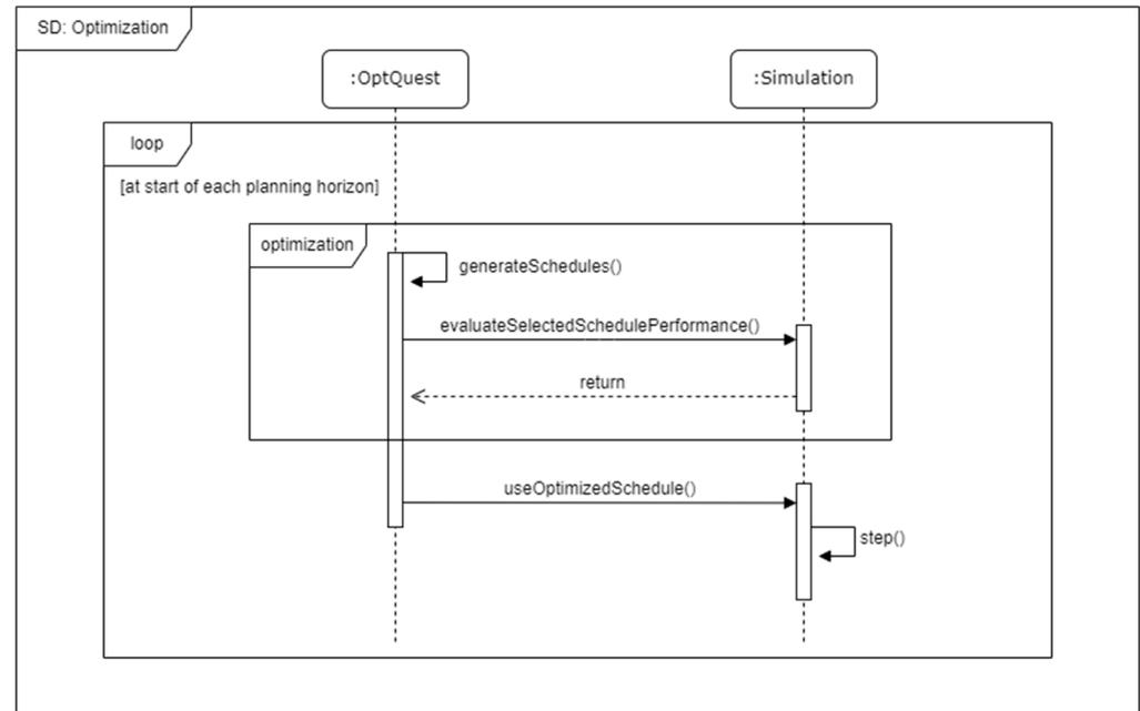
**Figure 6.** Sequence diagram showing the multi-objective optimization-simulation interaction.
