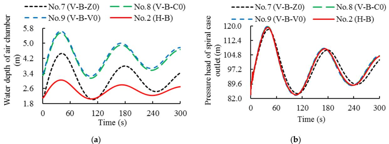
**Figure 4.** Comparison of horizontal and vertical ACSCs under load rejection condition B: (a) Water depth varying with time; (b) Pressure at the end of spiral case varying with time.
