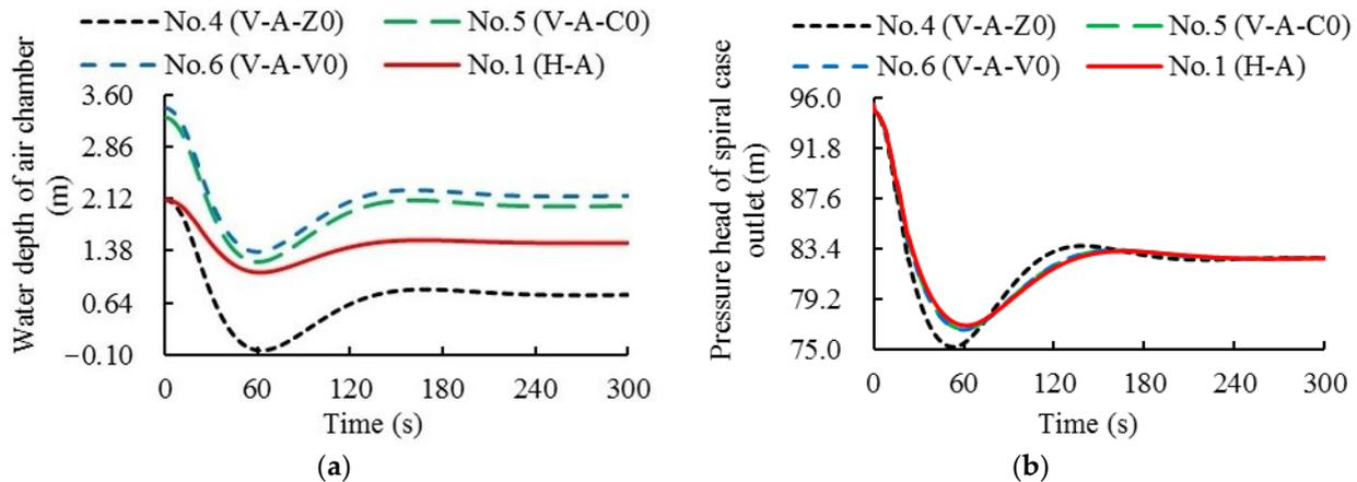
**Figure 3.** Comparison of horizontal and vertical ACSCs under load acceptance condition A: (a) Water depth varying with time; (b) Pressure at the end of spiral case varying with time.
