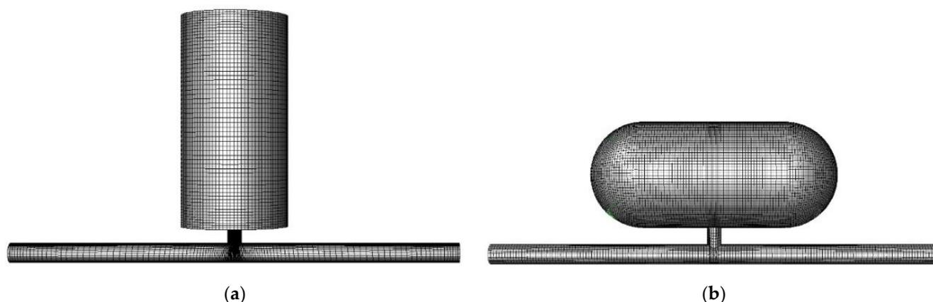
**Figure 2.** Computational domain of two models of 3D simulation. (a) Vertical ACSC; (b) Horizontal ACSC.
