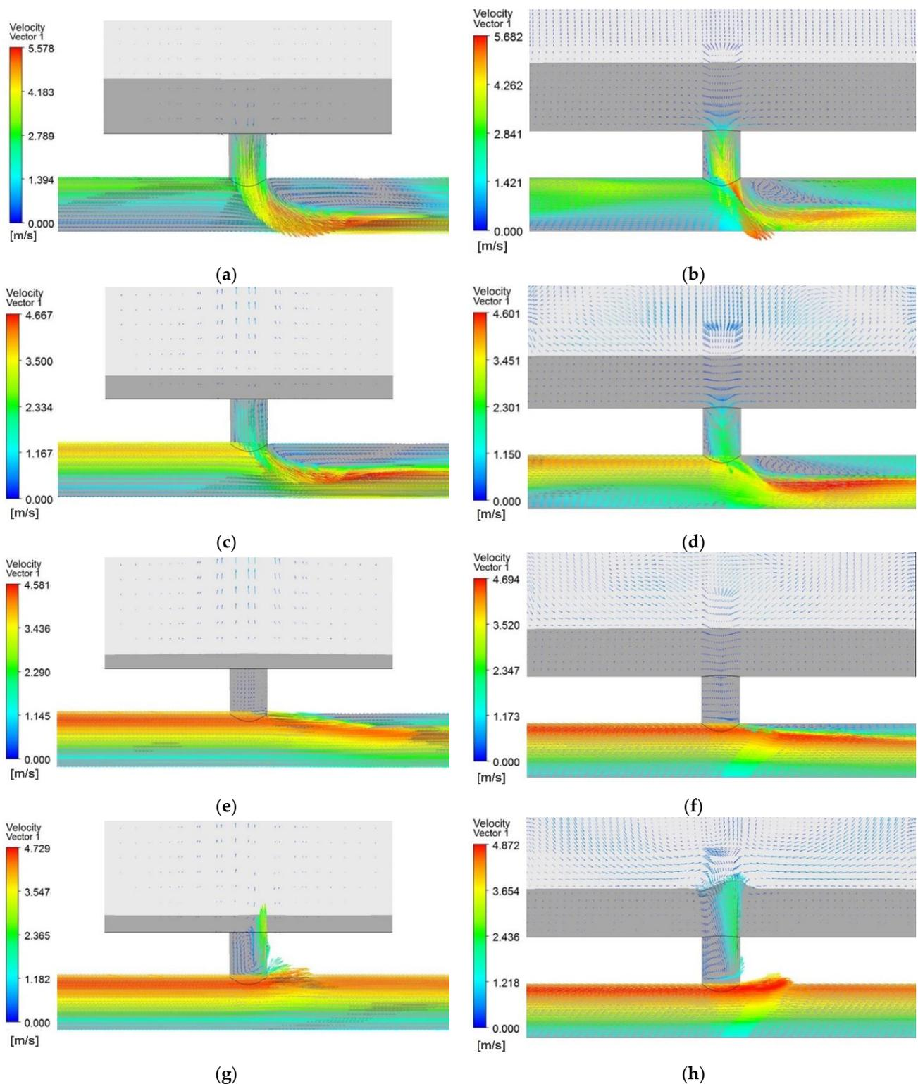
**Figure 7.** Comparison of horizontal and vertical ACSC flow regimes at different time points: (a) vertical ACSC at  $T = 23.5$  s; (b) horizontal ACSC at  $T = 23.5$  s; (c) vertical ACSC at  $T = 45$  s; (d) horizontal ACSC at  $T = 45$  s; (e) vertical ACSC at  $T = 67$  s; (f) horizontal ACSC at  $T = 67$  s; (g) vertical ACSC at  $T = 80$  s; (h) horizontal ACSC at  $T = 80$  s.
