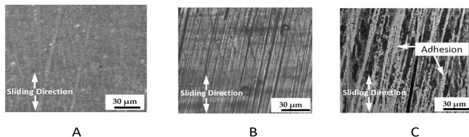
**Figure 1.** Cr electroplated piston ring friction wear scars under different static loads. (A) Load 50 [N]; (B) Load 290 [N]; (C) Load 400 [N] [4].
