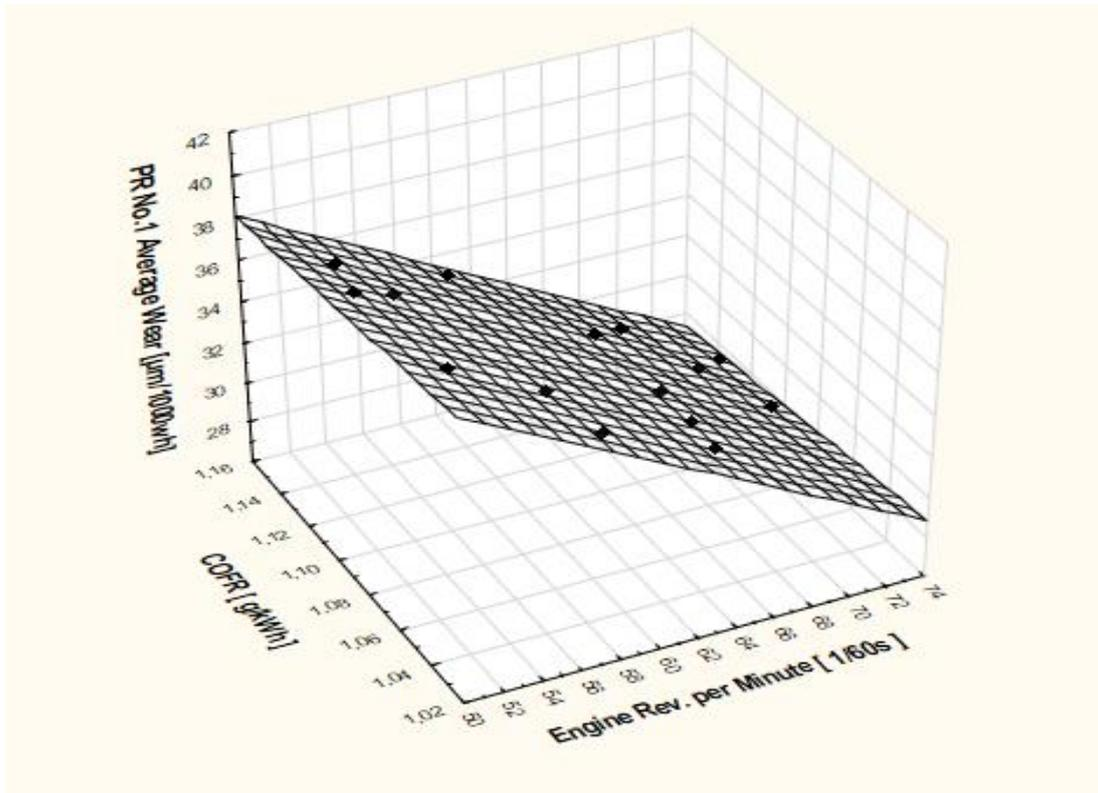
**Figure 3.** Results of average wear rates for PR No. 1 in all engine units, depending on COFR and the engine's RPM (piston speed).
