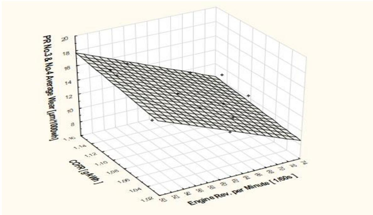
**Figure 5.** Results of average wear rates for PR No. 3 and 4 in all engine units, depending on COFR and the engine's RPM (piston speed).
