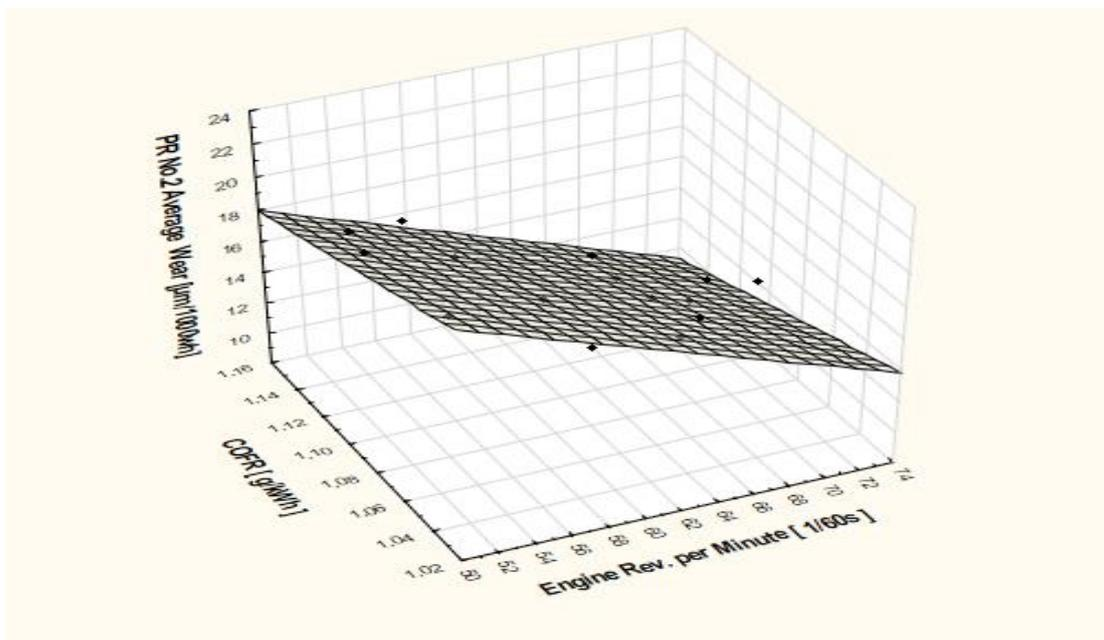
**Figure 4.** Results of average wear rates for PR No. 2 in all engine units, depending on COFR and the engine's RPM (piston speed).
