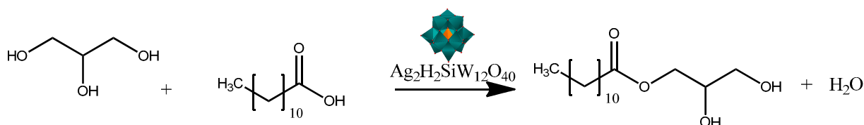
Scheme 4. Glycerol esterification with lauric acid over silver partially exchanged silicotungstate catalyst [56].
