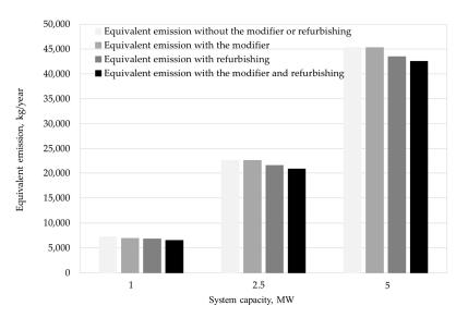
**Figure 7.** Equivalent emission (SO<sub>2</sub>, NO<sub>2</sub> and particulate matter) in fuel oil combustion for system capacities from 1 MW to 5 MW.
