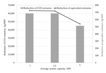
**Figure 5.** The size of emission reductions per 1 MW of capacity for the system for improving energy and ecological efficiency.
