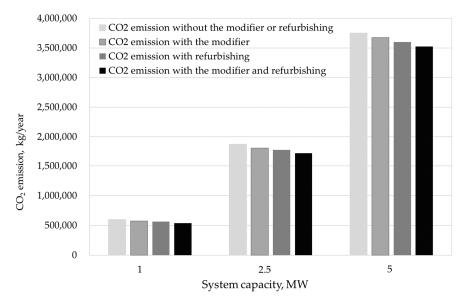
Figure 6. CO<sub>2</sub> emission in fuel oil combustion for system capacities from 1 MW to 5 MW.
