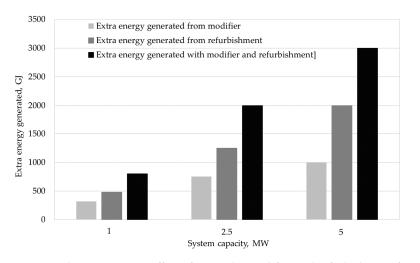
**Figure 3.** The extra energy effect of using the modifier and refurbishment for system capacities from 1 MW to 5 MW.
