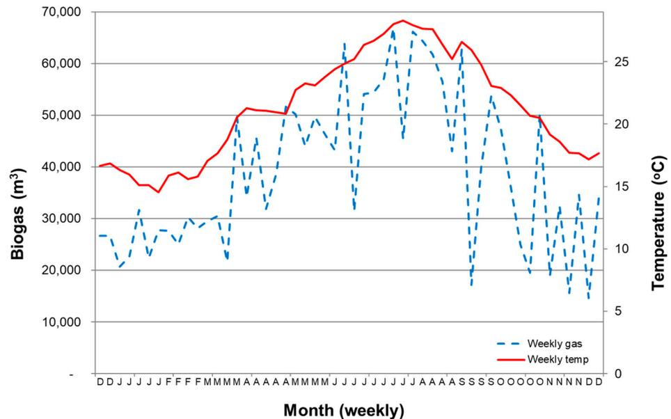
**Figure 4.** Weekly temperatures and biogas volumes for the second year of operation, starting with the last two weeks of December (D) of the previous year. The letters on the x-axis represent the weekly data for each month of year. The solid line is the temperature, and the dashed line is the biogas.
