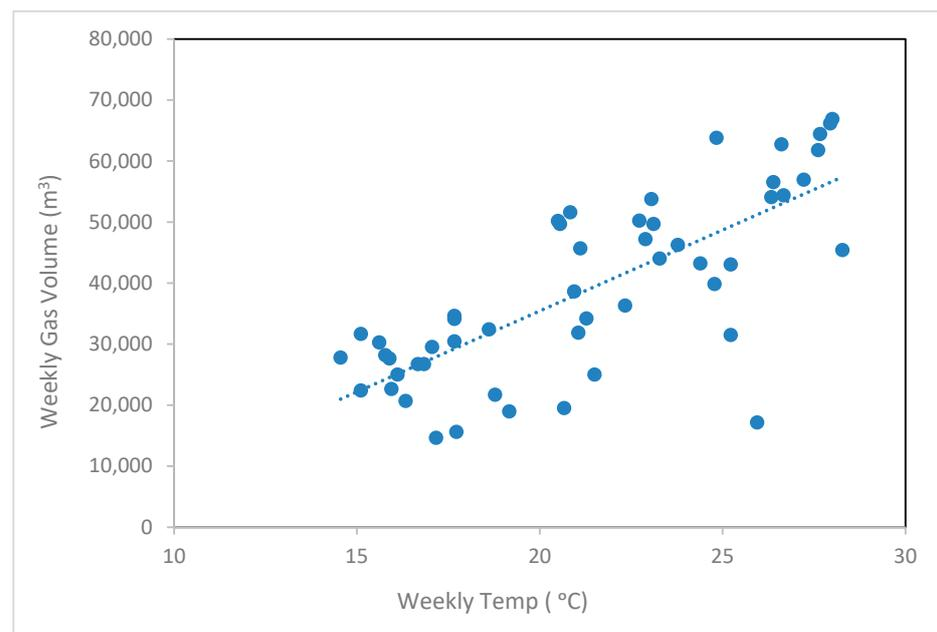
**Figure 5.** Linear regression of gas volumes (solid dots) versus temperatures showing a regression line (dashed line) with an  $R^2$  value of 0.57.
