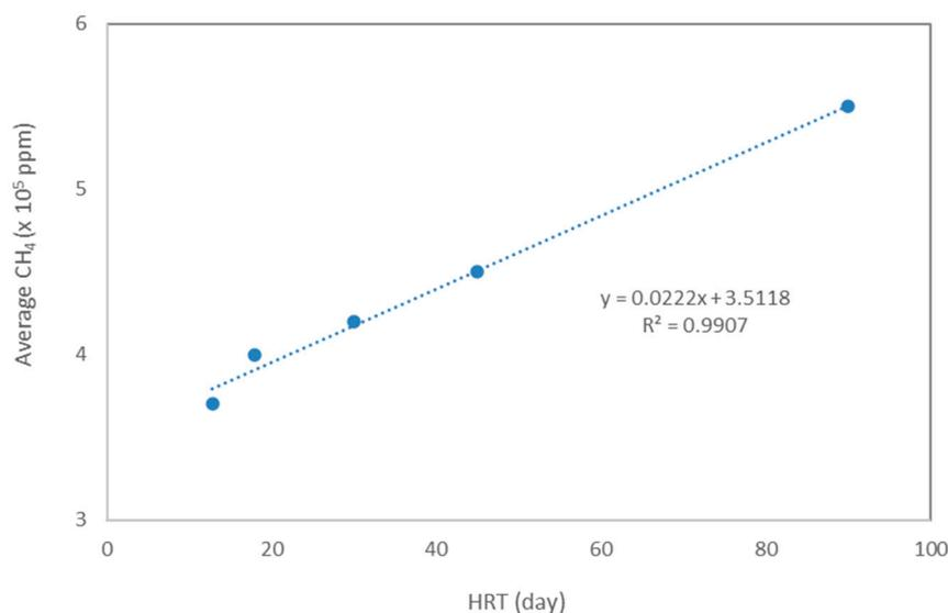
**Figure 9.** Linear regression line (dashed line) of hydraulic retention time (HRT) versus the average methane concentration ( $\times 10^5$  ppm) as solid dots with an  $R^2$  value of 0.99.
