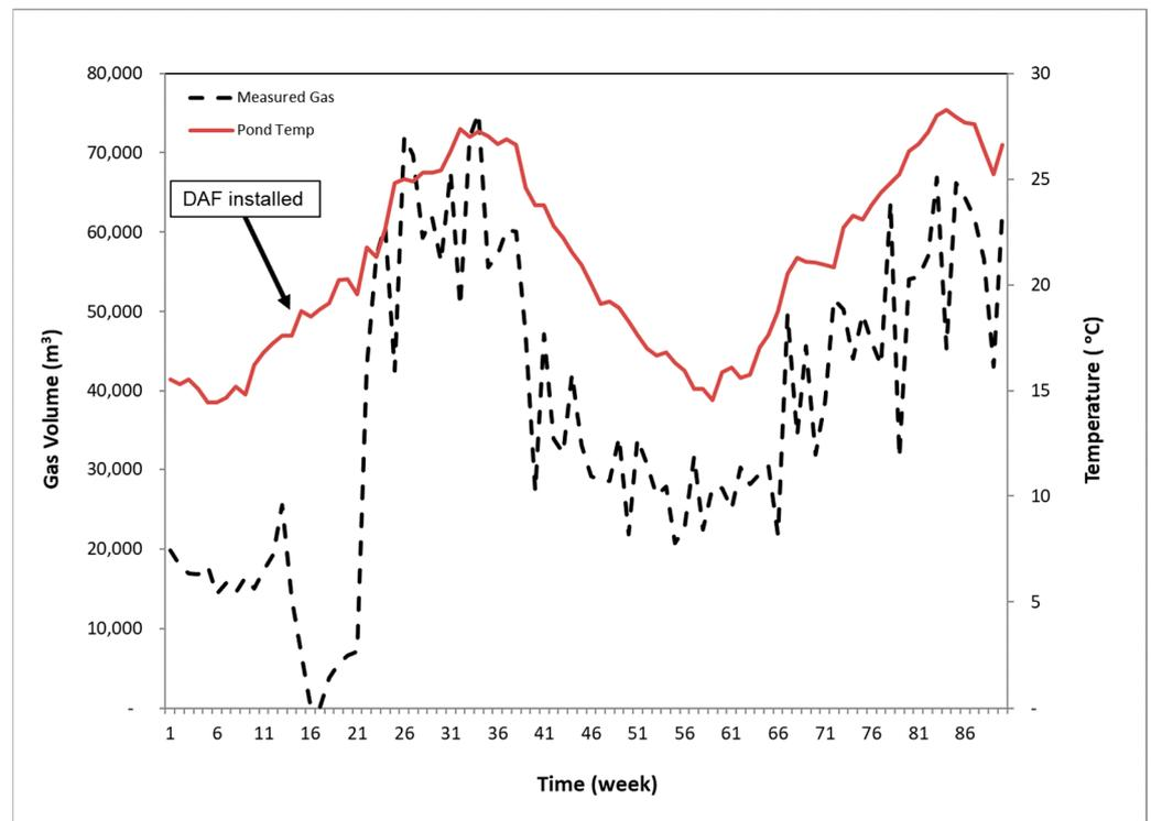
**Figure 7.** Weekly biogas volumes and temperatures of the lagoon anaerobic digester for the first two years of operation. A dissolved air flotation system (DAF) was installed in the second quarter of the first year. The solid line is the lagoon temperature, and the dashed line is the biogas volume.
