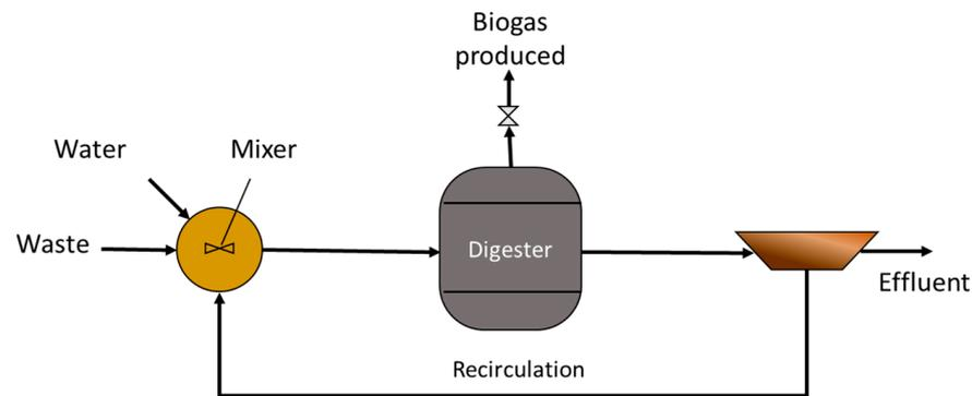
**Figure 1.** Schematic of anaerobic digestion of poultry rendering wastes.
