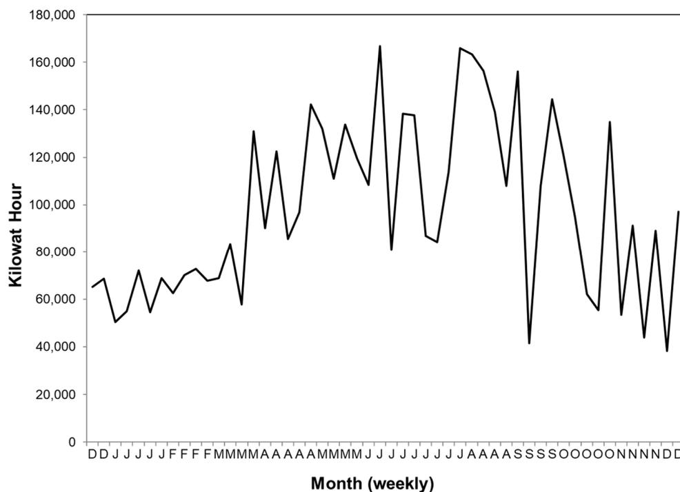
**Figure 6.** Weekly energy production (second year of operation) from December (D) to December in kilowatt-hours (kWh). The letters on the x-axis represent the weekly data for each month of the year.
