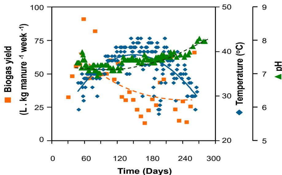
**Figure 8.** The effect of temperatures and pH on biogas yield using dairy manure as feedstock.
