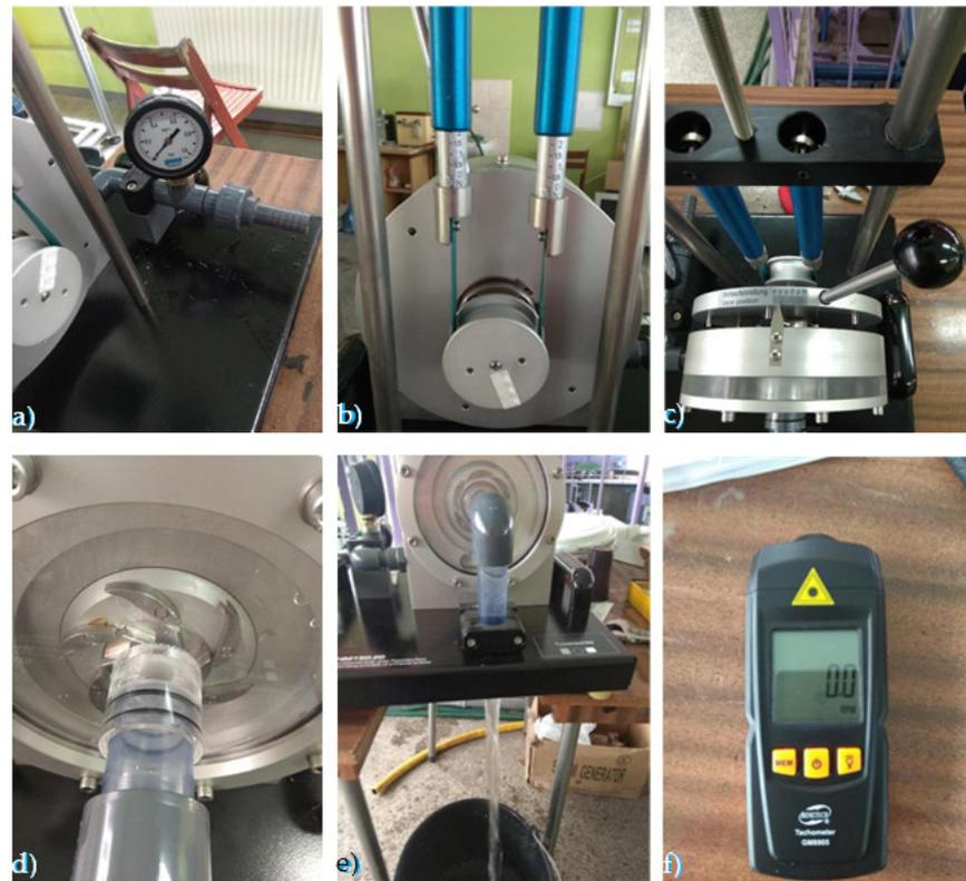
**Figure 2.** Turbine components used in the model tests: (a) inlet pipe with pressure gauge, (b) rotating shaft with weights, (c) control system, (d) impeller, (e) outlet pipe (K. Mastalerek), and (f) Benetech GM8905 laser tachometer (K. Mastalerek).
