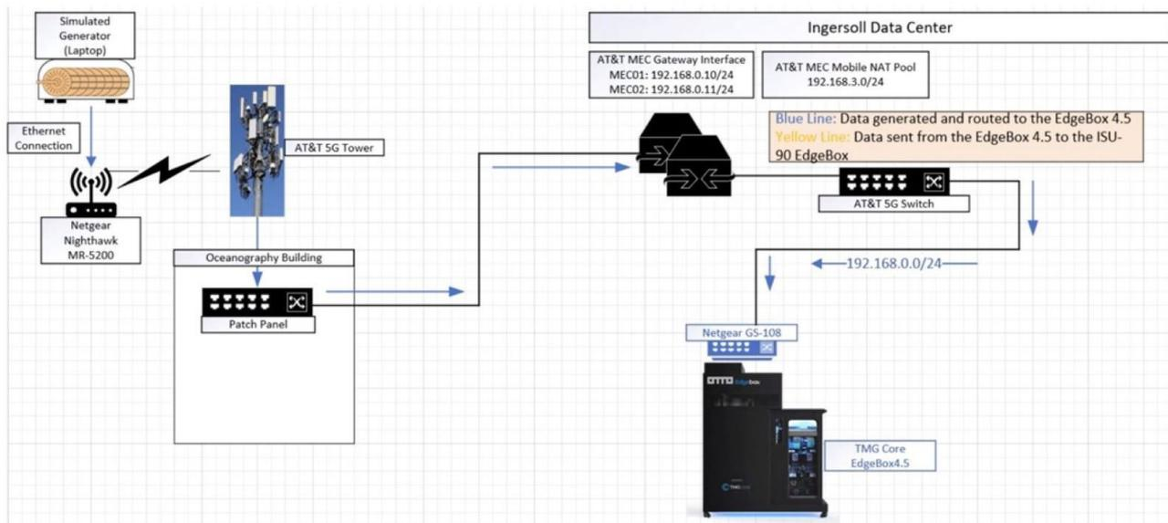
**Figure 2.** Experimental data path from the Nighthawk router to the EdgeBox to replay 5G data files and obtain 5G PCAP data.
