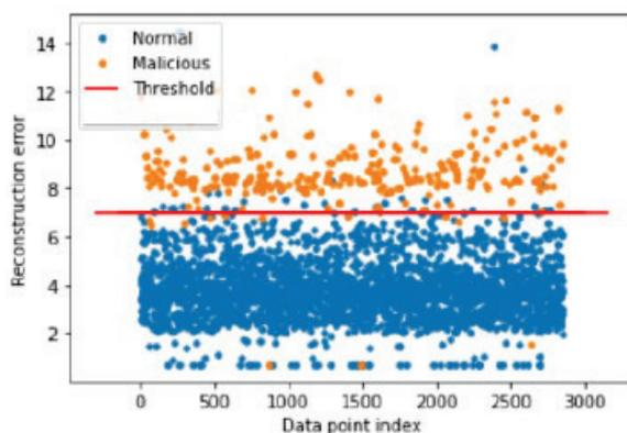
**Figure 11.** The graph depiction of the Efficient model separating data and plotting predictions on one NAVFAC data set that mimics an FDIA with 10% increase in AMI input values.
