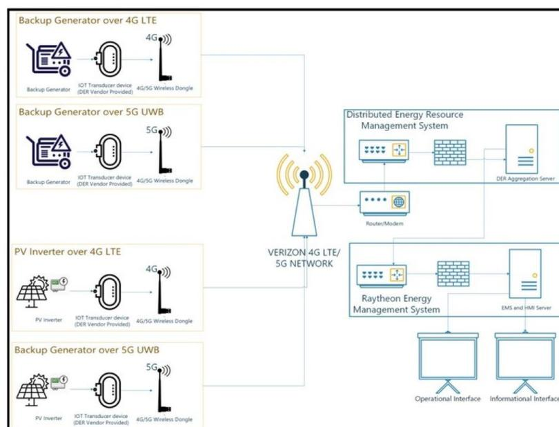
**Figure 1.** Generic system architecture for 4G LTE/5G control of PV and back up generators. Each DER is connected to an IoT transducer device, which is then connected to a 4G or 5G dongle which then forwards traffic to the Verizon 4G LTE/5G tower. The EMS is shown on the left side of the figure [7].
