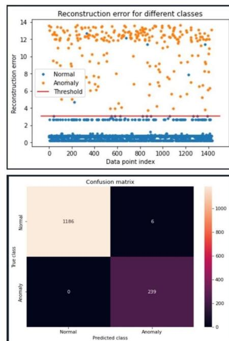
**Figure 8.** Efficient model with Modbus Data–DDoS attack detection results on the Modbus TCP/IP over Ethernet data set using the most efficient model tested. The model uses the LeakyRelu activation function and Adam optimizer along with both unit norm and tied weights.
