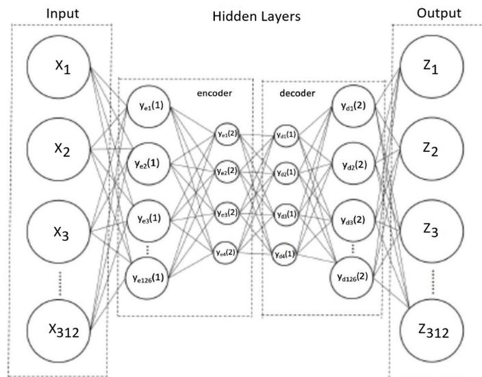
Figure 5. Model of Efficient autoencoder structure used in experiments.
