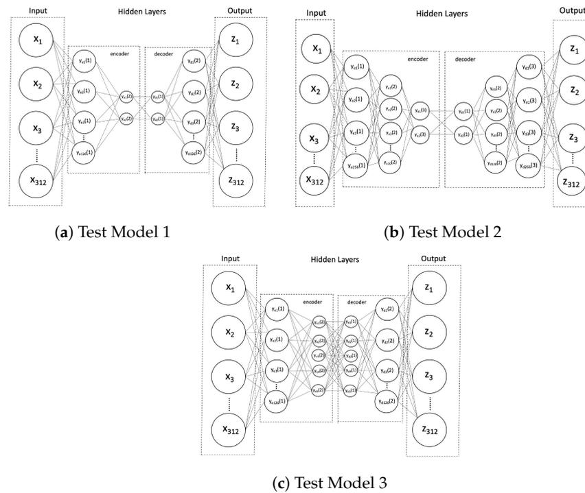
Figure 4. Depictions of the three test models used to identify the Efficient model that is used for anomaly detection training.
