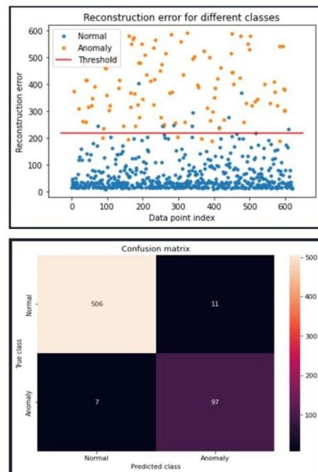
**Figure 9.** Deep model with 5G Data-DDoS attack detection results on the 5G PCAP data set using the Deep model. The model uses the LeakyRelu activation function and Adam optimizer along with both unit norm and tied weights.
