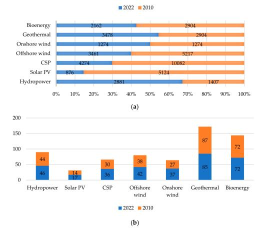
**Figure 14.** Total installed costs and capacity factor of RE technology. (a) Total installed cost of RE (UDS/kW), according to IRENA report in [146]; (b) RE capacity factor, according to the IRENA report in [146].
