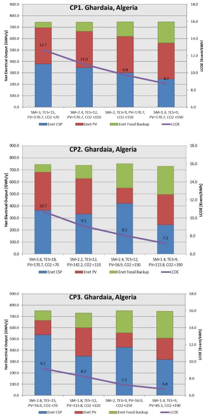
**Figure 7.** Energy production per configuration case (CP) and location. Solar multiple (SM), thermal storage capacity in full load hours (TES), nominal PV capacity in MW and CO<sub>2</sub> emissions in g CO<sub>2</sub>/kWh.
