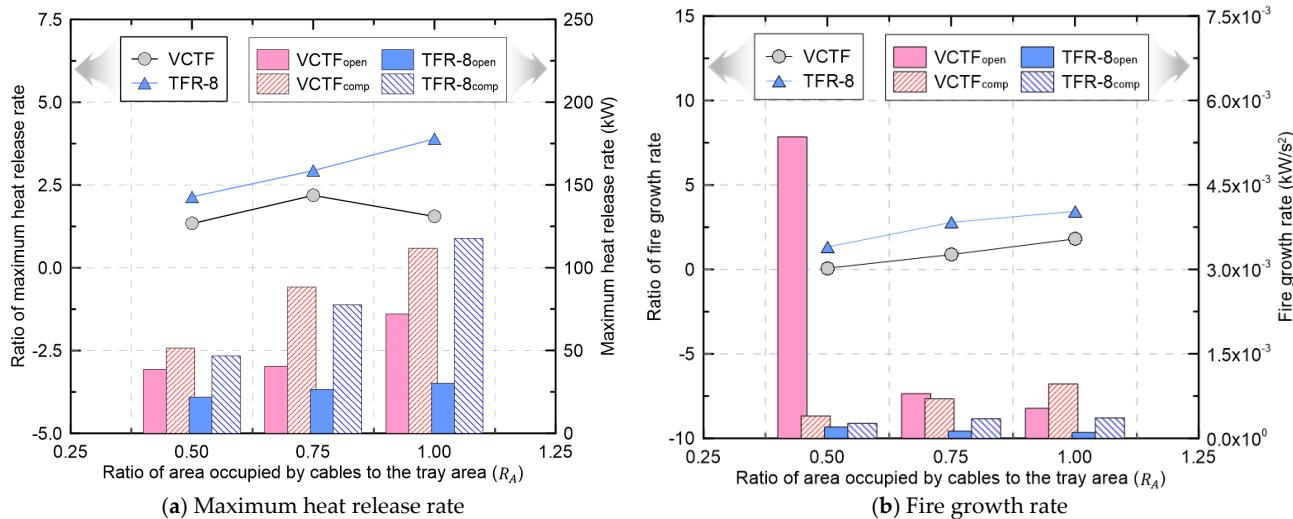
**Figure 13.** Changes in fire characteristics of the VCTF and TFR-8 cables between the open and compartment environments.
