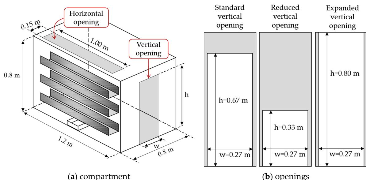
**Figure 3.** Schematic diagrams of the experimental setup to examine the burning characteristics of the cables in a compartment fire environment.
