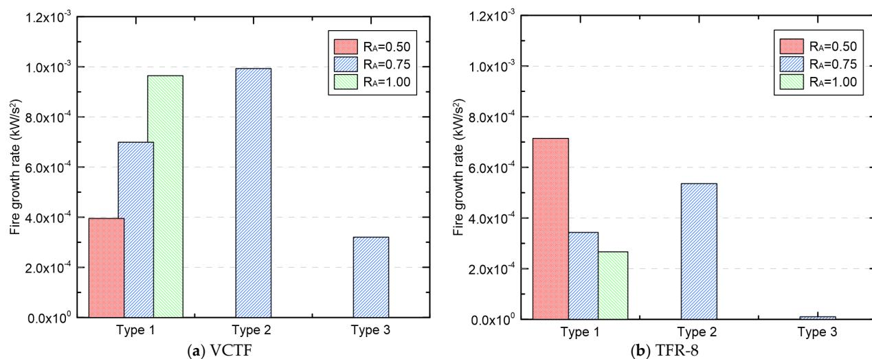
**Figure 12.** Comparison of the fire growth rate according to the quantity and arrangement method of cables in a compartment environment.
