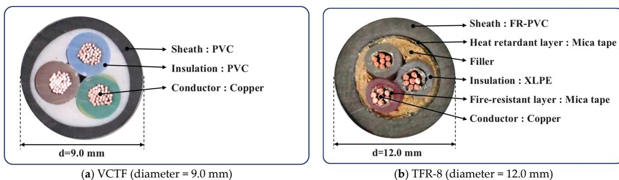
**Figure 1.** Cross-section photos of target cables and their constituent materials.
