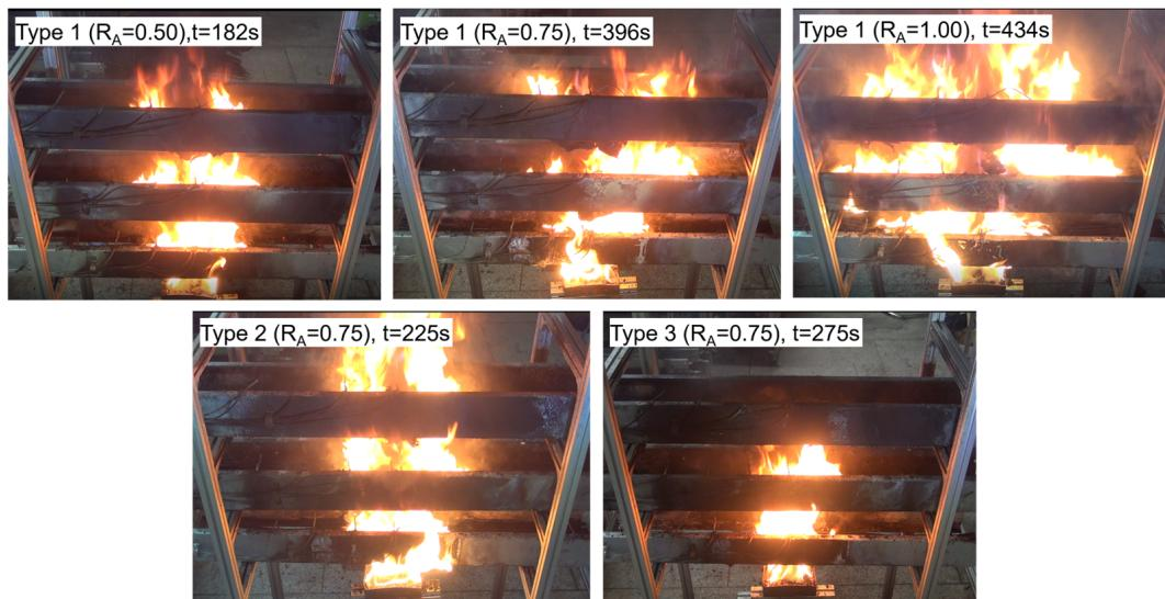
**Figure 5.** Photos of the flame at the moment of the maximum HRR according to the quantity and arrangement of the VCTF cable in an open environment.
