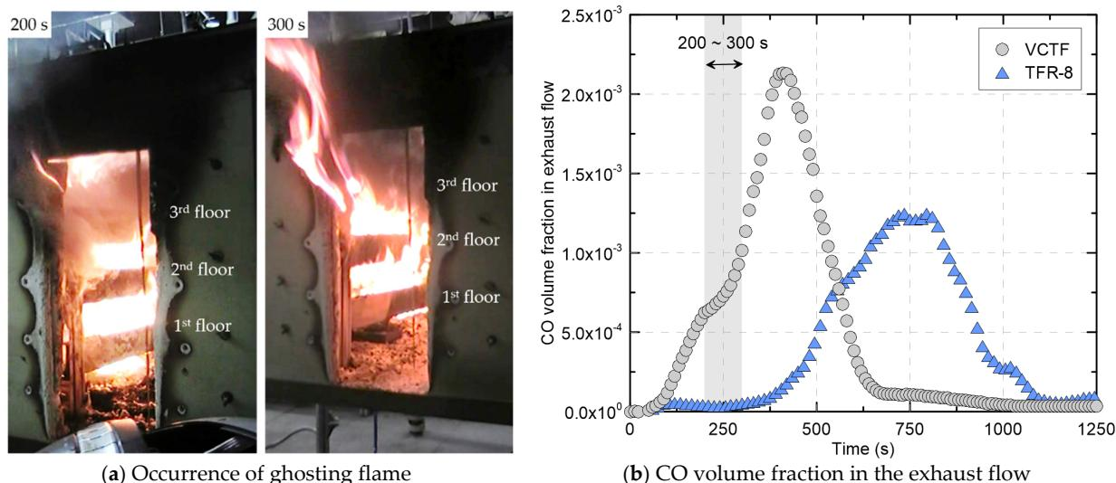
**Figure 14.** Fire phenomenon of the VCTF cables under the type 1 and  $R_A = 1.00$  condition.
