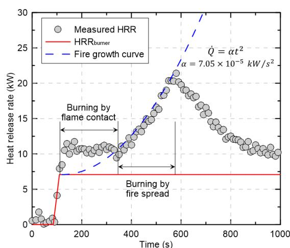
**Figure 4.** A fire growth curve to evaluate the fire growth rate using the measurement results of the TFR-8 cable (Type 1,  $R_A = 0.5$ ) in an open environment as an example.
