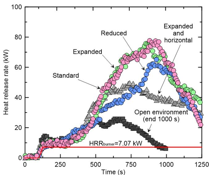
**Figure 16.** Comparison of the fire growth behavior for TFR-8 cables under various opening conditions.
