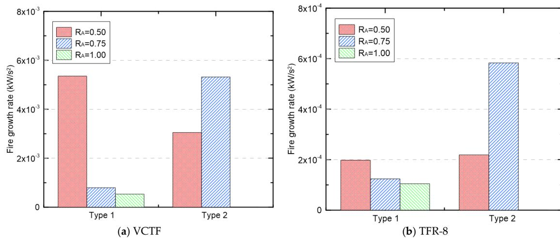
**Figure 8.** Comparison of the fire growth rate according to the quantity and arrangement method of cables in an open environment.
