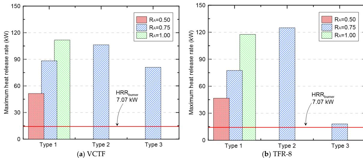
**Figure 11.** Comparison of the maximum heat release rate according to the quantity and arrangement method of cables in a compartment environment.
