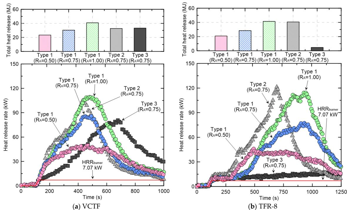
**Figure 10.** Comparison of the fire growth curve and total heat release according to the quantity and arrangement method of cables in a compartment environment.
