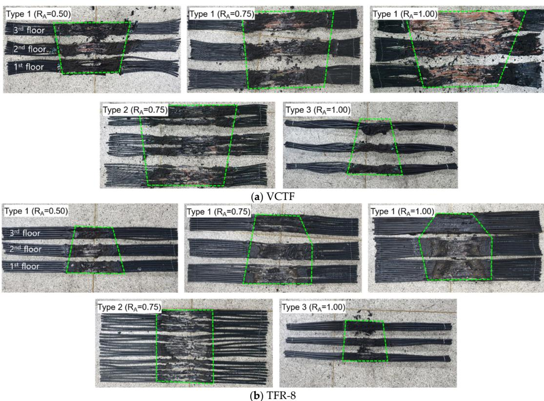
**Figure 9.** Comparison of the damaged area according to the quantity and arrangement method in an open environment.
