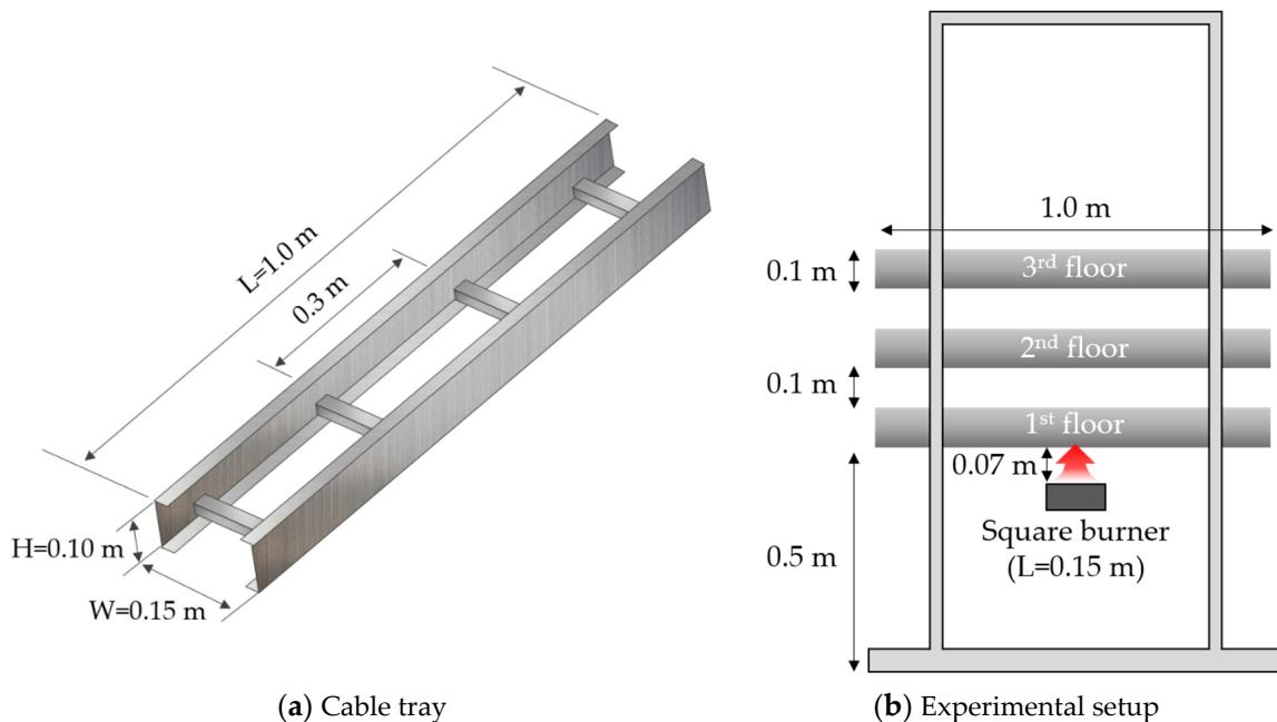
**Figure 2.** Schematic diagrams of the experimental setup to examine the burning characteristics of cables in an open environment.
