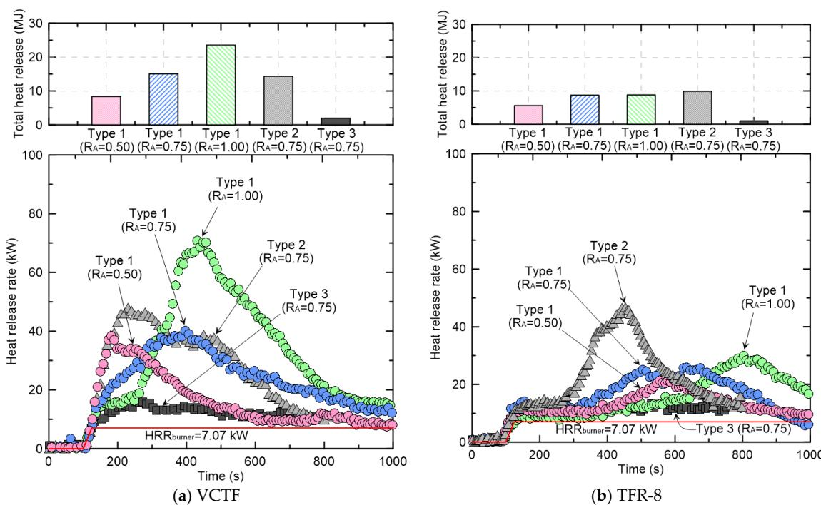
**Figure 6.** Comparison of the fire growth curve and total heat release according to the quantity and arrangement method of cables in an open environment.
