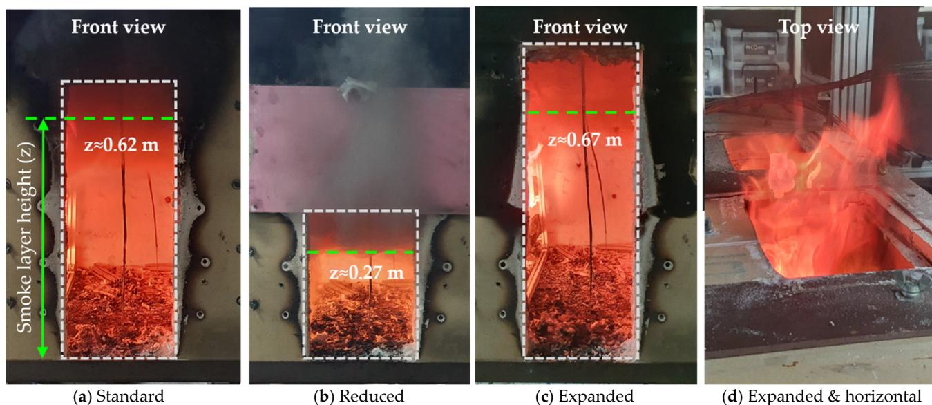
**Figure 15.** Comparison of the smoke layer height at the peak period under various opening shape conditions.
