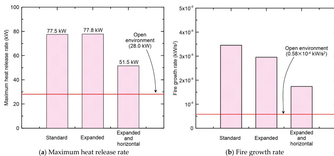
**Figure 17.** Comparison of the fire characteristics according to the opening shape to analyze the effect of thermal feedback from the smoke layer and walls.
