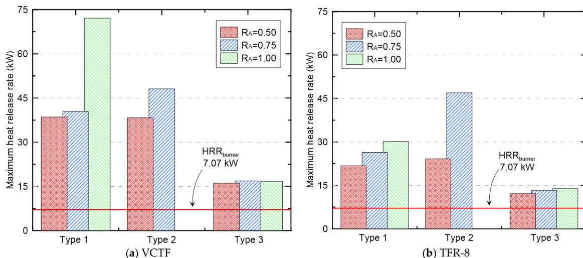
**Figure 7.** Comparison of the maximum HRR according to the quantity and arrangement method of cables in an open environment.
