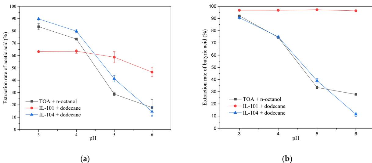
**Figure 1.** Extraction rates of acetic acid (a) and butyric acid (b) using different solvents at different pH.
