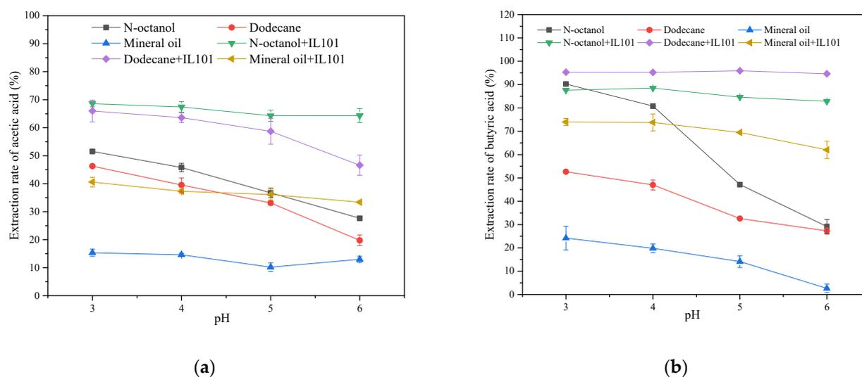
**Figure 2.** Extraction rates of acetic acid (a) and butyric acid (b) using IL 101 with different diluents.
