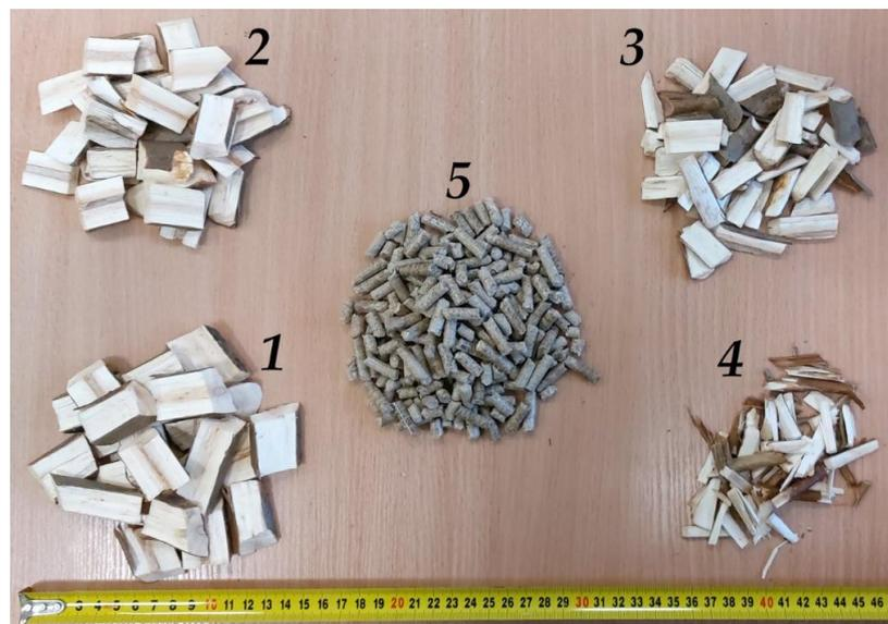
**Figure 2.** Fractional composition of the fuel from the biomass of a fast-growing willow *Salix Viminalis*: 1—a large fraction, 2—a medium fraction, 3—a small fraction, 4—a very small fraction, and 5—fuel pellets.
