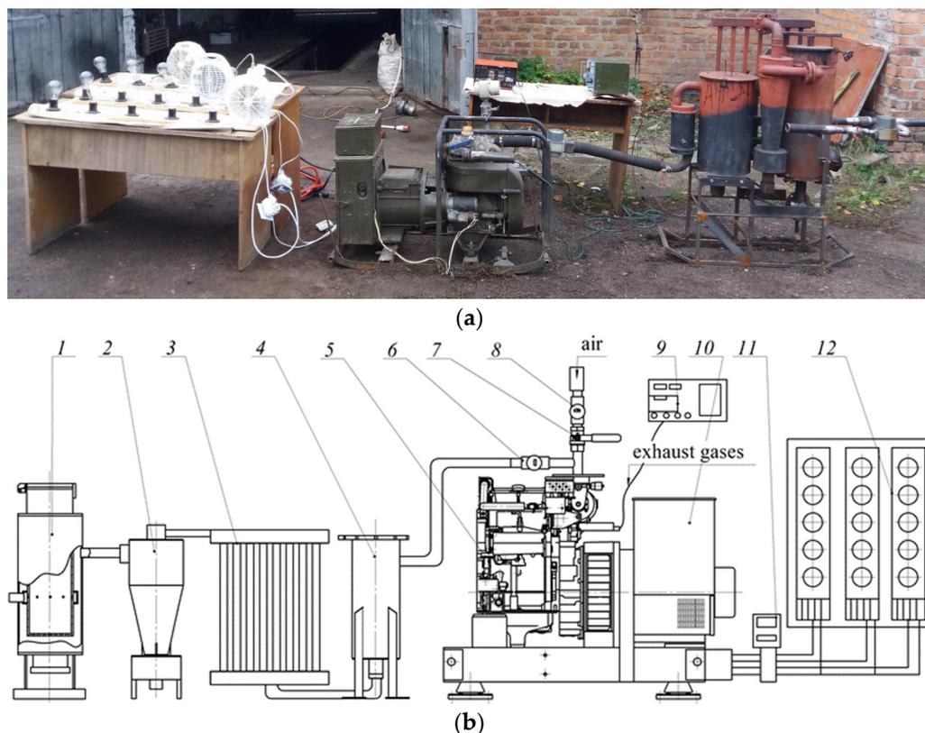
**Figure 3.** General view (a) and a scheme (b) of plant number 2 for conducting research: 1—a downdraft gasifier; 2—a filter for intermediate gas purification; 3—a refrigerator; 4—a filter for a final gas purification; 5—an internal combustion engine; 6—a gas meter; 7—a mixer for regulating the air supply into the engine; 8—an air meter; 9—an analyzer of the chemical composition of exhaust gases; 10—an electric generator; 11—wattmeter; and 12—a standard electrical load consumer.
