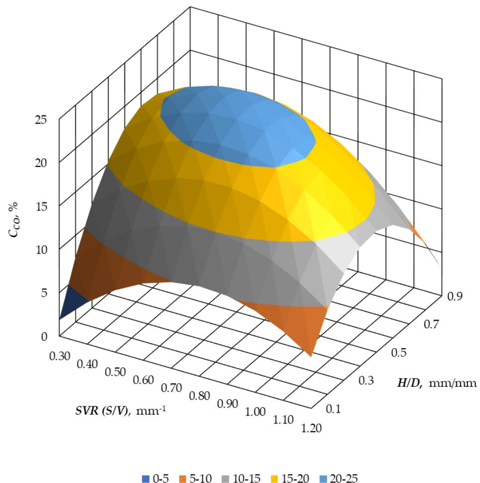
**Figure 4.** Graphic image of the dependence of CO concentration in the received gas on the ratio indicators of height to the reduction zone diameter ( $H/D$ ) and on the ratio of the full side area ( $S$ ) to the volume ( $V$ ) of a fuel fraction ( $SVR$ ).
