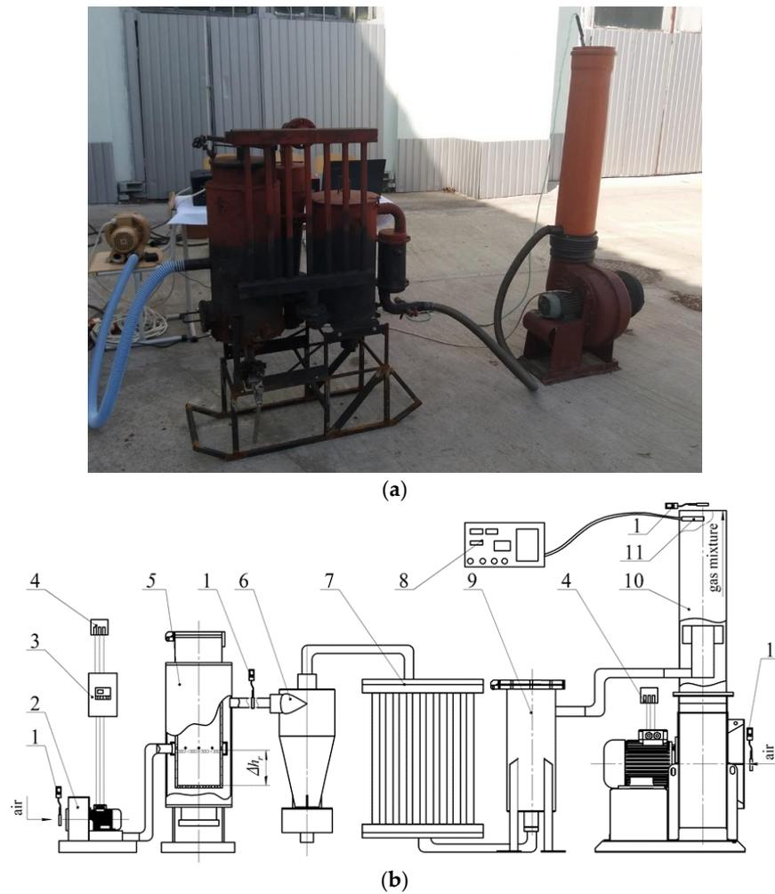
**Figure 1.** General view (a) and a scheme (b) of plant number 1 for conducting research: 1—an anemometer, 2—an air blower (an oxidant blower), 3—a frequency converter, 4—an electric power source, 5—a downdraft gasifier, 6—an intermediate purification filter, 7—a cooler, 8—a chemical analyzer of gas content, 9—a filter for final gas purification, 10—a mixer, and 11—an analyzer sensor 8.
