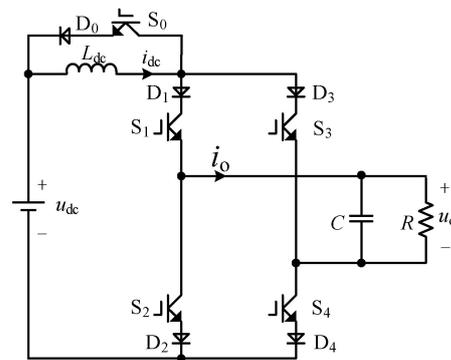
**Figure 1.** The topology of the proposed single-phase CSI.
