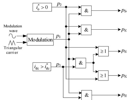
Figure 6. Logical conversion for the proposed single-phase CSI.
