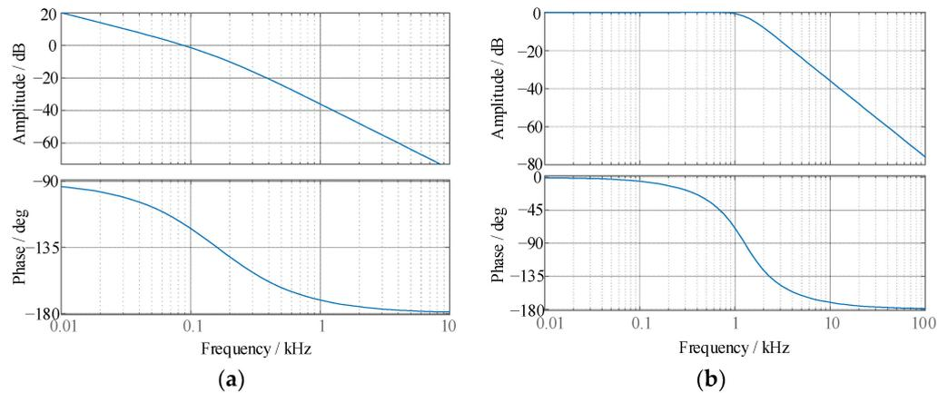
Figure 9. The Bode-plots of the output voltage control: (a)  $G_{open}(s)$ , (b)  $G_{close}(s)$ .
