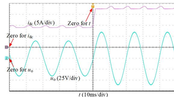
**Figure 14.** The dynamic-state experimental waveforms under amplitude changing.
