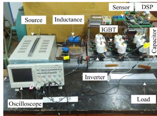
Figure 10. Experimental prototype of proposed single-phase CSI.
