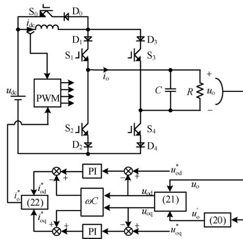
Figure 8. Control strategy diagram of output voltage.
