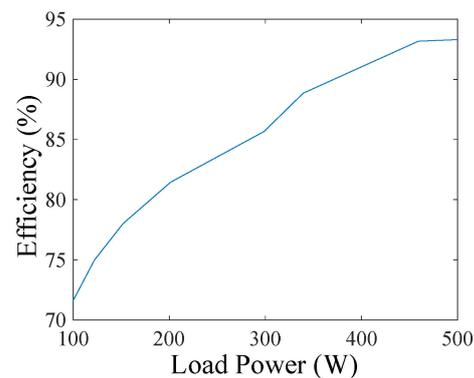
Figure 16. The efficiency map of the proposed single-phase CSI.
