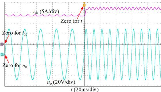
Figure 15. The dynamic-state experimental waveforms under frequency changing.
