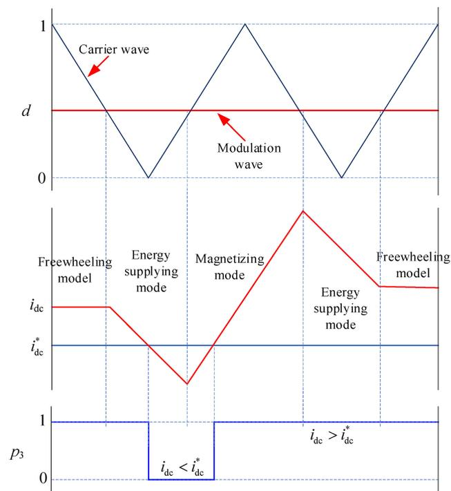
Figure 5. The changing process of  $i_{dc}$  and  $p_3$ .
