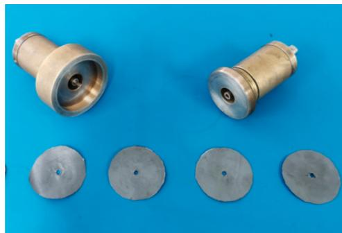
**Figure 9.** Specimens and coaxial fixture.
