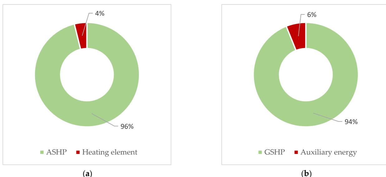
**Figure 18.** Electrical energy distribution for (a) ASHP and (b) GSHP.
