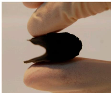
**Figure 19.** Picture of a  $\text{CoCp}_2$ @SWCNTs film fabricated by Fukumaru et al. Reprinted with permission [156].
