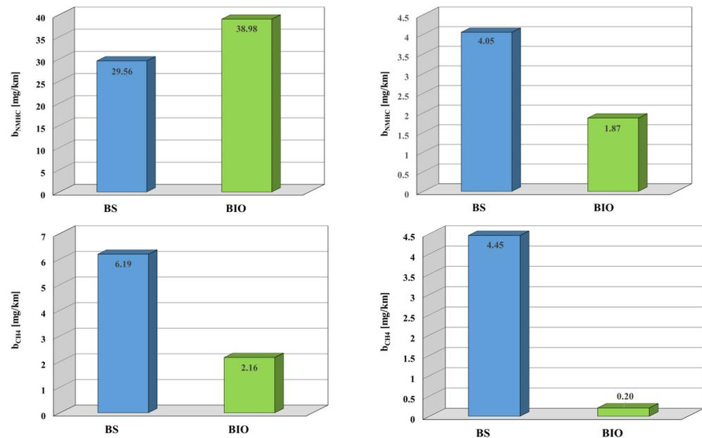
**Figure 2.** Average specific distance emissions of non-methane hydrocarbons and methane— $b_{NMHC}$  and  $b_{CH4}$  in the WLTC test when the car was supplied with motor gasoline (BS) and EtG fuel (BIO) at the start-up of a cold engine (diagrams on the left) and a hot engine (diagrams on the right). Measurement error  $\pm 5\%$ .
