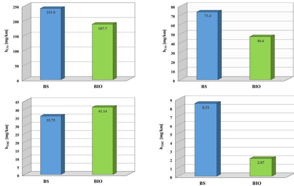
**Figure 1.** Average specific distance emissions of carbon monoxide and total hydrocarbons— $b_{CO}$  and  $b_{THC}$  in the WLTC test when the vehicle was running on petrol (BS) and EtG (BIO) fuel at the start-up of a cold engine (diagrams on the left) and a hot engine (diagrams on the right). Measurement error  $\pm 5\%$ .
