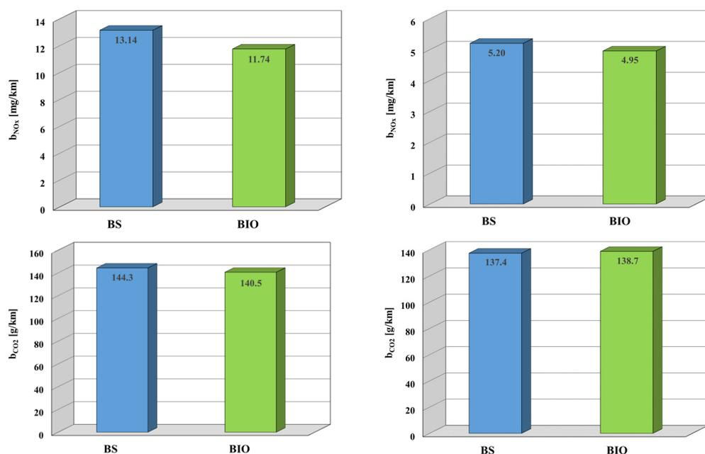
**Figure 3.** Average specific distance emissions of nitrogen oxides and carbon dioxide— $b_{NO_x}$  and  $b_{CO_2}$  in the WLTC test when the car is running on petrol (BS) and EtG (BIO) fuel at the start-up of a cold engine (diagrams on the left) and a hot engine (diagrams on the right). Measurement error for  $NO_x$  is  $\pm 5\%$ , and for  $CO_2$ — $\pm 3\%$ .
