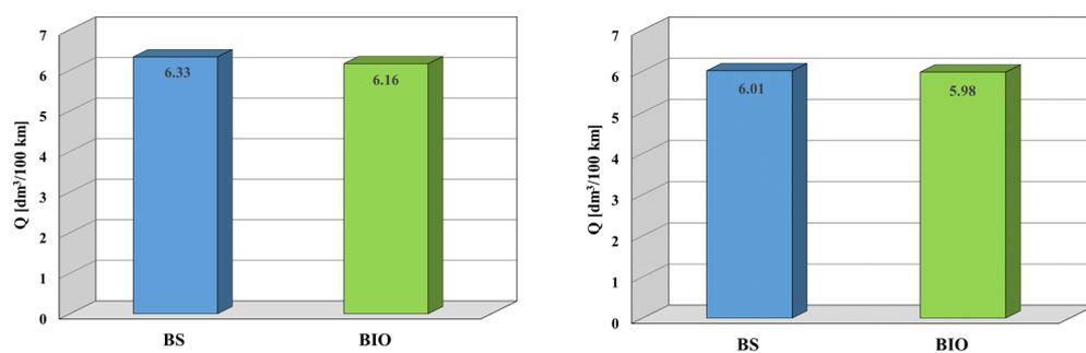
**Figure 4.** Operational fuel consumption— $Q$  in the WLTC test with the car is supplied with petrol—BS and BIO fuel when starting a cold engine (left-hand diagram) and a hot engine (right-hand diagram). Measurement error is  $\pm 3\%$ .
