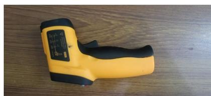
(b) Infrared thermometer heat gun
