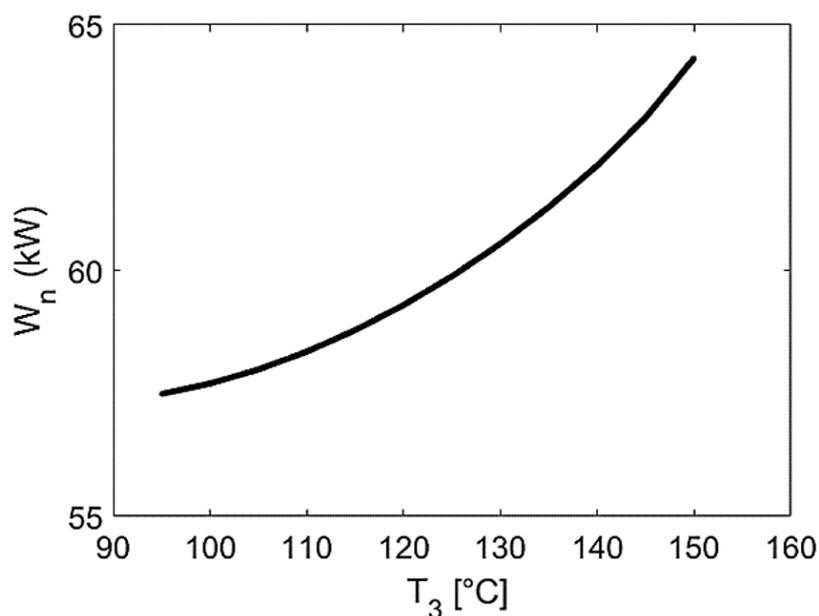
**Figure 5.** Effect of operation temperature in the net power output.
