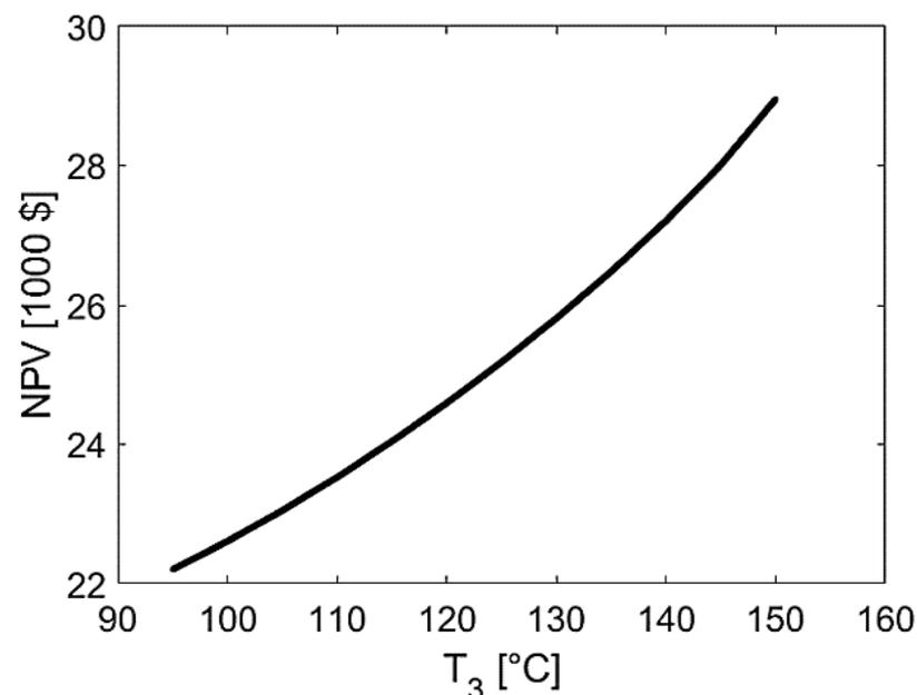
Figure 11. Effect of operating temperature on the net present value of the project.
