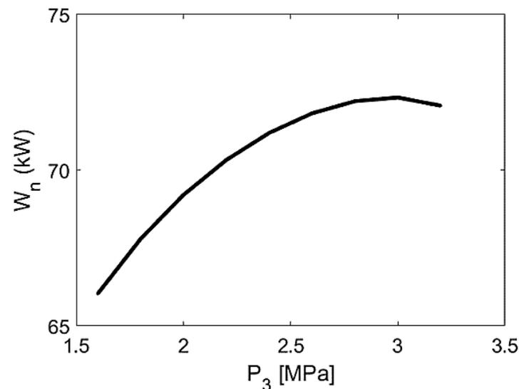
**Figure 7.** Effect of operating pressure on the net power output.
