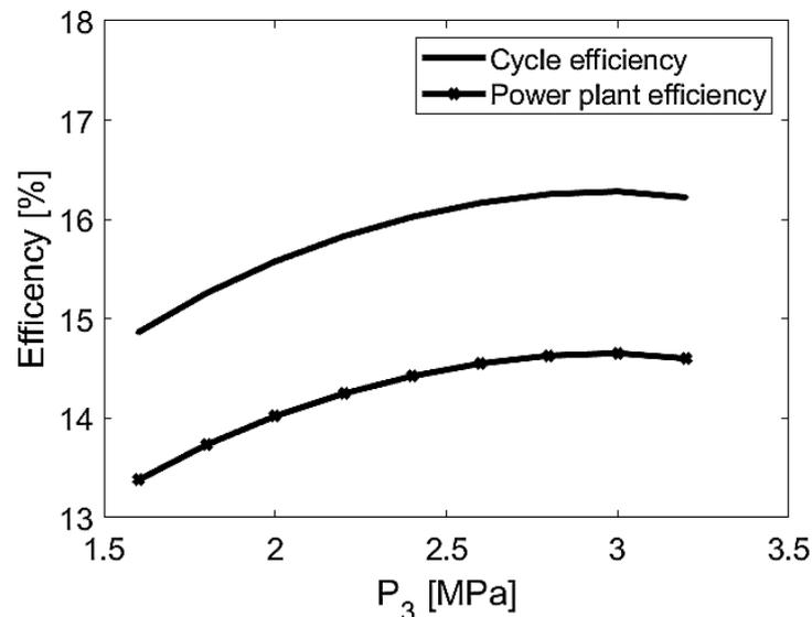
**Figure 8.** Effect of operating pressure on the efficiency of the system.
