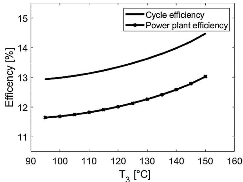
**Figure 6.** Effect of operating temperature on cycle and power plant efficiency.
