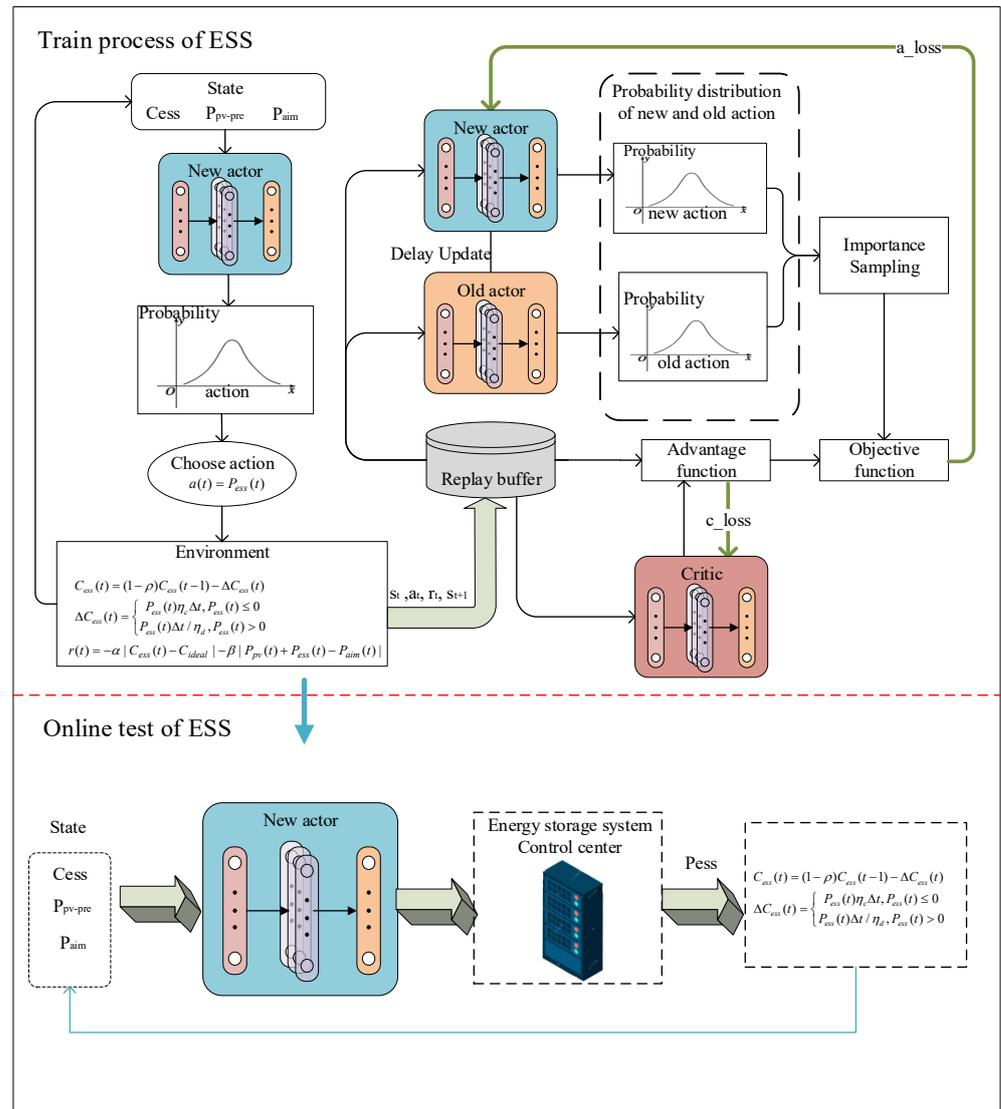
Figure 4. Control strategy based on the PPO algorithm.
