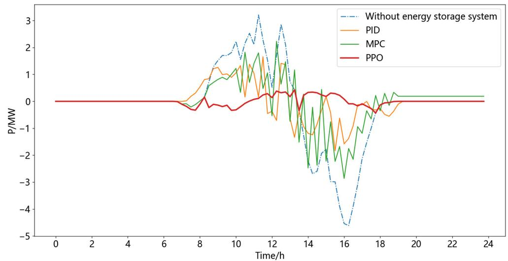
**Figure 10.** The average errors of tracking for no storage system, and two storage system with PID, MPC, and PPO.
