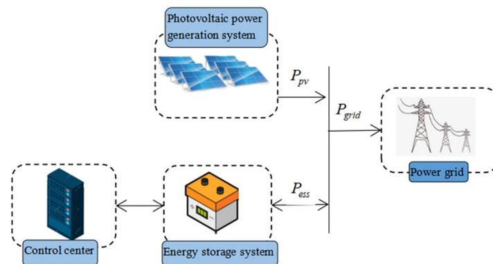
**Figure 1.** Photovoltaic and energy storage hybrid system.
