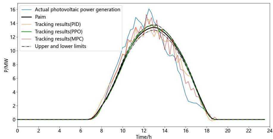
**Figure 7.** Tracking results of the power generation plan.
