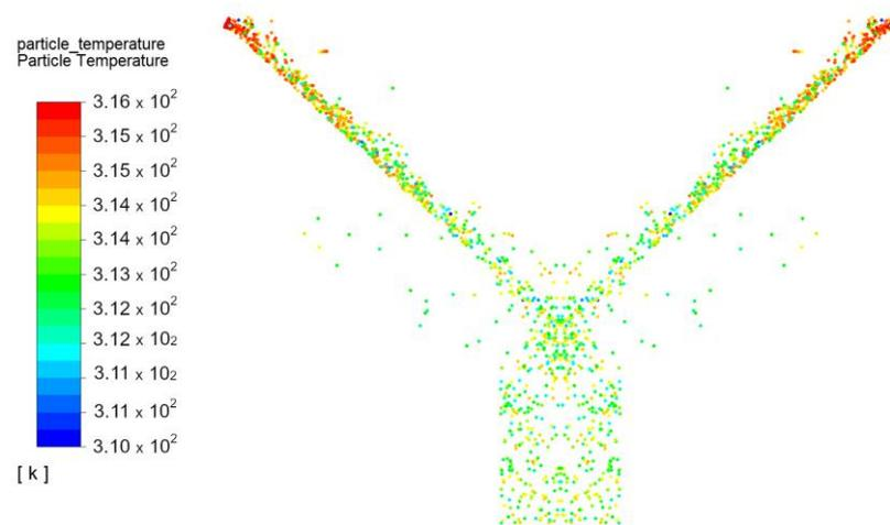
**Figure 2.** Distribution and temperature of particles at 6 s.
