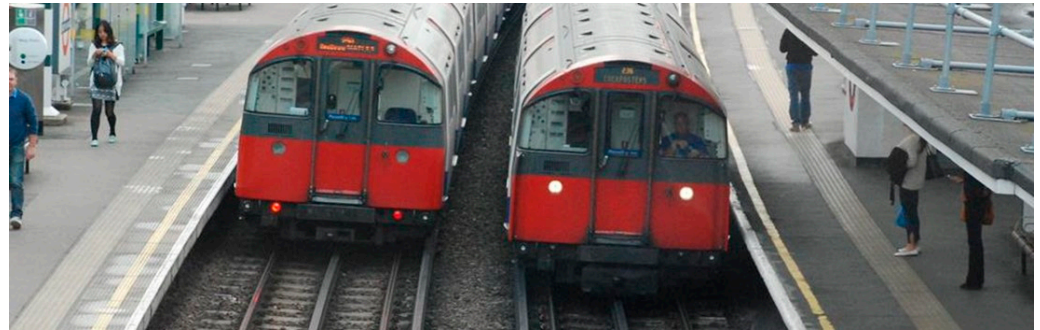
Figure 2. Third rail system in operation in the London underground adapted from [18] (Andrew Riley [CC BY-SA 4.0 ( https://creativecommons.org/licenses/by-sa/4.0/ )]).
