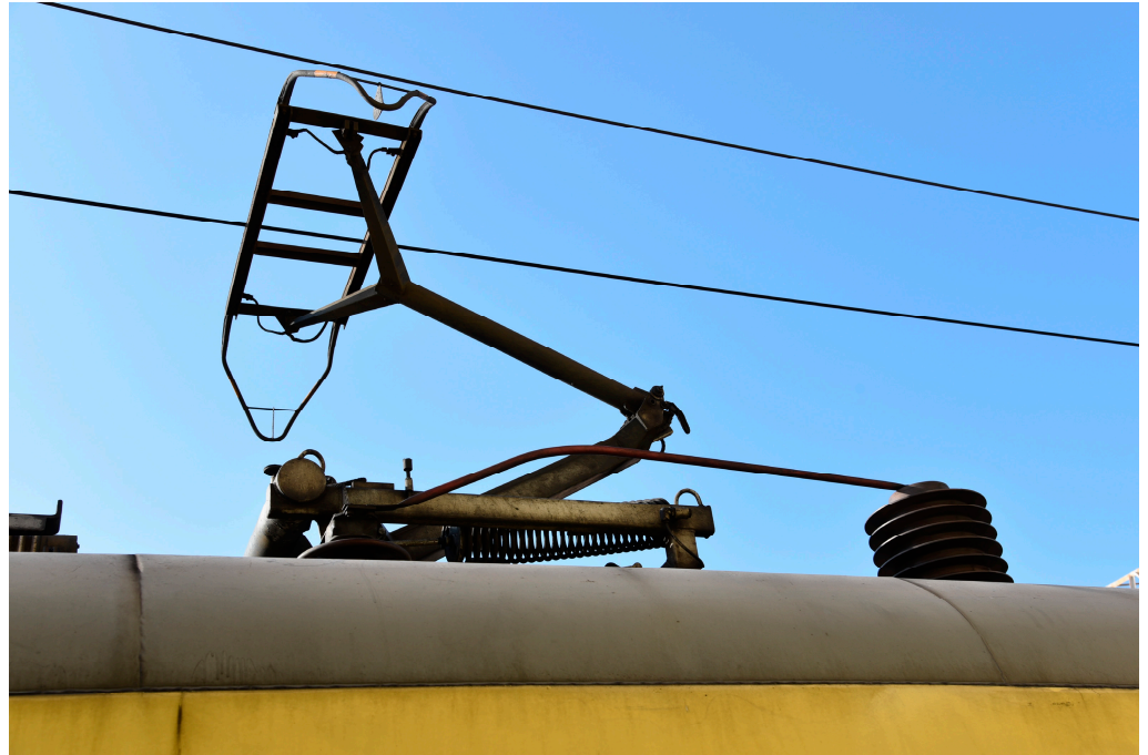
Figure 1. Light rail vehicle with pantograph/OCS power system. Adapted from [10] (Brecknell Willis [CC BY-SA 4.0 ( https://creativecommons.org/licenses/by-sa/4.0/ )]).
