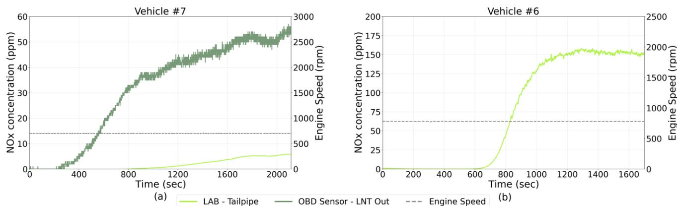
**Figure 4.** NO<sub>x</sub> concentration profiles at tailpipe (solid light green line) from vehicle #7 (a) and #6 (b) during hot idling test (both measured by CLD analysers). (a) also includes NO<sub>x</sub> sensor signal at the LNT outlet (solid dark green line), available at the OBD port. Engine speed (dashed grey line) is reported on the secondary axis. Time scale of both (a,b) starts at the end of the warm-up phase.
