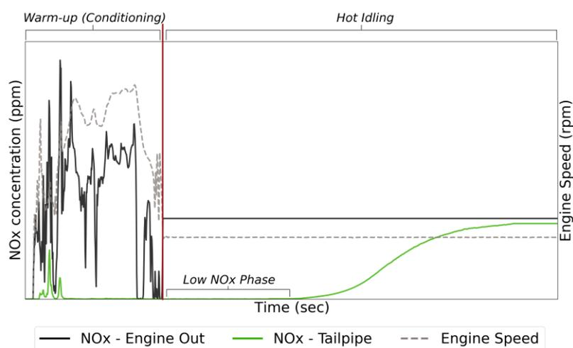
**Figure 1.** Simplified schematic representation of the hot idling procedure. NO<sub>x</sub> concentration and engine speed displayed are indicative.
