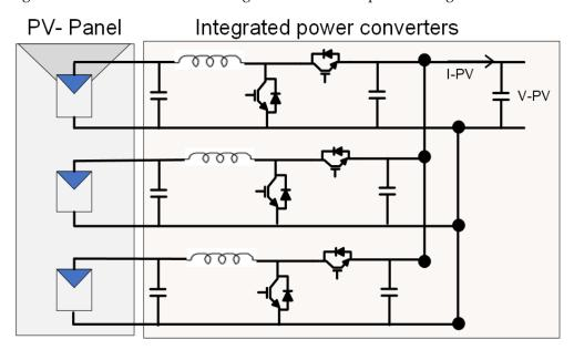
**Figure 13.** The connection between the PV sub-module and sub-panel micro converters of a single PV panel.
