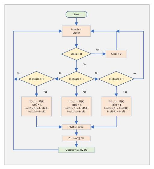
Figure 12. A flow chart illustrating the MPP algorithm according to the current of the PV SMs.
