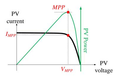
Figure 6. Generic current-voltage and power-voltage curves for a PV module.
