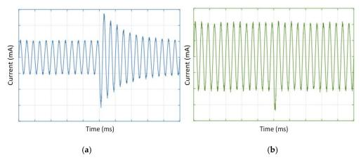
**Figure 2.** Experimental results for inverters during faults with a (**a**) slow dynamic response and (**b**) fast dynamic response (10 ms/div–5 A/div).
