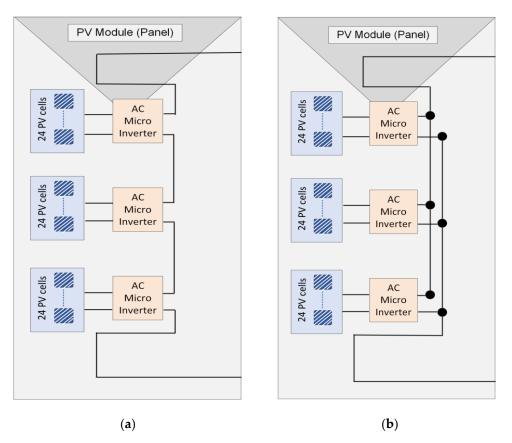
Figure 8. Sub-module grid-connected micro inverter: (a) Series-connected MI and (b) Parallel-connected MI.
