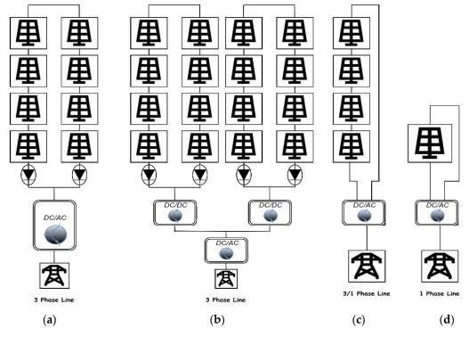
**Figure 4.** The grid-connected PV system classification according to DMPPT level: (**a**) single central PV inverter; (**b**) multi-central PV inverter; (**c**) string PV inverter; (**d**) PV module MI.
