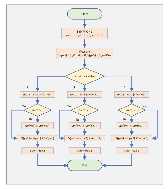
Figure 14. The flowchart shows the unified MPPT algorithm for capturing the MPP of PV sub-modules.
