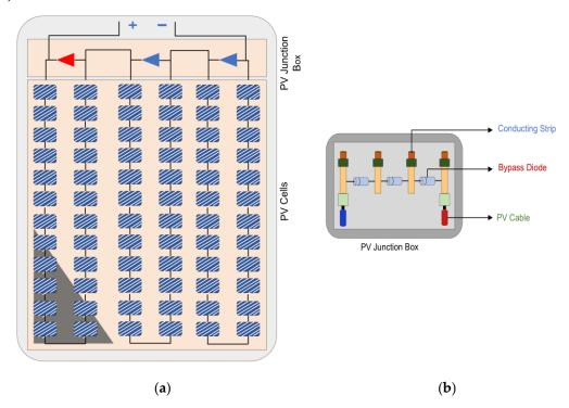
**Figure 7.** A standard 72-PV-cell panel circuit diagram: (**a**) the structure of the series connection of a 72-solar-cell PV panel and (**b**) the integrated junction box of the 72-cell PV panel.
