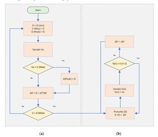
the next tracking cycle can be decided by comparing the voltage of the current cycle with the voltage of the previous tracking cycle.
