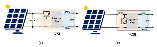
Figure 3. Generic configurations for DC/AC inverters: (a) VSI; (b) CSI.
