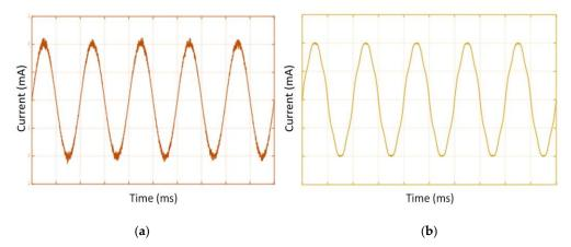
**Figure 1.** Experimental results for inverters with a (**a**) high-order harmonic current and (**b**) low-order harmonic current (10 ms/div–5 A/div).
