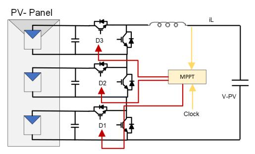
Figure 11. Configuration of the optimized buck-based MPPT system.
