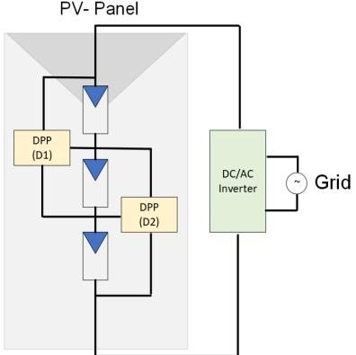
Figure 15 illustrates the DPP PV–PV architecture that is used to mitigate mismatch issues between the PV SMs.
