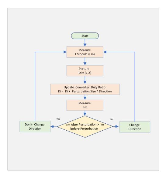
**Figure 16.** A flowchart illustrating the algorithm for operating the DPP and balancing the current between PV SMs.
