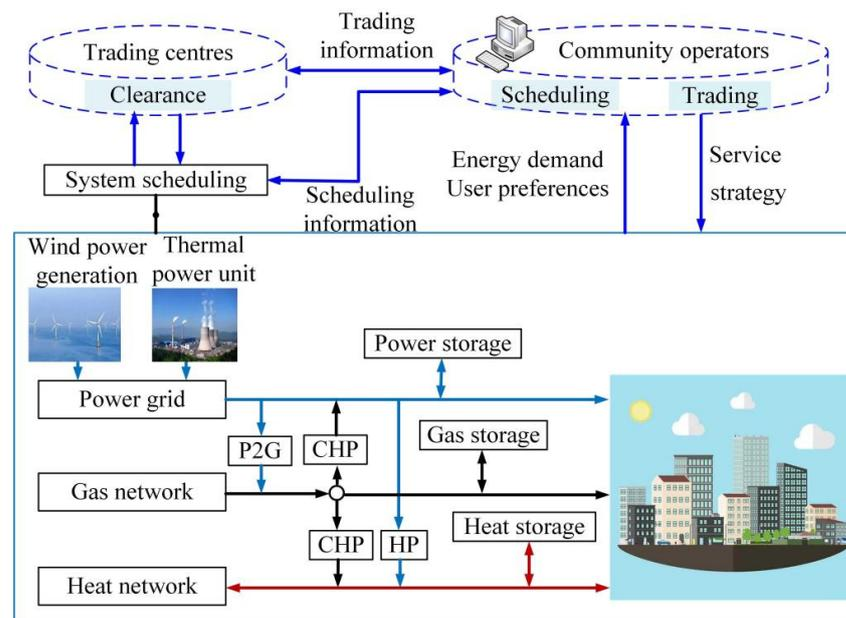
**Figure 1.** Structure diagram of the integrated energy system.
