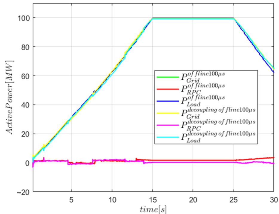
Figure 9. Comparison of active power profiles with and without decoupling lines at 100  $\mu$ s (offline).
