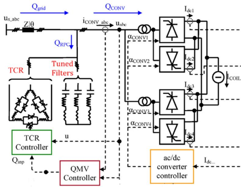
Figure 4. RPC and CS Converter Unit.
