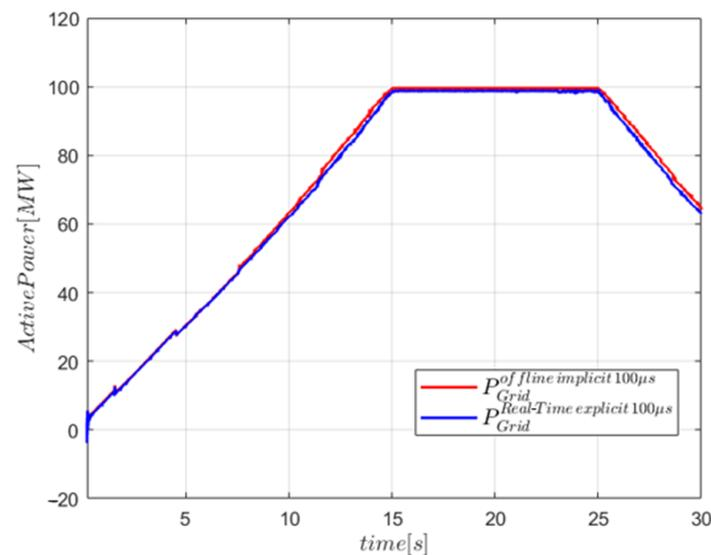
**Figure 13.** Load active power, model with two CUs—two decoupling lines—three Model References.
