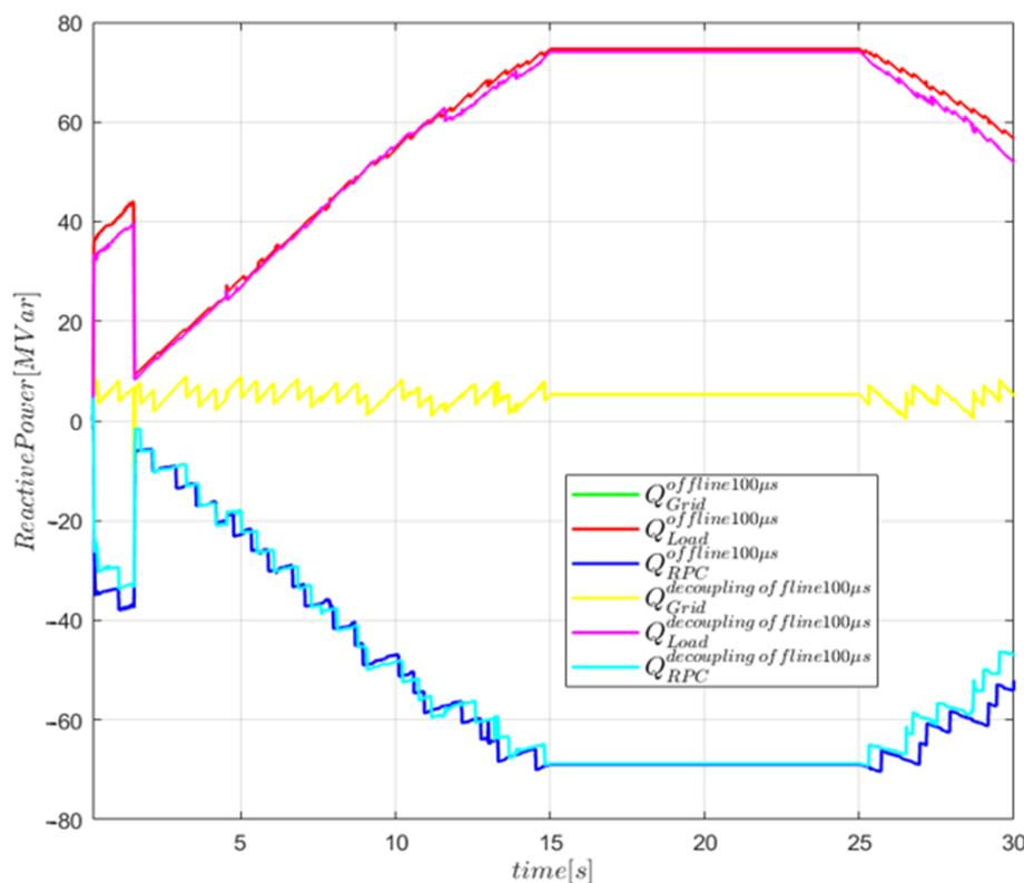
Figure 10. Comparison of reactive power profiles with and without decoupling lines at 100 μs (offline).
