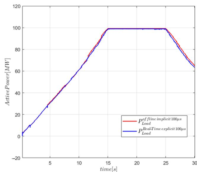
**Figure 12.** Grid active power, model with two CUs—two decoupling lines—three Model References.
