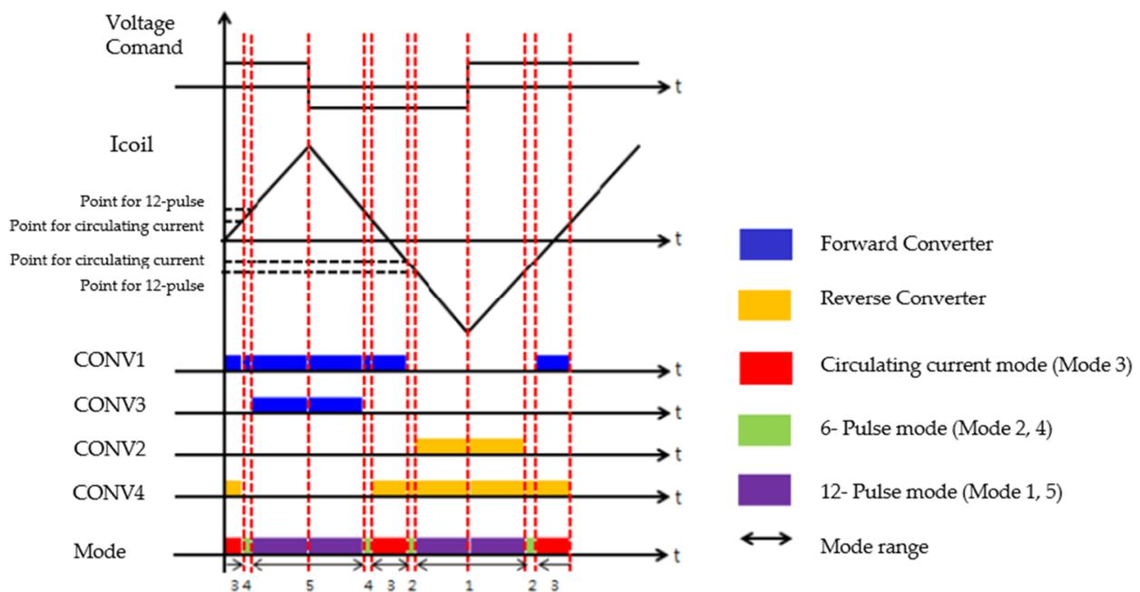
**Figure 5.** Voltage command, coil current, and control modes.
