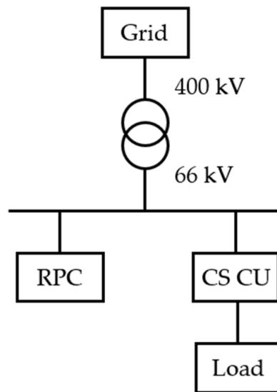
Figure 3. CS Power Supply grid scheme.
