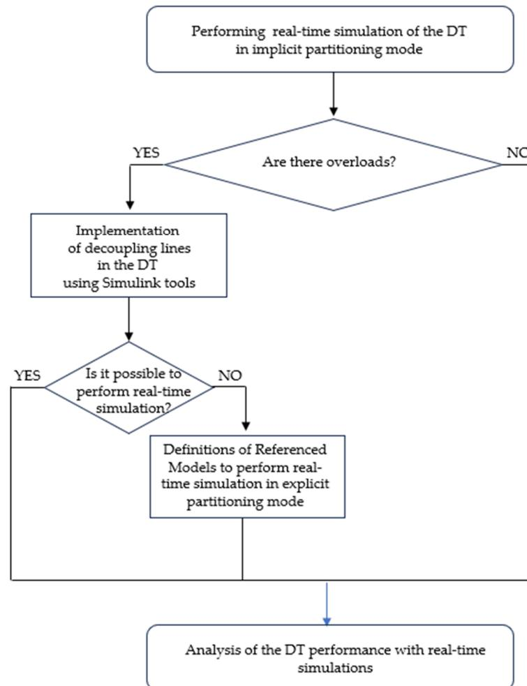
**Figure 2.** Flowchart of the progressive approach for real-time simulation of complex DTs.
