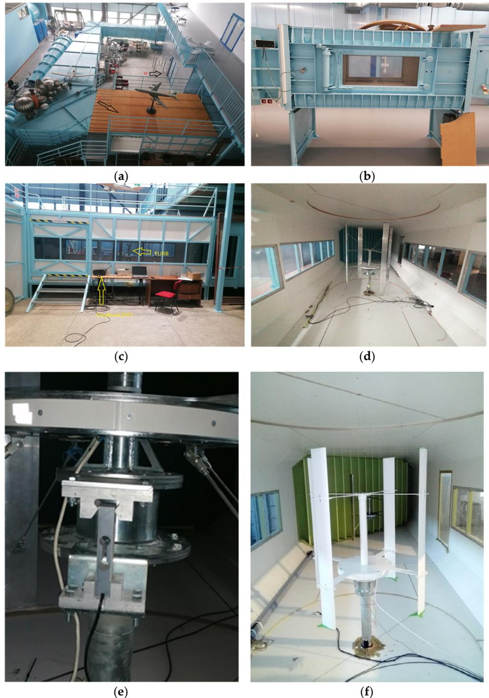
**Figure 4.** Aerodynamic measurement station. (a) Top view of the tunnel: small measurement space for high speeds and larger measurement space for low speeds. (b) Section of the tunnel with a high-
