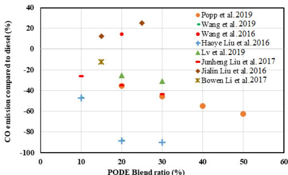
Figure 7. Variation in carbon monoxide emissions with different PODEn blend ratios compared to diesel [31–33,36,40,41,45,47].
