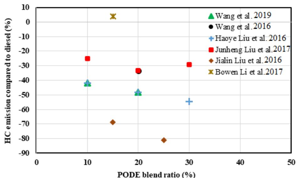
Figure 6. Effect of PODEn blend ratio on hydrocarbon emissions [31–33,36,41,45].
