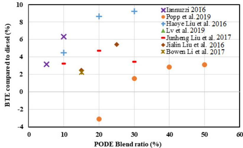
Figure 3. Effect of PODEn blend ratio on brake thermal efficiency compared to diesel [16,30,32,33,36,40,47].
