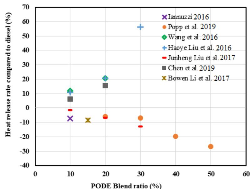
**Figure 2.** Effect of PODEn blend ratio on heat-release rate compared to diesel [16,30,32,33,40,45,52].
