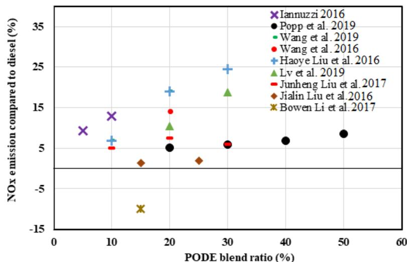
Figure 4. Variation in oxides of nitrogen with different PODEn blend ratios [16,31–33,36,40,41,45,47].
