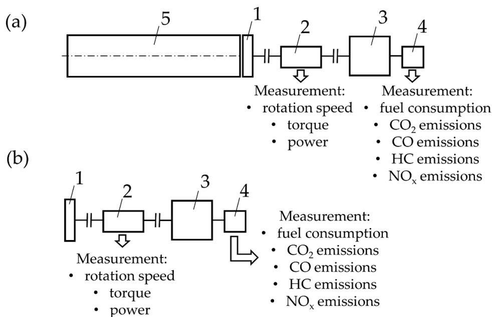
**Figure 2.** Diagram of the test stand: (a) measurement during duct flow test (Method A); (b) measurement during open flow test (Method B), where 1—fan impeller, 2—torque meter with speed measurement function, 3—combustion engine, 4—PEMS, and 5—air flow measurement channel.
