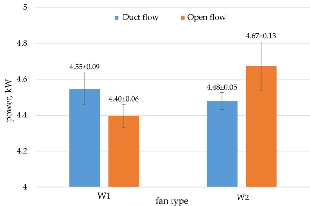
**Figure 6.** Mean power during tests with Methods A (duct flow) and B (open flow), where W1—fan with conventional impeller, W2—fan with turbo impeller. All mean values were determined at a 95% confidence interval ( $p = 0.05$ ).
