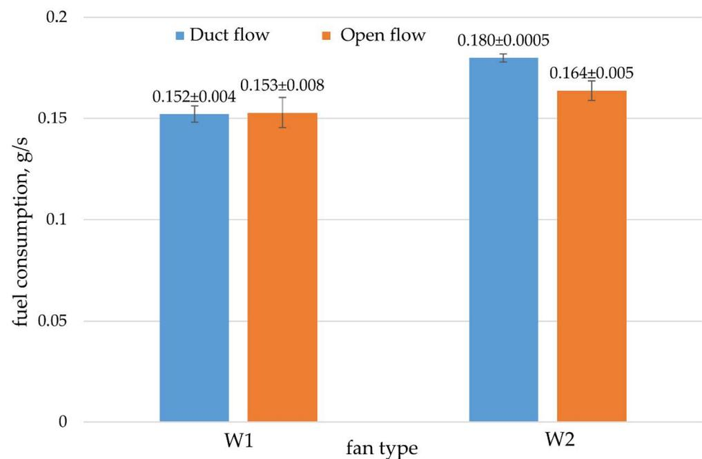
**Figure 7.** Mean fuel consumption during tests with Methods A (duct flow) and B (open flow), where W1—fan with conventional impeller, W2—fan with turbo impeller. All mean values were determined at a 95% confidence interval ( $p = 0.05$ ).
