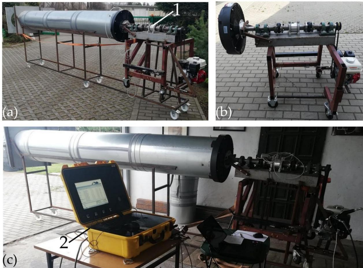
**Figure 1.** Test stand during measurement of the emissions of harmful exhaust gases and energy consumption: (a) measurement during duct flow test (Method A); (b) measurement during open flow test (Method B); (c) PEMS measuring apparatus, where 1—torque meter, 2—PEMS.
