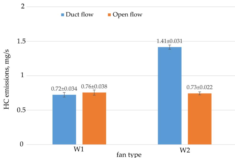
**Figure 10.** Mean HC emissions during tests with Methods A (duct flow) and B (open flow), where W1—fan with conventional impeller, W2—fan with turbo impeller. All mean values were determined at a 95% confidence interval ( $p = 0.05$ ).
