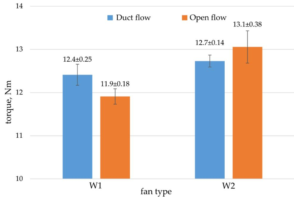
**Figure 5.** Mean torque during tests with Methods A (duct flow) and B (open flow), where W1—fan with conventional impeller, W2—fan with turbo impeller. All mean values were determined at a 95% confidence interval ( $p = 0.05$ ).
