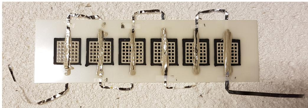
**Figure 4.** The stack consists of six pairs of electrodes on a single electrolyte, electrically connected in series.
