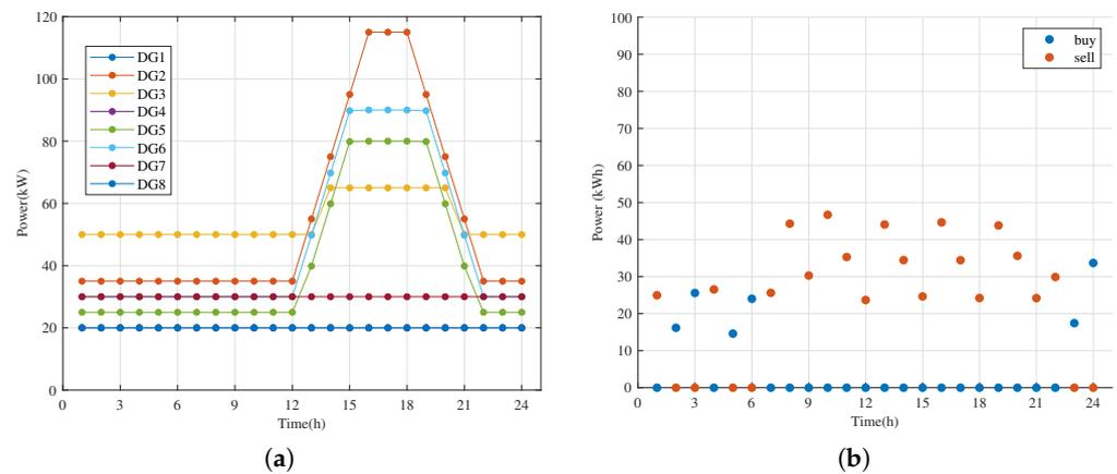
**Figure 8.** The electric power in a VPP: (a) The power of DG; (b) The transaction power with the electrical market.
