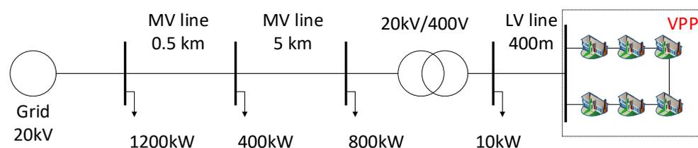
**Figure 1.** The schematic diagram of the VPP.
