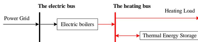
Figure 3. Structure of a regenerative electric heating system.
