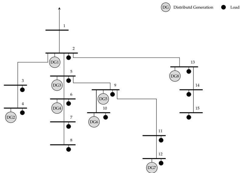
**Figure 4.** The single line diagram of a VPP.
