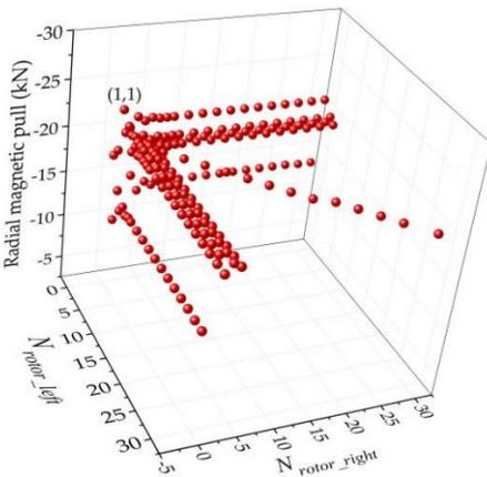
(d) Radial magnetic pull ( $F_{rMR}$ ) (radian of magnetic bond is  $0.5^\circ$ )
