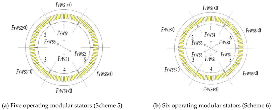
Figure 25. Diagrammatic sketch of combined stators operating in Schemes 5 and 6.
