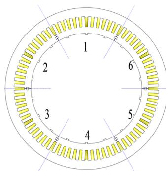
Figure 15. Diagrammatic sketch of the number of modular stators.
