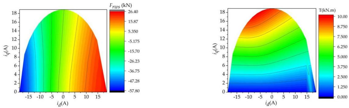
(a) Radial magnetic pull of the whole stator ( $F_{rws}$ )
