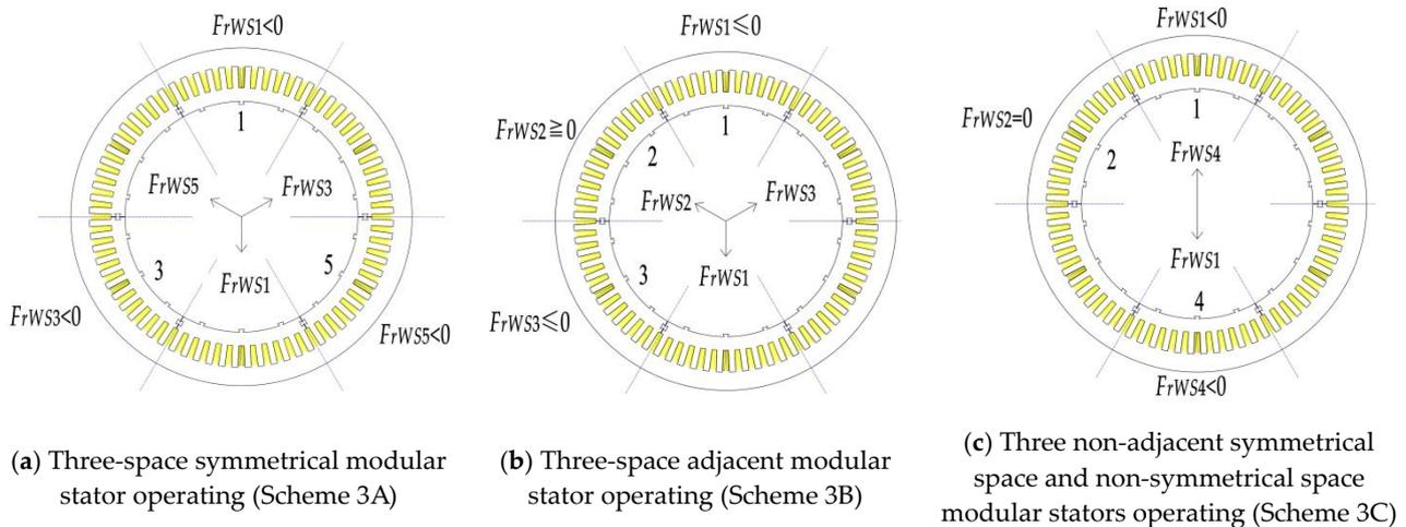
Figure 23. Diagrammatic sketch of combined stators operating in Schemes 3A, 3B and 3C.
