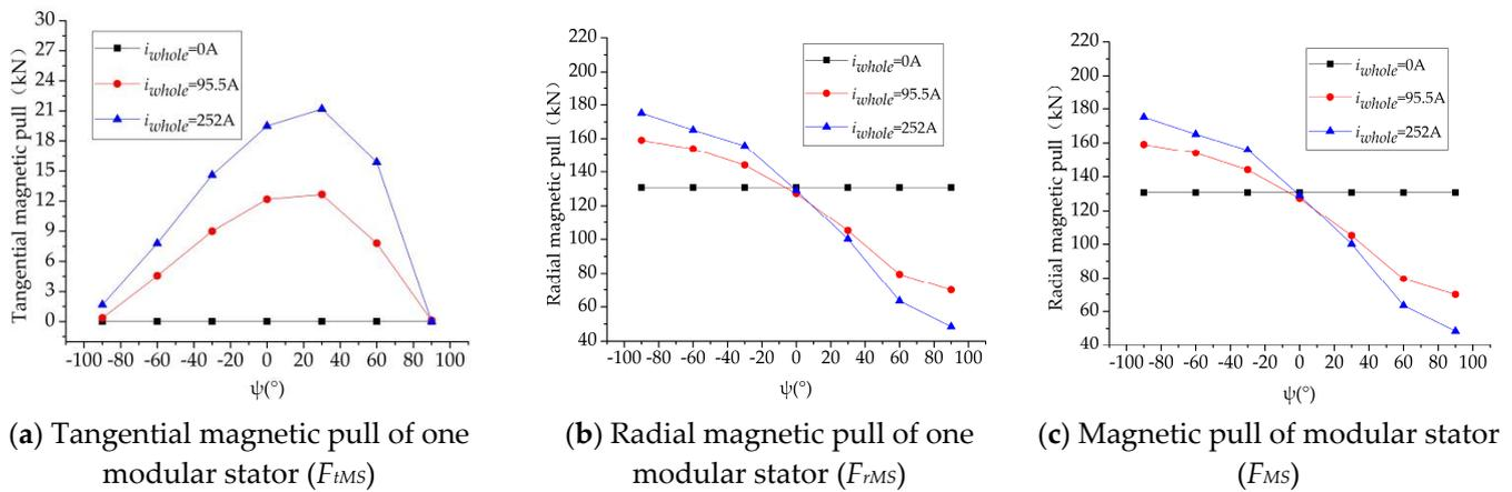
Figure 13. The magnetic pull of the stator with different loads and  $\Psi$ .
