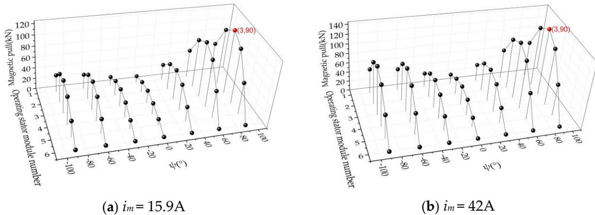
Figure 14. The magnetic pull of the whole stator with different numbers of operating modular stators.
