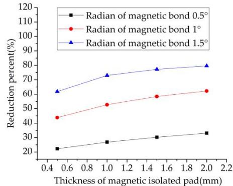
(f) The reduction percent of modular stator magnetic pull
