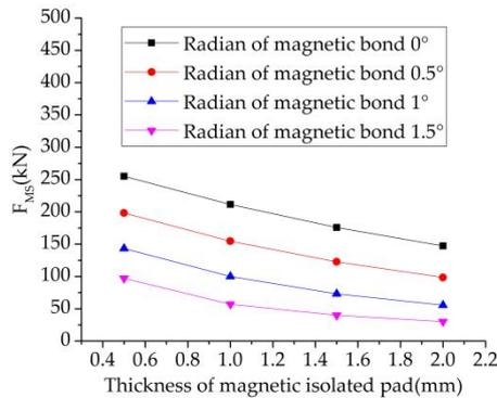
(e) Magnetic pull of modular stator ( $F_{ms}$ )
