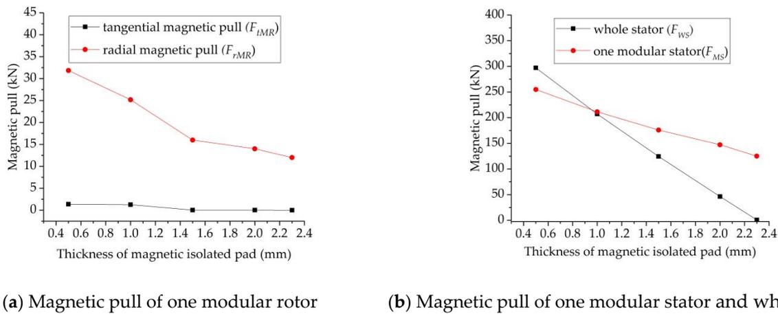
(a) Magnetic pull of one modular rotor (b) Magnetic pull of one modular stator and whole stator
