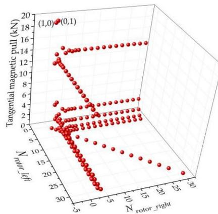
(b) Tangential magnetic pull ( $F_{tMR}$ ) (radian of magnetic bond is  $1^\circ$ )
