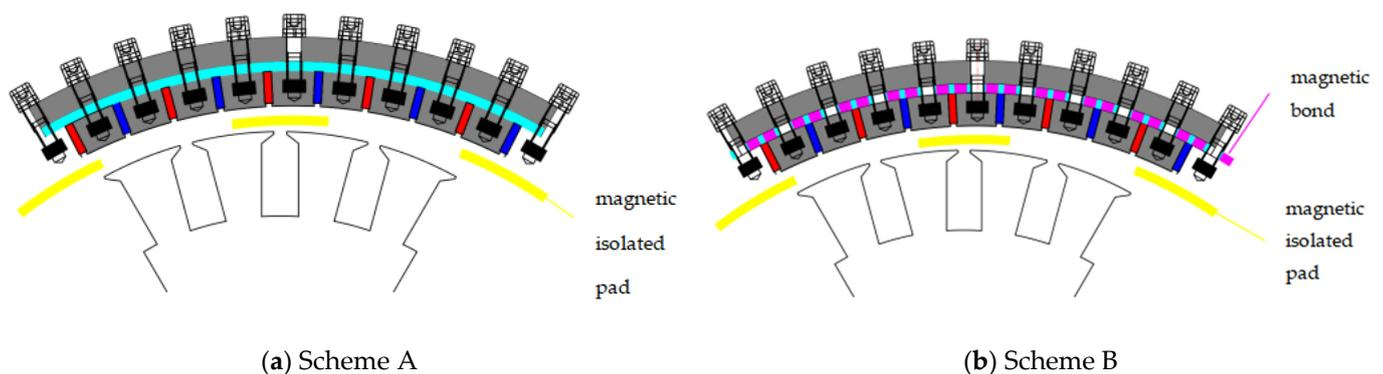
**Figure 3.** Schematic diagram of the motor assembly scheme.
