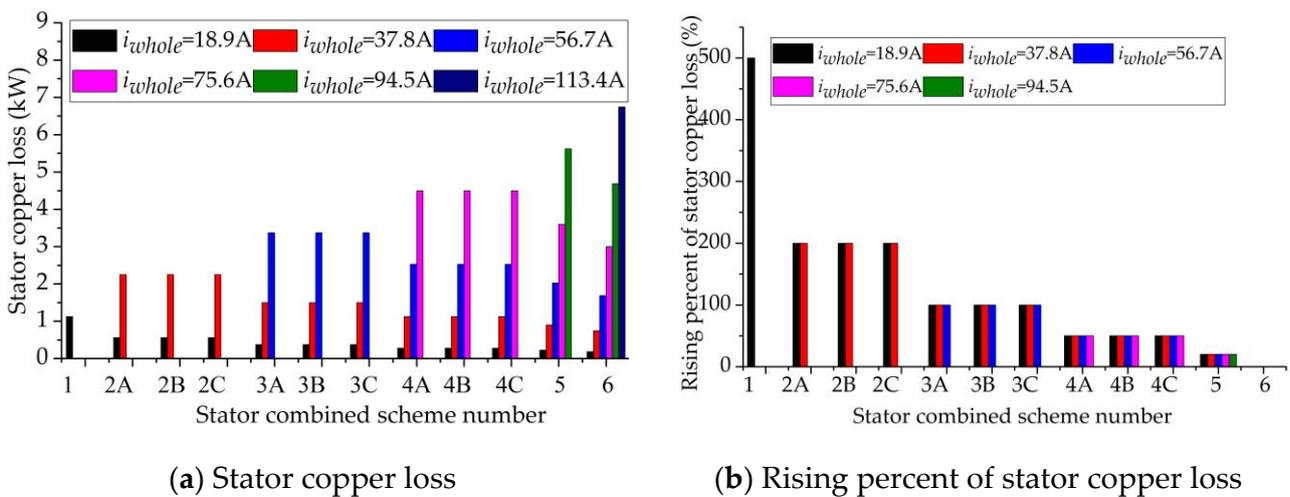
Figure 28. Comparison diagram of the copper loss with different load currents and different operating modular stator combinations.
