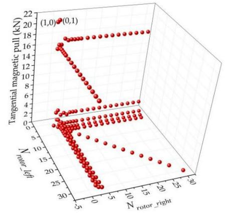
(c) Tangential magnetic pull ( $F_{tMR}$ ) (radian of magnetic bond is  $1.5^\circ$ )
