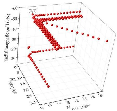
(f) Radial magnetic pull ( $F_{rMR}$ ) (radian of magnetic bond is  $1.5^\circ$ )
