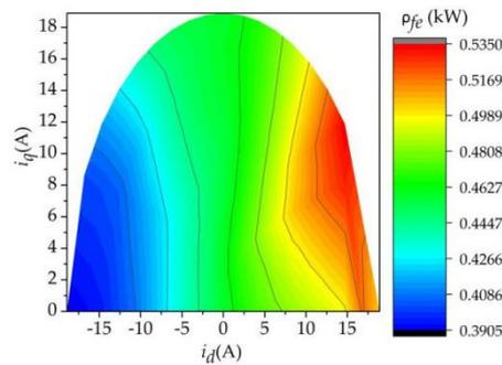
**Figure 17.** The stator iron loss ( $\rho_{fe}$ ) with different  $i_d$  and  $i_q$ .
