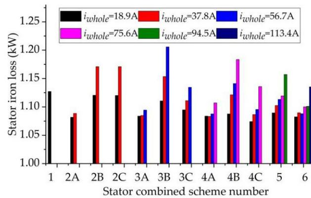
Figure 27. Comparison diagram of the iron loss with different load currents and different operating modular stator combinations.
