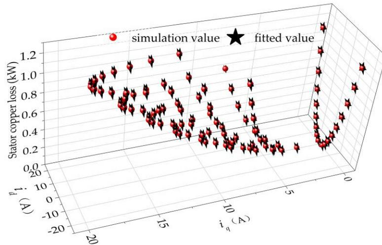
**Figure 20.** The stator copper loss ( $\rho_{cu}$ ) under different  $i_d$  and  $i_q$  with one stator module operating.
