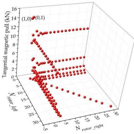
(a) Tangential magnetic pull ( $F_{tMR}$ ) (radian of magnetic bond is  $0.5^\circ$ )
