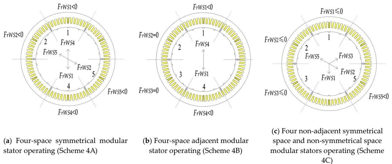
Figure 24. Diagrammatic sketch of combined stators operating in Schemes 4A, 4B, and 4C.
