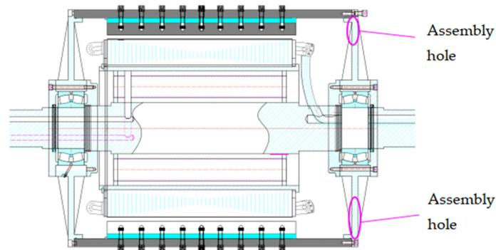
**Figure 4.** Schematic diagram of the assembly hole location.
