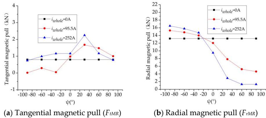
Figure 12. The magnetic pull of one modular rotor with different load currents and  $\Psi$ .
