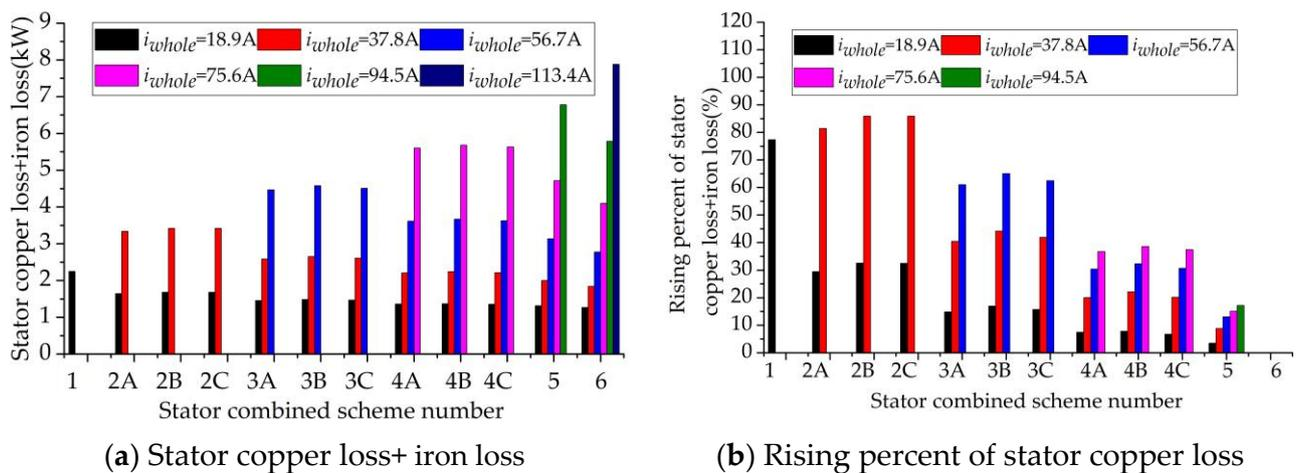
**Figure 29.** Comparison diagram of the stator copper and iron loss with different load currents and different operating modular stator combinations.
