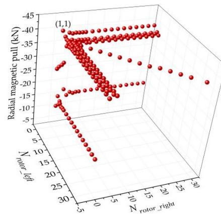
(e) Radial magnetic pull ( $F_{rMR}$ ) (radian of magnetic bond is  $1^\circ$ )
