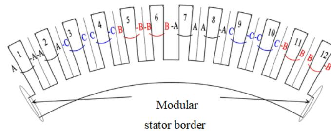
**Figure 2.** Coil layout of one modular stator.
