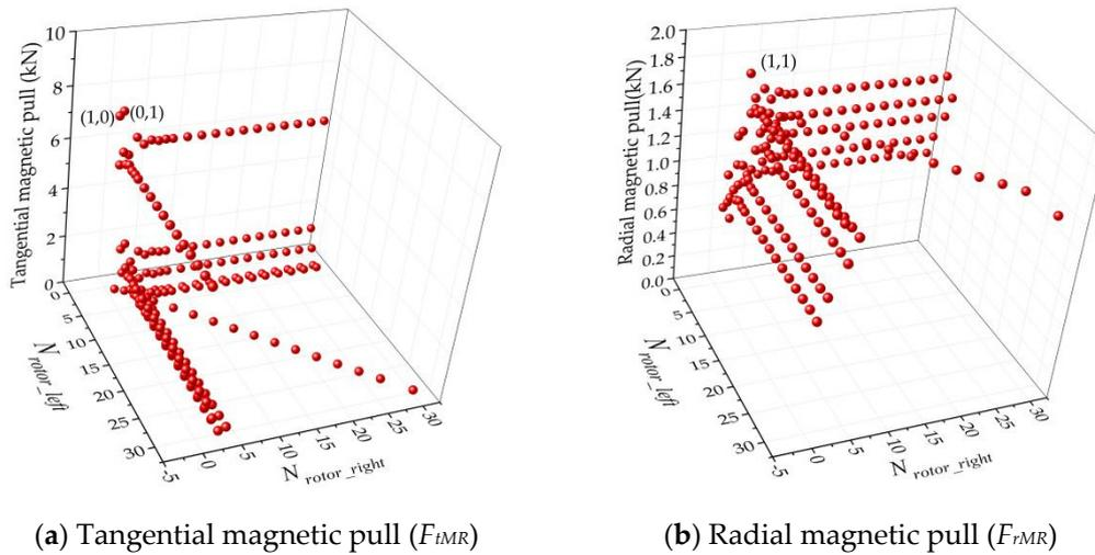
Figure 8. Magnetic pull of one modular rotor core in the Scheme A, Step A1 process.
