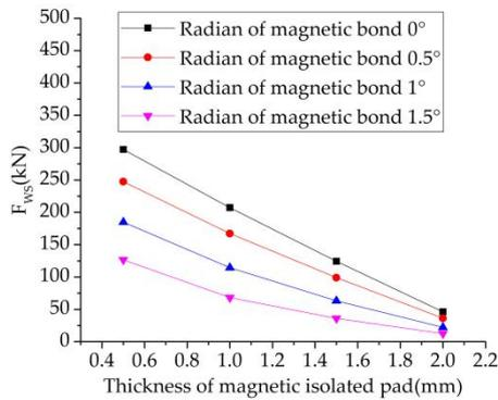
(c) Magnetic pull of whole stator ( $F_{ws}$ )
