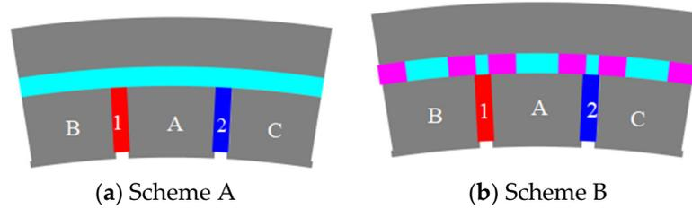
**Figure 6.** The local enlarged rotor schematic of rotor core A (with inserted magnets via magnet grooves 1 and 2).
