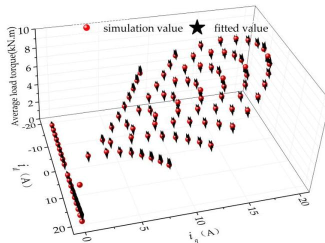
Figure 19. The load torque ( $T$ ) under different  $i_d$  and  $i_q$  with one stator module operating.
