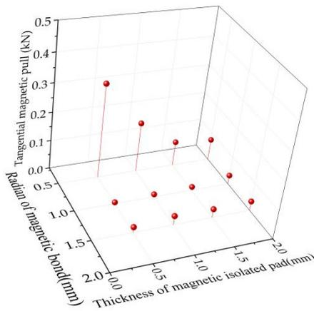
(a) Tangential magnetic pull of modular rotor ( $F_{tMR}$ )
