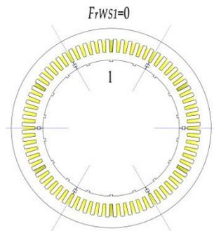
**Figure 21.** Diagrammatic sketch of the combined stator in Scheme 1: the single operating modular stator.
