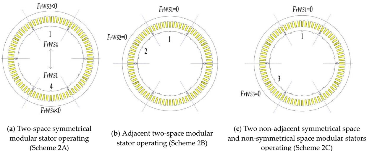
**Figure 22.** Diagrammatic sketch of combined stators operating in Schemes 2A, 2B, and 2C.
