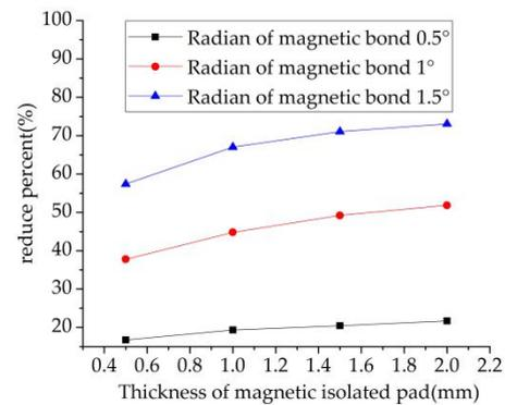
(d) The reduction percent of whole stator magnetic pull
