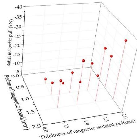
(b) Radial magnetic pull of modular rotor ( $F_{rMR}$ )
