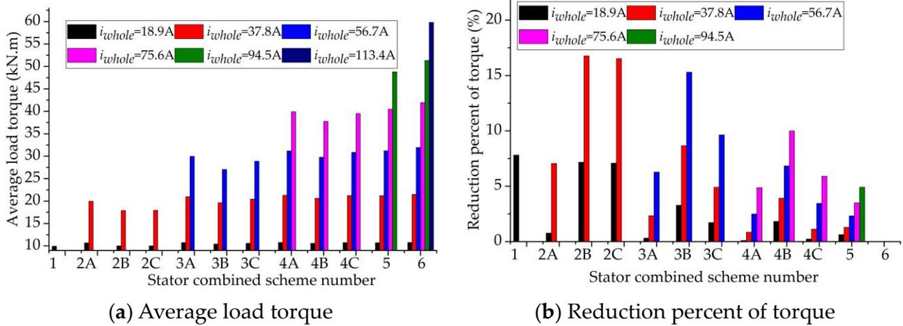
Figure 26. Comparison diagram of load torque with different load currents and different operating modular stator combinations.
