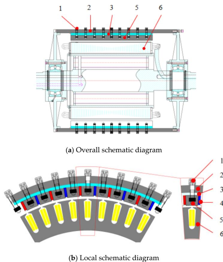
**Figure 1.** Diagram for the outer rotor of the MSTPMM. 1. Non-magnetic bolt; 2. outer rotor yoke; 3. non-magnetic stainless steel; 4. permanent magnet; 5. modular rotor core; and 6. modular stator core.
