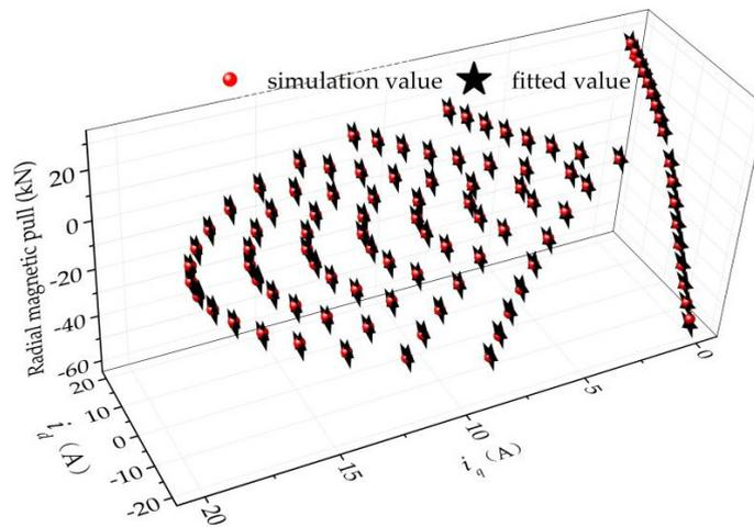
Figure 18. Radial magnetic pull of the whole stator ( $F_{rWS}$ ) under different  $i_d$  and  $i_q$  with one stator module operating.
