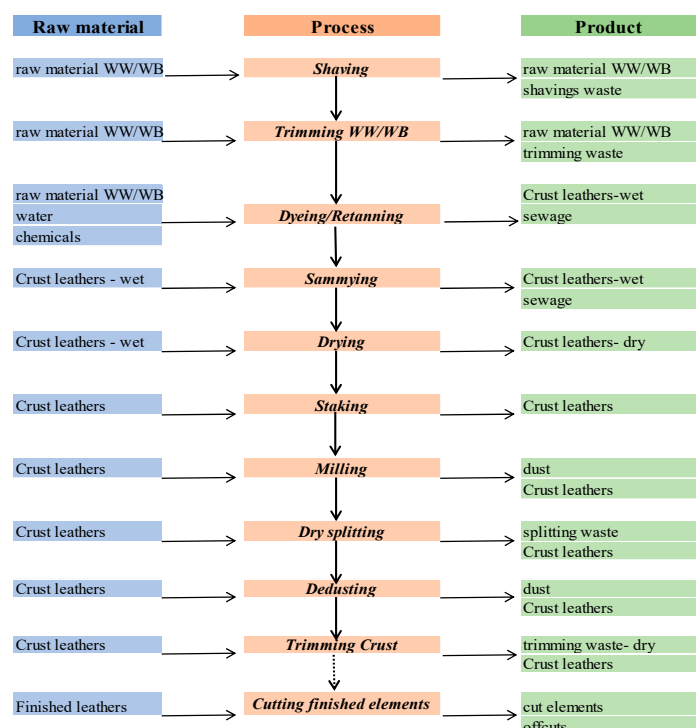
Figure 1. An exemplary technological diagram of leather processing.
